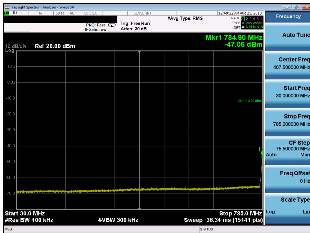
Plot 7-25. Conducted Spurious Plot (LTE Band 14, 5 MHz QPSK – RB Size 1, RB Offset 0 – Low Channel)
