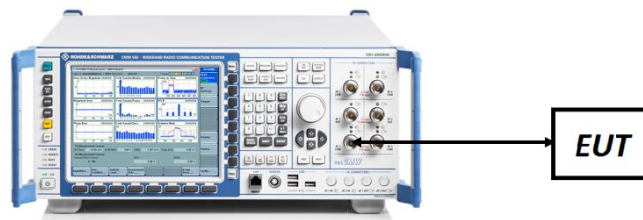
Figure 7-4. Conducted Power Measurement Setup
