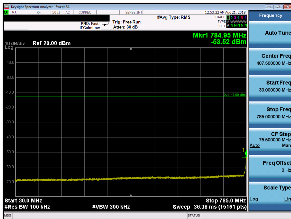
Plot 7-31. Conducted Spurious Plot (LTE Band 14, 5 MHz QPSK – RB Size 1, RB Offset 0 – High Channel)
