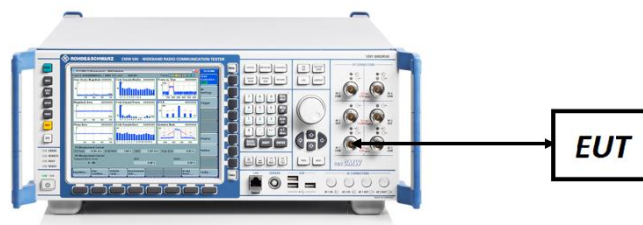
Figure 7-5. ERP/EIRP Measurement Setup
