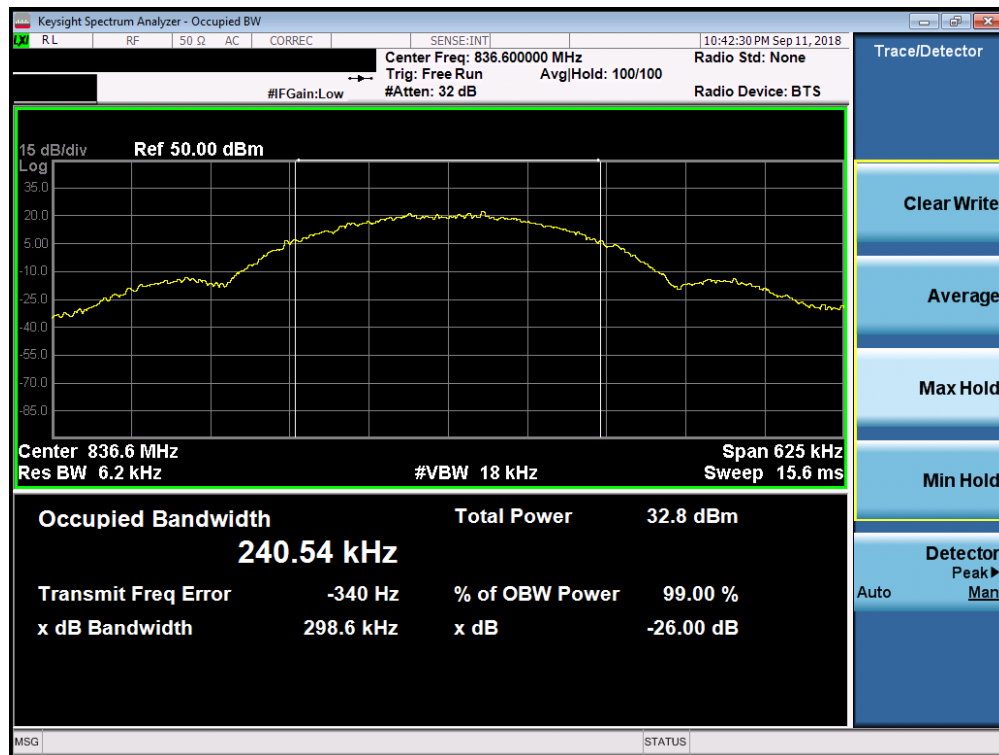
Plot 7-2. Occupied Bandwidth Plot (EDGE850Mode)
