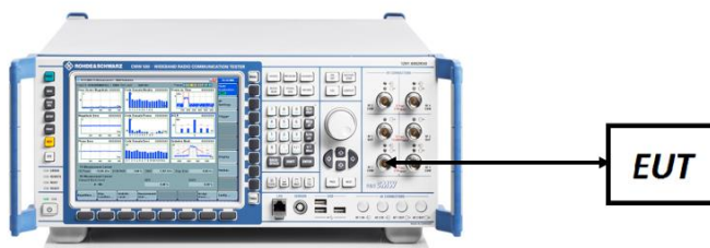
Figure 7-5. ERP/EIRP Measurement Setup
