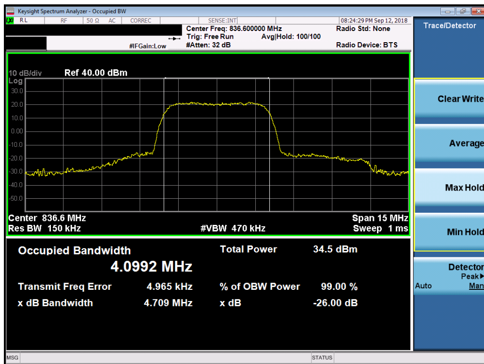
Plot 7-5. Occupied Bandwidth Plot (Cellular WCDMA Mode)
