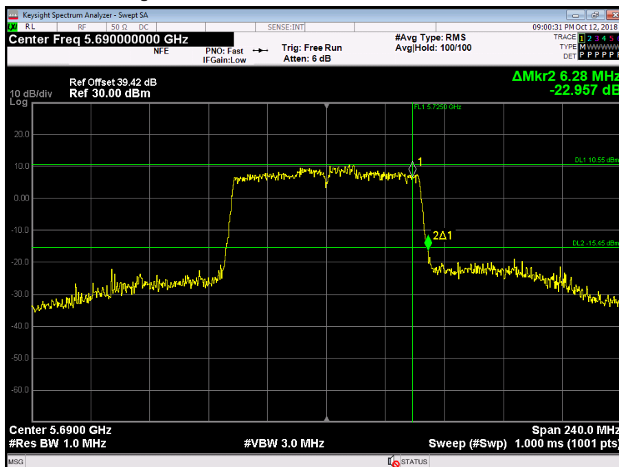
Figure 374 - 5690 MHz - 26 dB Emission Bandwidth
