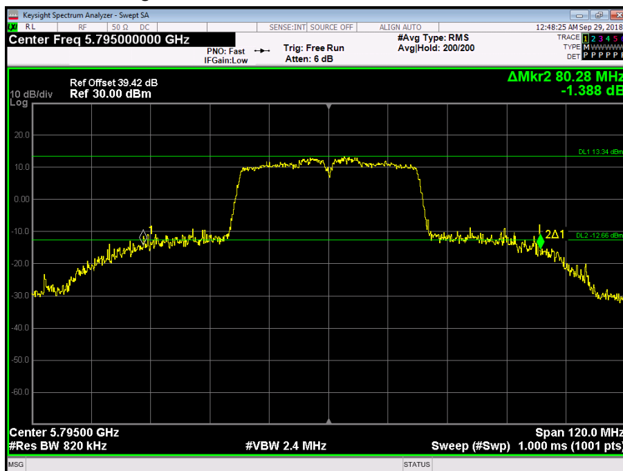
Figure 353 - 5795 MHz - 26 dB Emission Bandwidth
