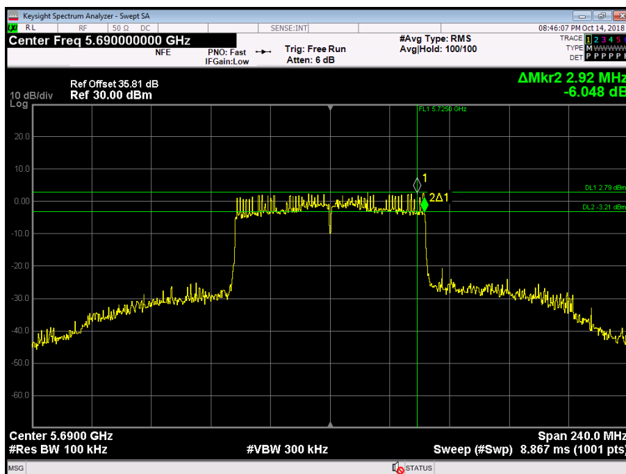
Figure 367 - 5690 MHz - 6 dB DTS Bandwidth
