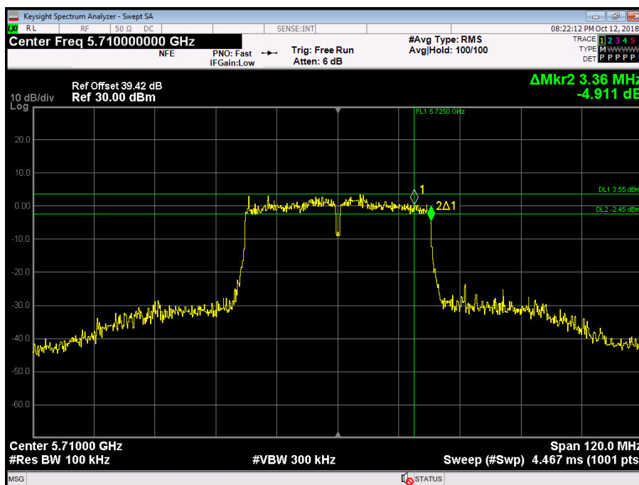
Figure 346 - 5710 MHz - 6 dB DTS Bandwidth
