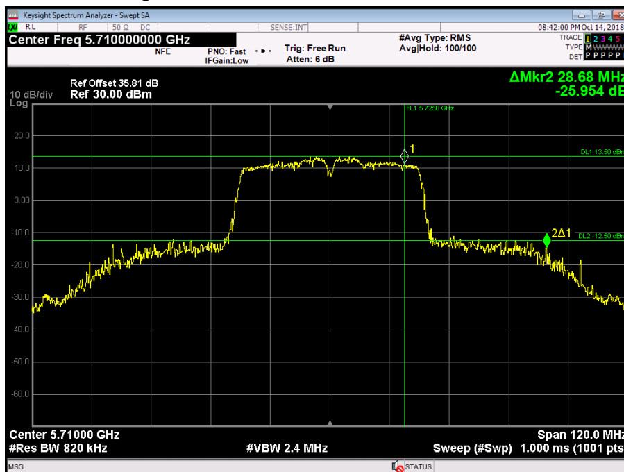
Figure 326 - 5710 MHz - 26 dB Emission Bandwidth
