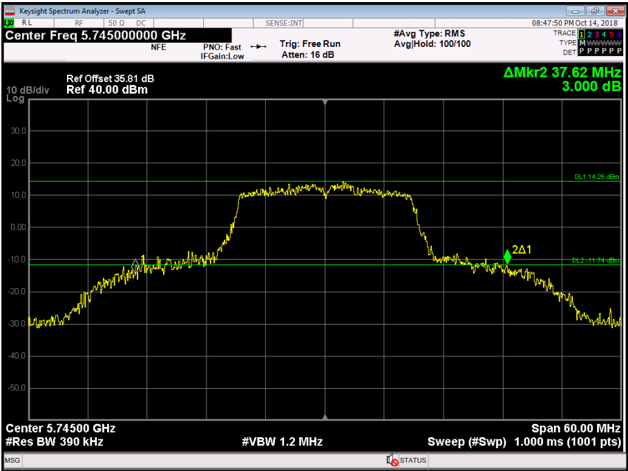
Figure 287 - 5745 MHz - 26 dB Emission Bandwidth
