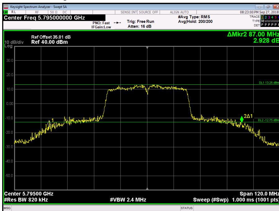
Figure 314 - 5795 MHz - 26 dB Emission Bandwidth
