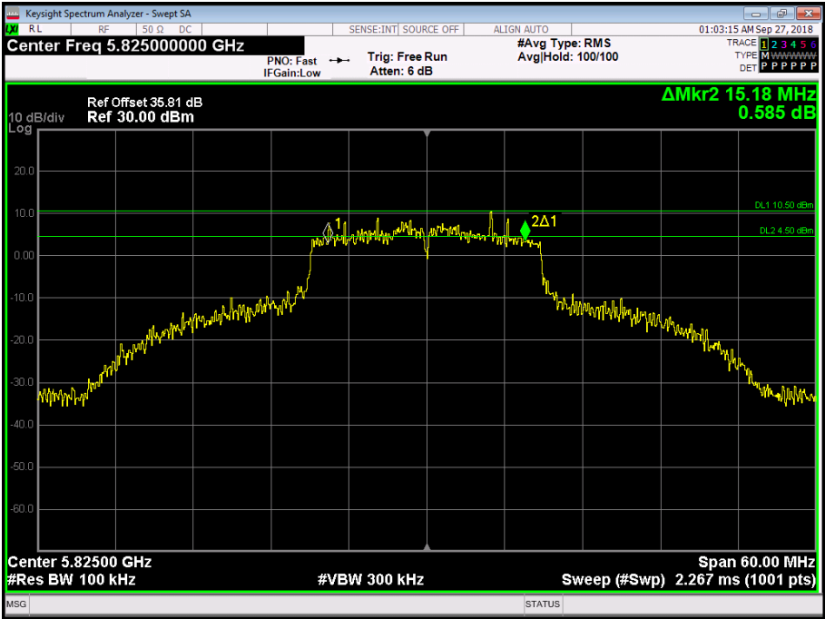
Figure 304 - 5825 MHz - 6 dB DTS Bandwidth
