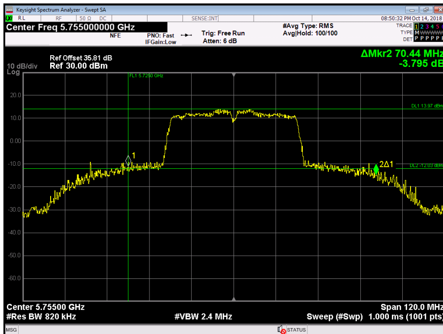
Figure 320 - 5755 MHz - 26 dB Emission Bandwidth
