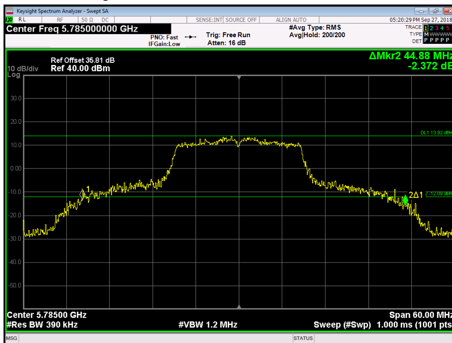
Figure 278 - 5785 MHz - 26 dB Emission Bandwidth
