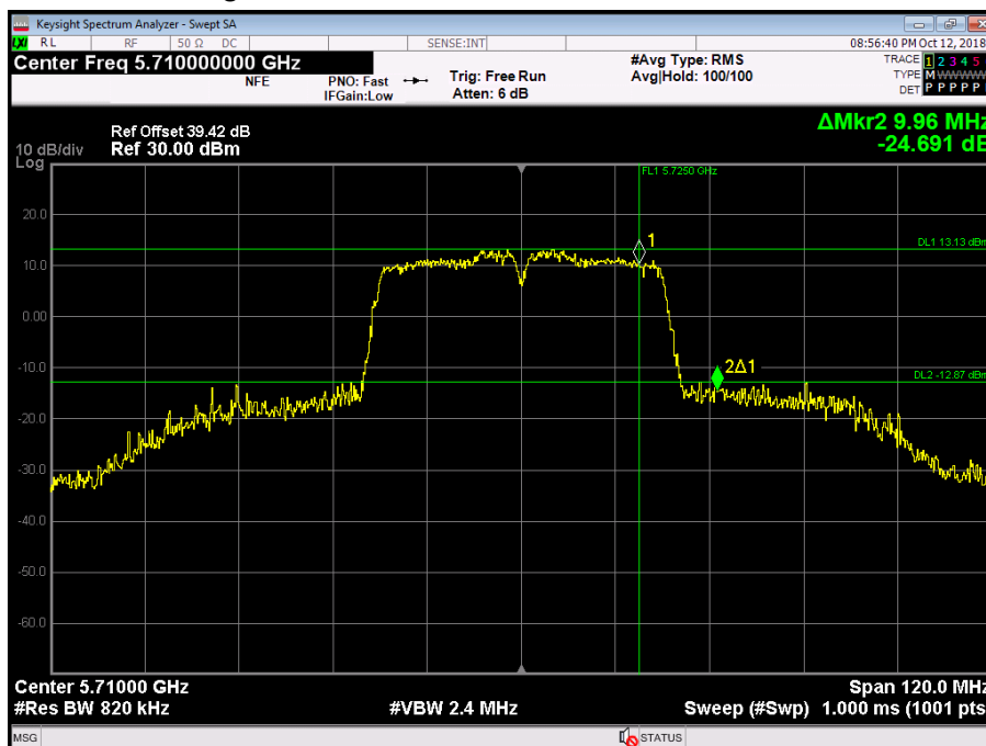
Figure 347 - 5710 MHz - 26 dB Emission Bandwidth
