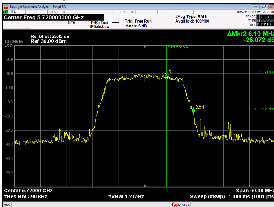
Figure 335 - 5720 MHz - 26 dB Emission Bandwidth
