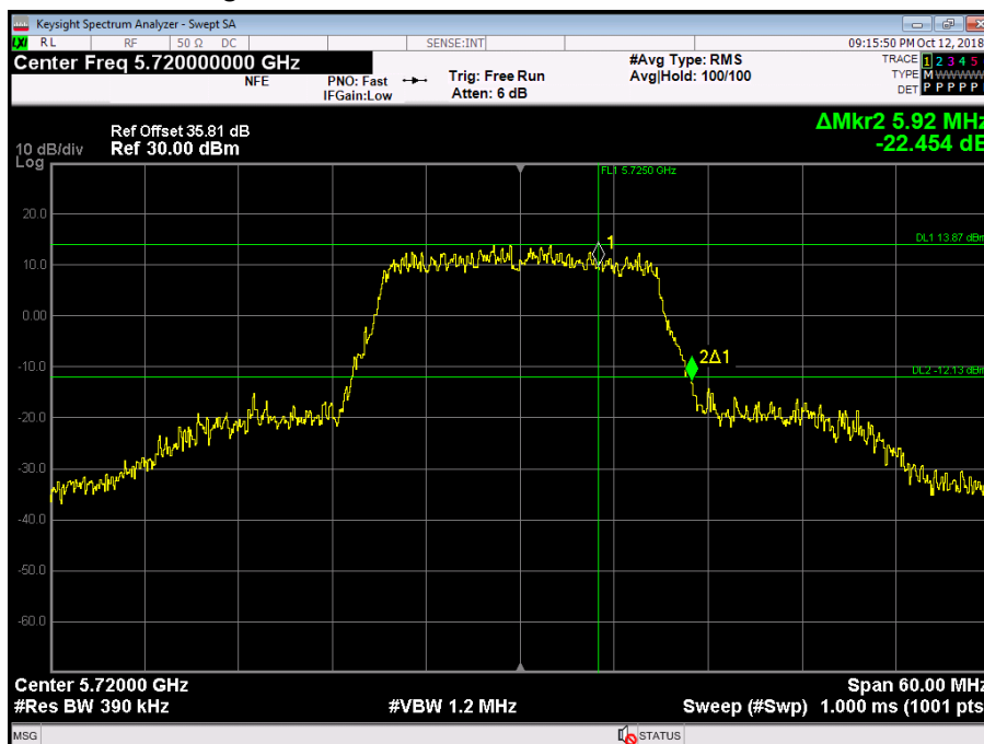
Figure 272 - 5720 MHz - 26 dB Emission Bandwidth
