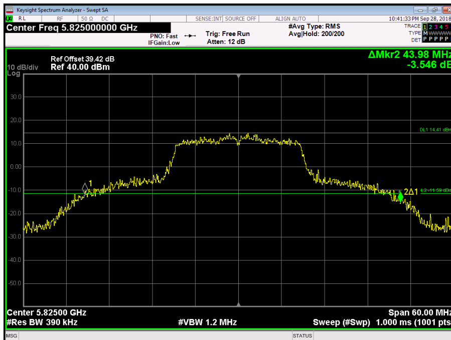
Figure 344 - 5825 MHz - 26 dB Emission Bandwidth
