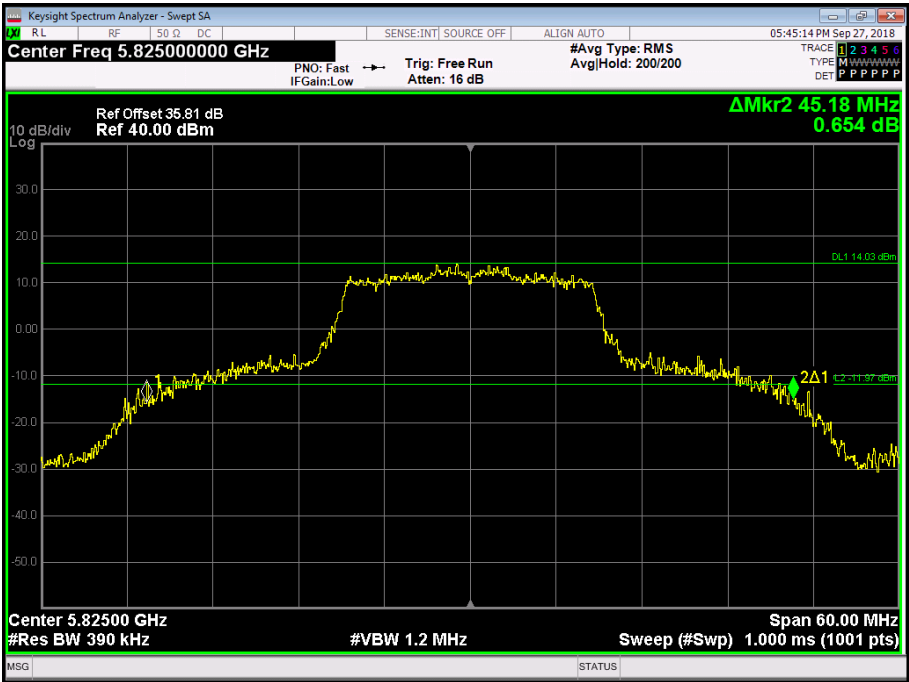
Figure 281 - 5825 MHz - 26 dB Emission Bandwidth
