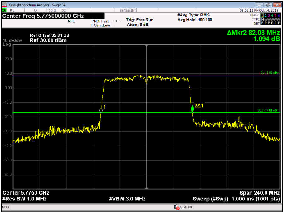
Figure 365 - 5775 MHz - 26 dB Emission Bandwidth
