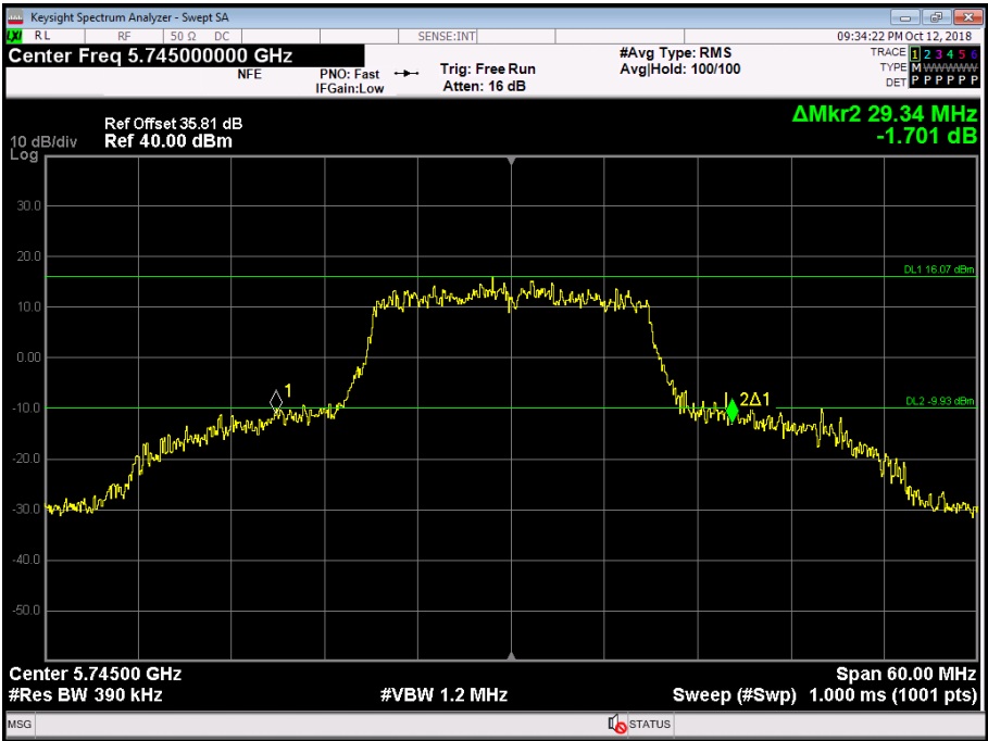
Figure 275 - 5745 MHz - 26 dB Emission Bandwidth
