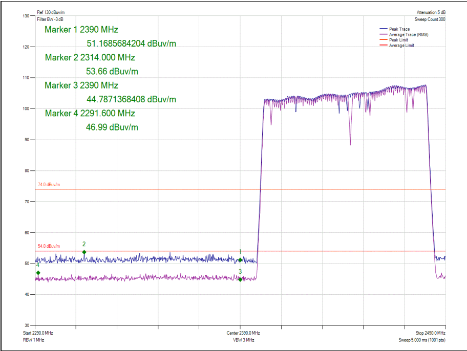
Figure 46 - Hopping - GFSK/DH5 - Measured Frequency 2390.0 MHz
