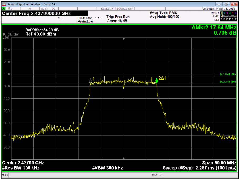
Figure 63 - 2437 MHz - 6 dB DTS Bandwidth
