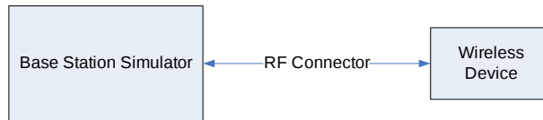
Figure 8-2 Power Measurement Setup
