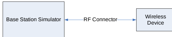
Figure 8-1 Power Measurement Setup
