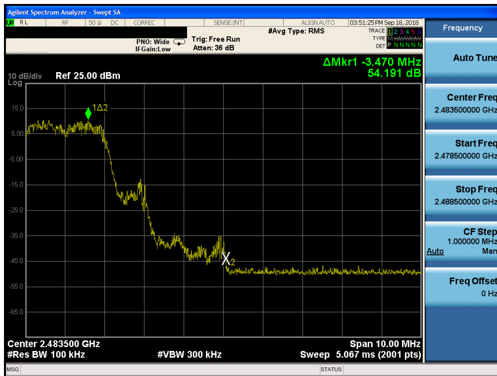
Plot 7-34. Band Edge Plot ANT1 (Bluetooth with Hopping Enabled, 8DPSK, ePA – Ch. 78)
