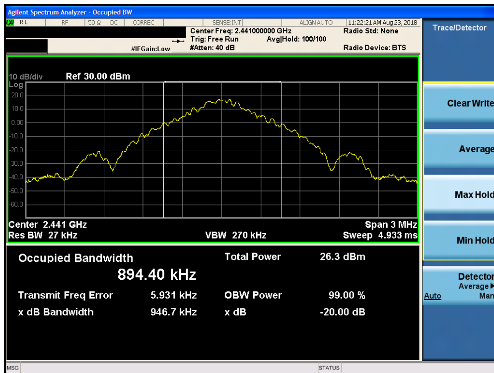
Plot 7-2. 20dB Bandwidth Plot ANT0 (Bluetooth, GFSK, ePA – Ch. 39)
