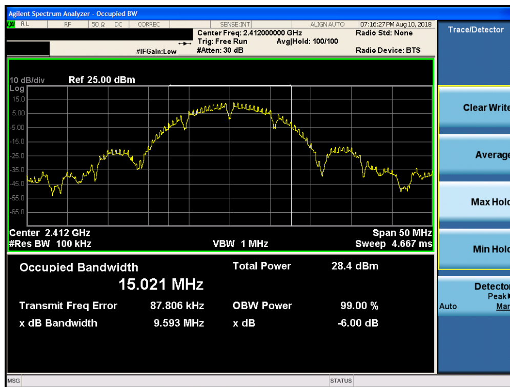
Plot 7-19. 6dB Bandwidth Plot SISO CORE1 DIVERSITY (802.11b – Ch. 1)
