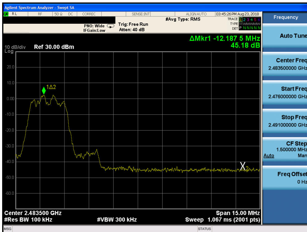
Plot 7-60. Band Edge Plot ANT1 (Bluetooth (HDR4, ePA), 4Mbps – Ch. 75)
