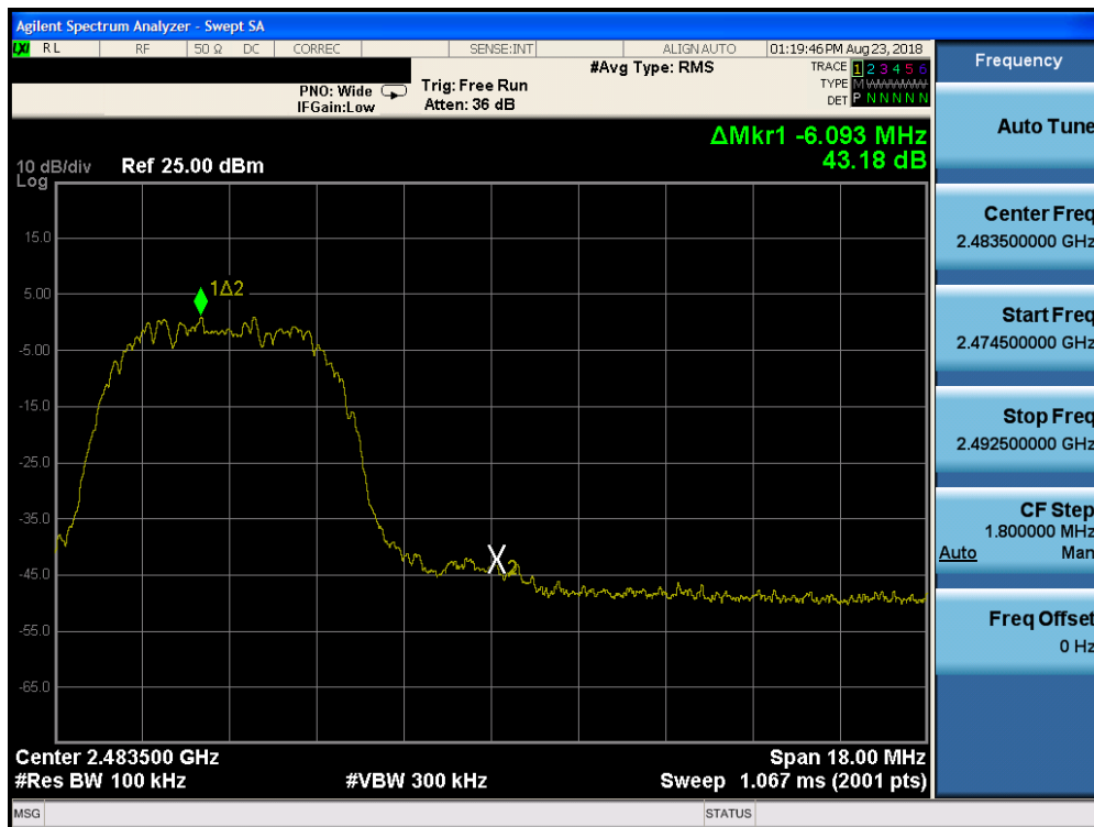
Plot 7-58. Band Edge Plot ANT0 (Bluetooth (HDR8, ePA), 8Mbps - Ch. 75)
