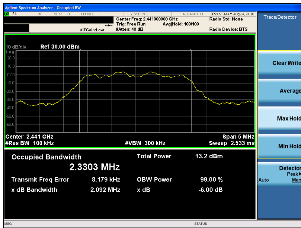
Plot 7-14. 6dB Bandwidth Plot ANT2 (Bluetooth (HDR4, ePA), 4Mbps – Ch. 38)
