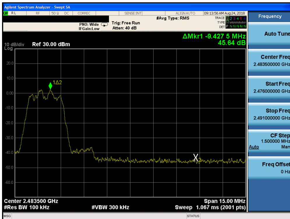
Plot 7-64. Band Edge Plot ANT2 (Bluetooth (HDR4, ePA), 4Mbps – Ch. 75)
