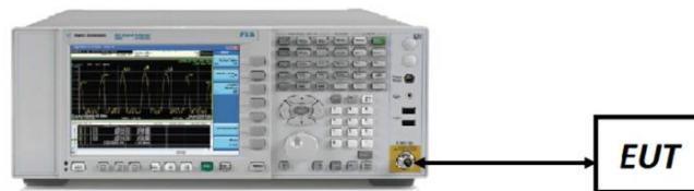
Figure 7-5. Test Instrument & Measurement Setup
