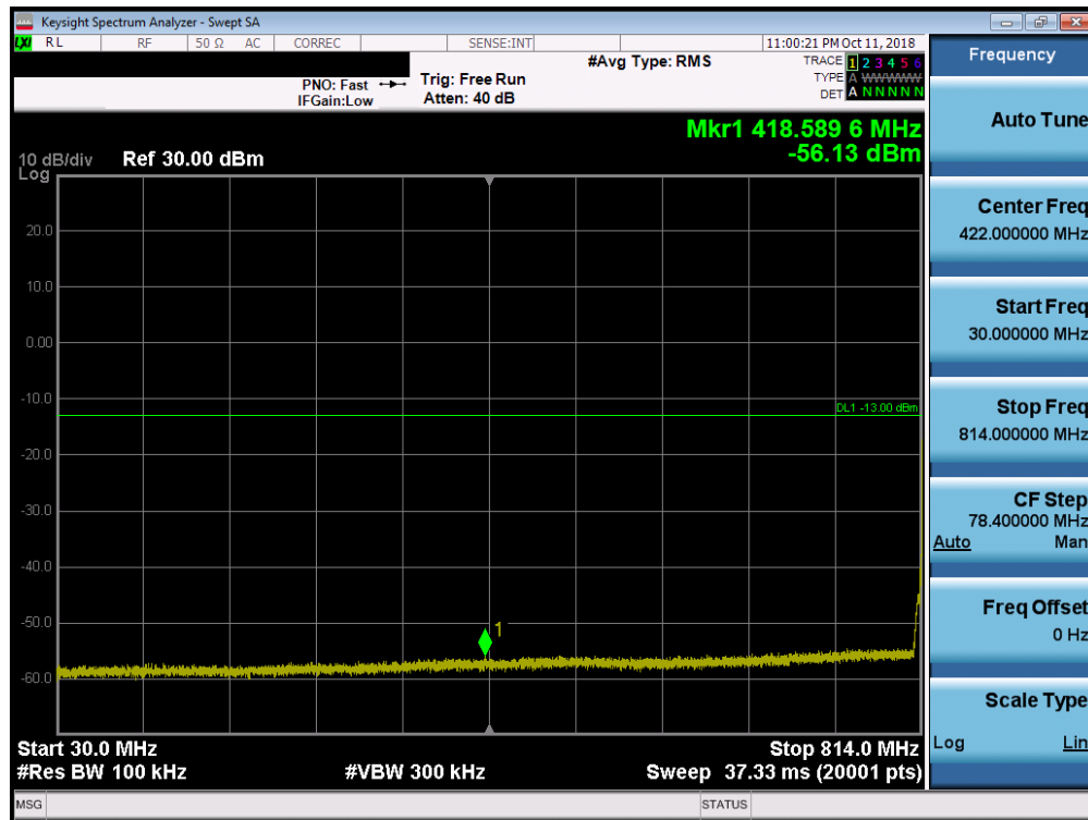
Plot 7-19. Conducted Spurious Plot (LTE Band 26, 5 MHz QPSK – RB Size 1, RB Offset 0 – Low Channel)
