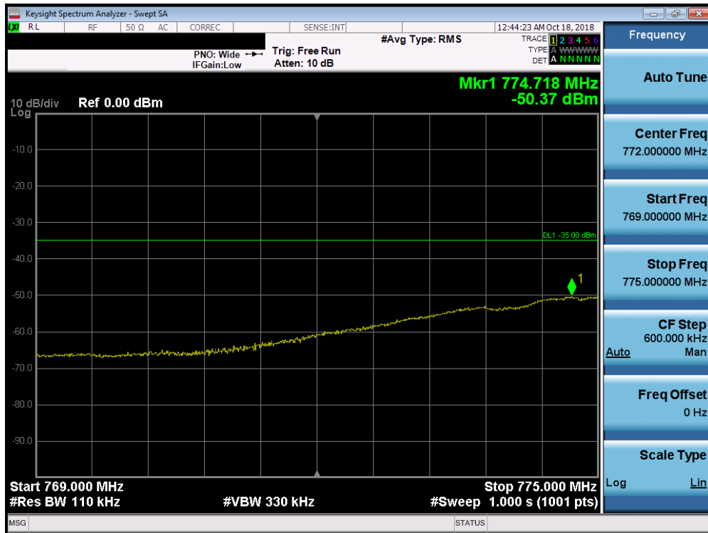
Plot 7-46. Lower Emission Mask Plot (LTE Band 14, 10MHz QPSK – RB Size 50)
