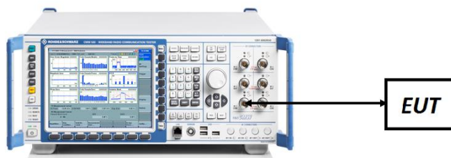
Figure 7-5. ERP/EIRP Measurement Setup
