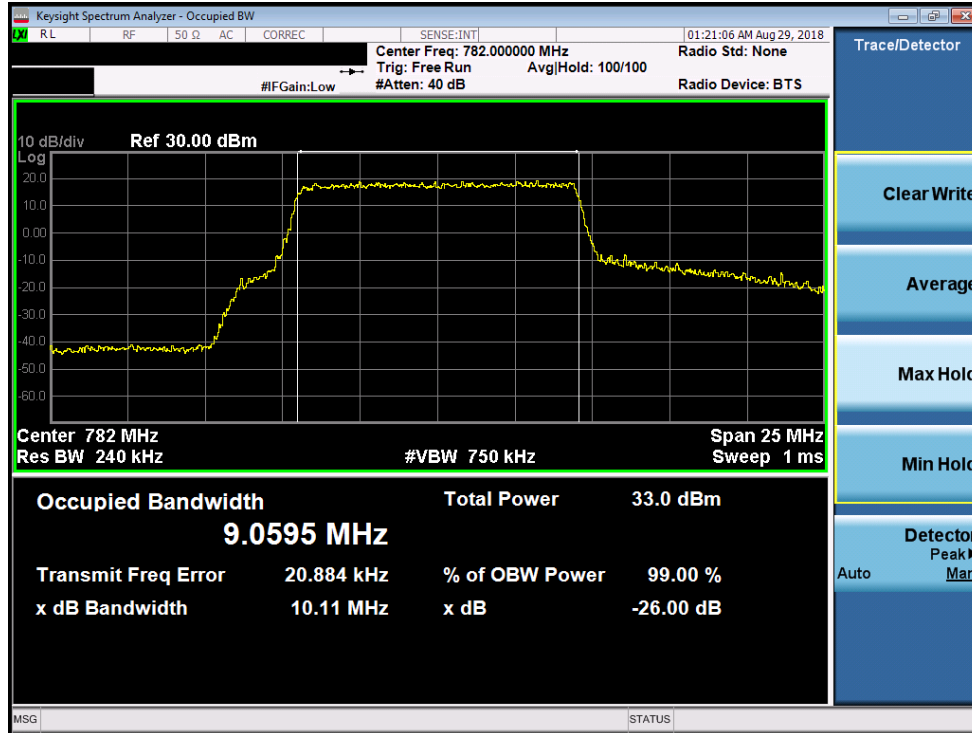
Plot 7-17. Occupied Bandwidth Plot (Band 13 – 10.0MHz 16-QAM – RB Size 50)
