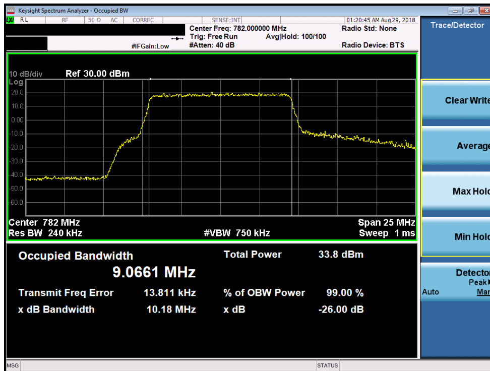
Plot 7-16. Occupied Bandwidth Plot (Band 13 – 10.0MHz QPSK – RB Size 50)
