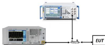
Figure 7-2. Test Instrument & Measurement Setup
