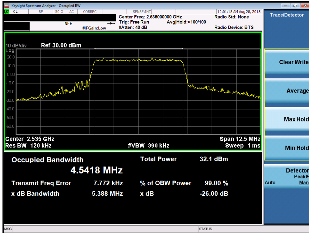
Plot 7-75. Occupied Bandwidth Plot (Band 7 – 5.0MHz 64-QAM – RB Size 25)
