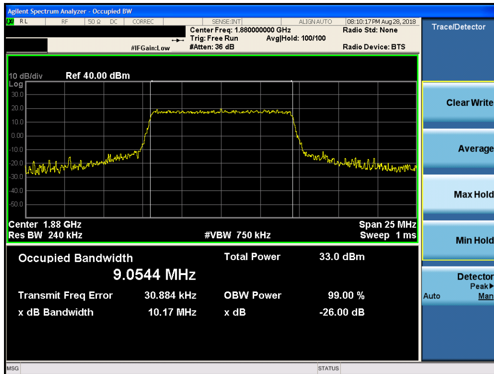
Plot 7-58. Occupied Bandwidth Plot (Band 25/2 – 10.0MHz QPSK – RB Size 50)
