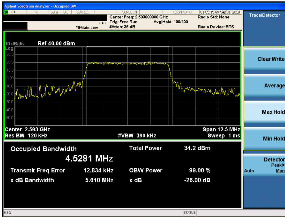
Plot 7-85. Occupied Bandwidth Plot (Band 41 – 5.0MHz QPSK – RB Size 25)
