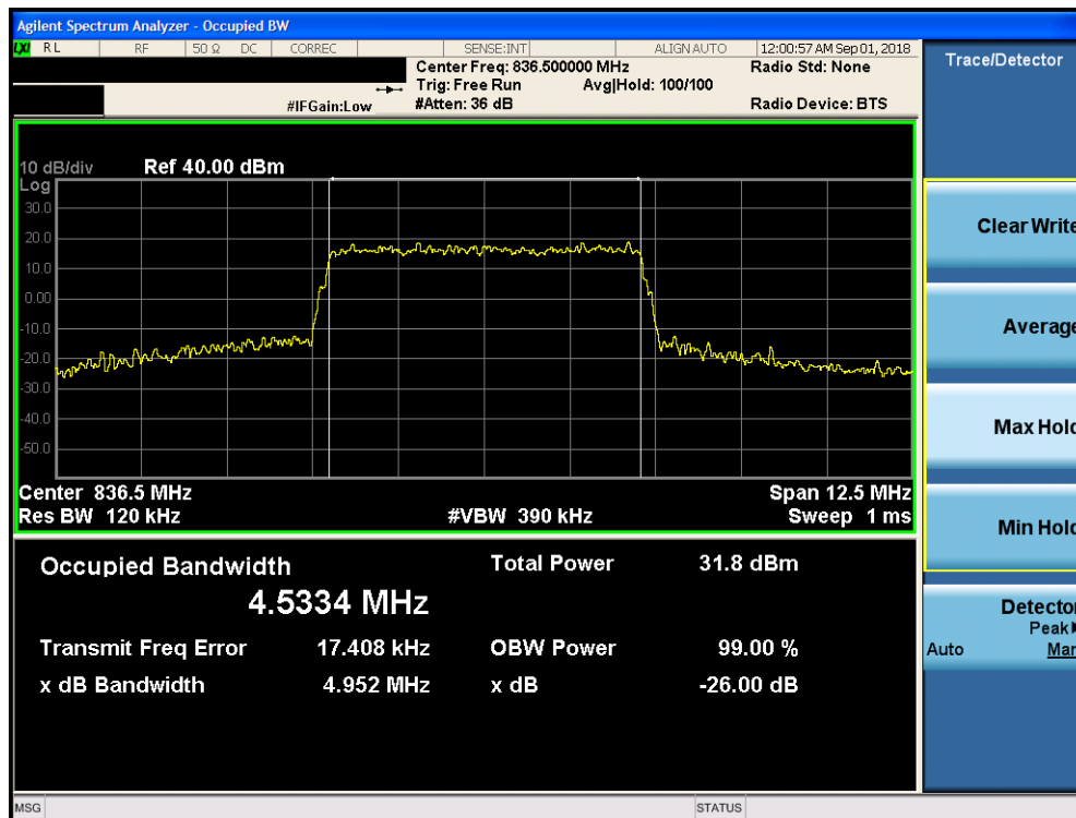
Plot 7-26. Occupied Bandwidth Plot (Band 26/5 – 5.0MHz 16-QAM – RB Size 25)
