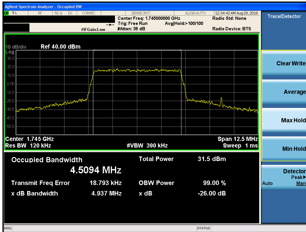
Plot 7-38. Occupied Bandwidth Plot (Band 66/4 – 5.0MHz 16-QAM – RB Size 25)
