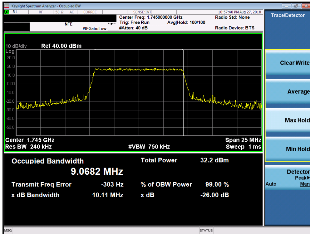
Plot 7-42. Occupied Bandwidth Plot (Band 66/4 – 10.0MHz 64-QAM – RB Size 50)
