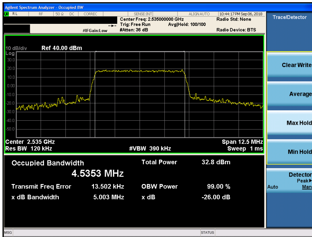
Plot 7-74. Occupied Bandwidth Plot (Band 7 – 5.0MHz 16-QAM – RB Size 25)
