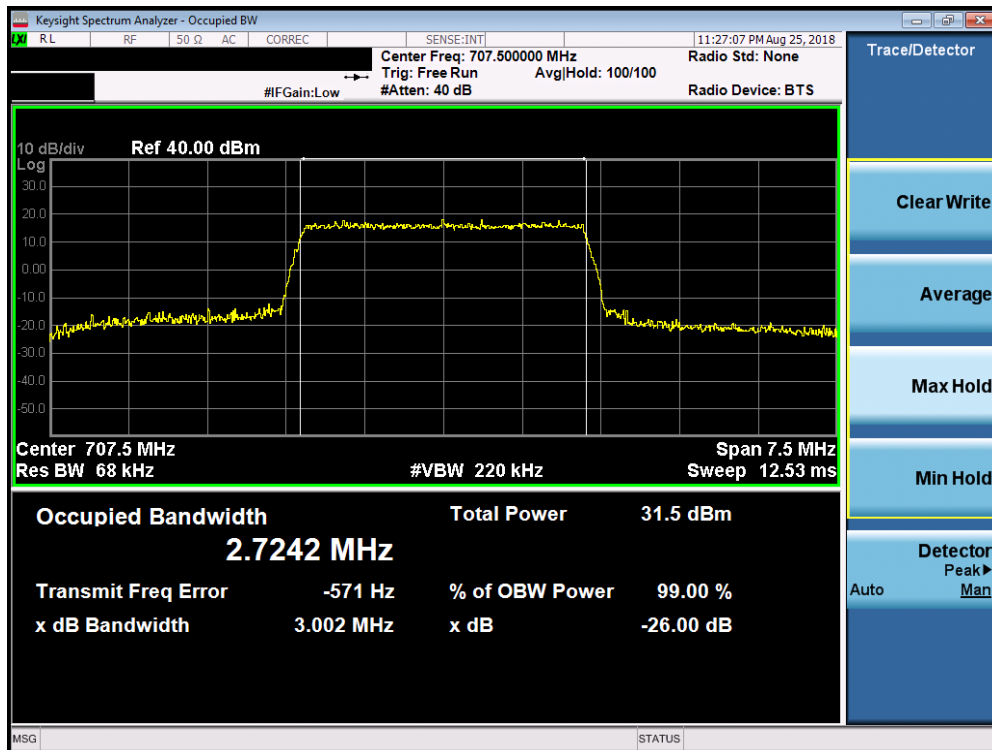
Plot 7-6. Occupied Bandwidth Plot (Band 12 – 3.0MHz 64-QAM – RB Size 15)
