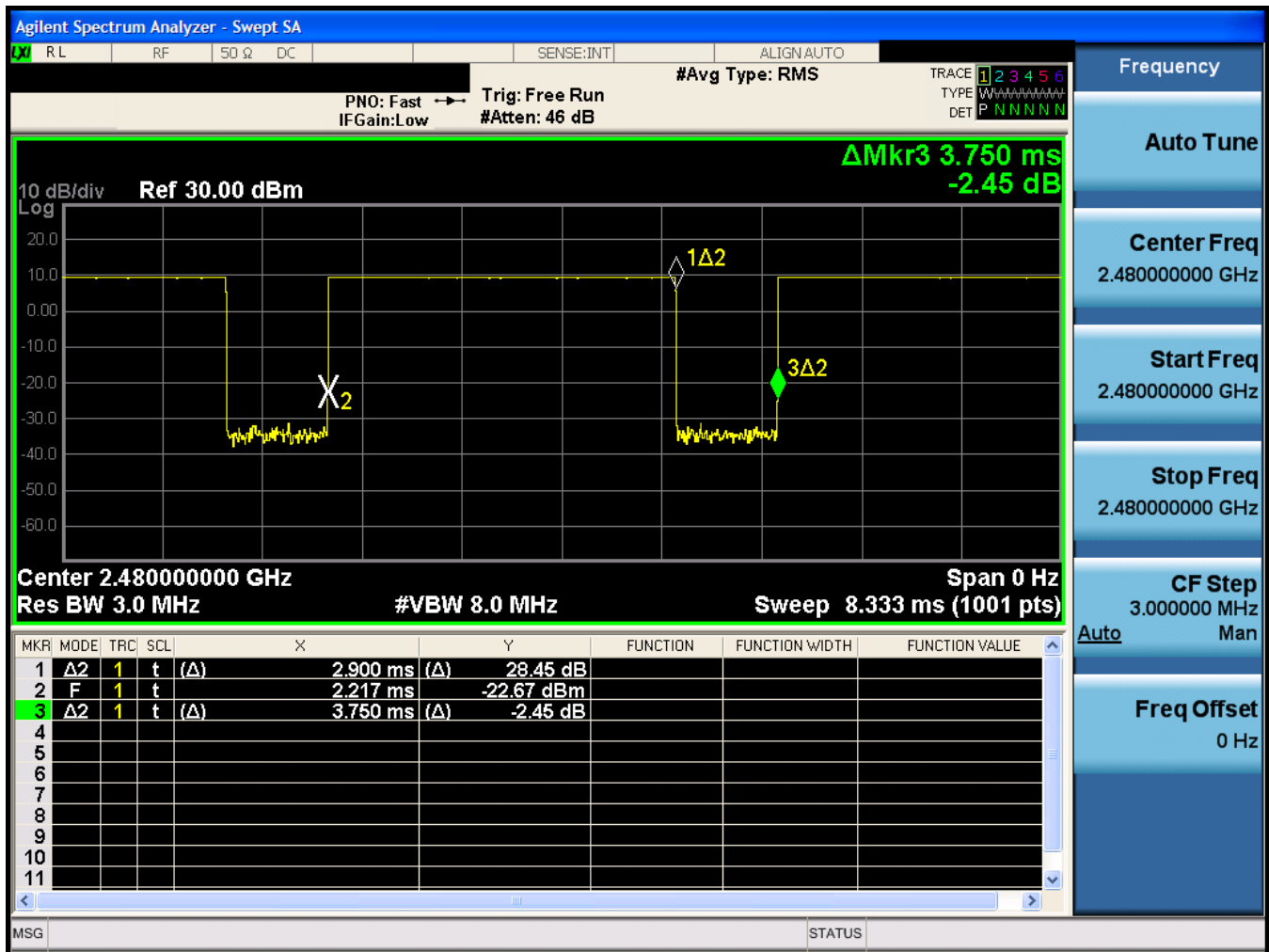
Figure 7-3 Bluetooth P_{Low} Transmission Plot & Duty Cycle Calculation – Variant 1
