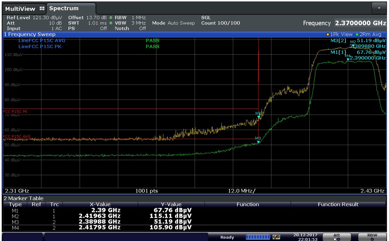
Plot 7-178. Radiated Restricted Upper Band Edge Measurement (Average & Peak)
