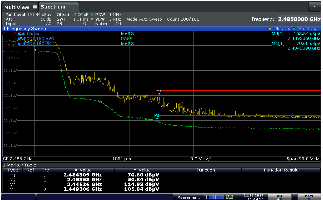
Plot 7-200. Radiated Restricted Upper Band Edge Measurement (Average & Peak)
