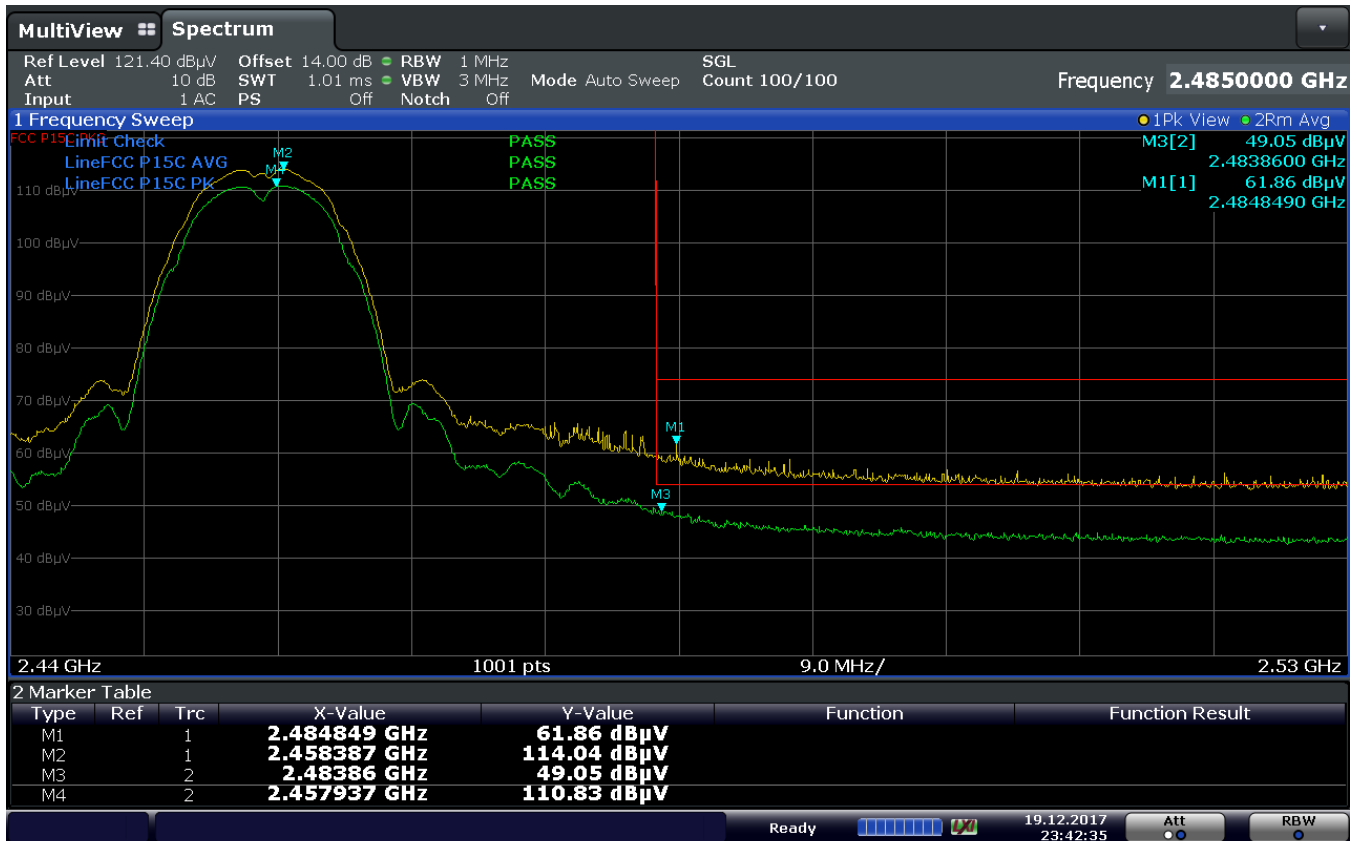
Plot 7-190. Radiated Restricted Upper Band Edge Measurement (Average & Peak)
