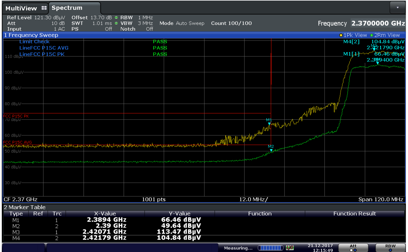
Plot 7-196. Radiated Restricted Lower Band Edge Measurement (Average & Peak)
