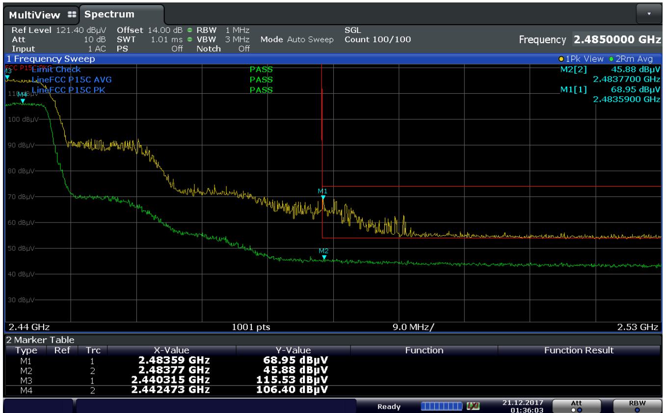
Plot 7-181. Radiated Restricted Upper Band Edge Measurement (Average & Peak)
