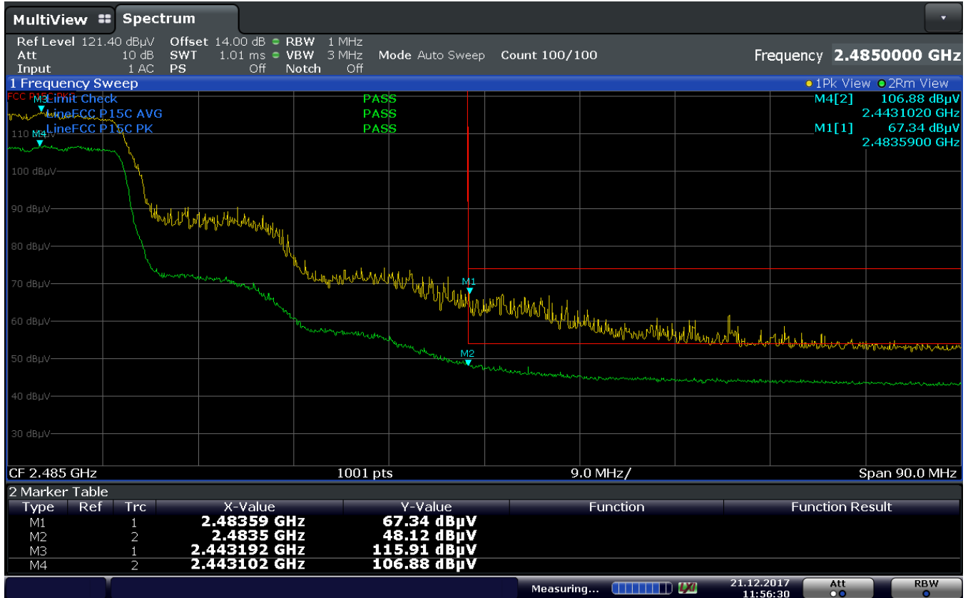
Plot 7-199. Radiated Restricted Upper Band Edge Measurement (Average & Peak)
