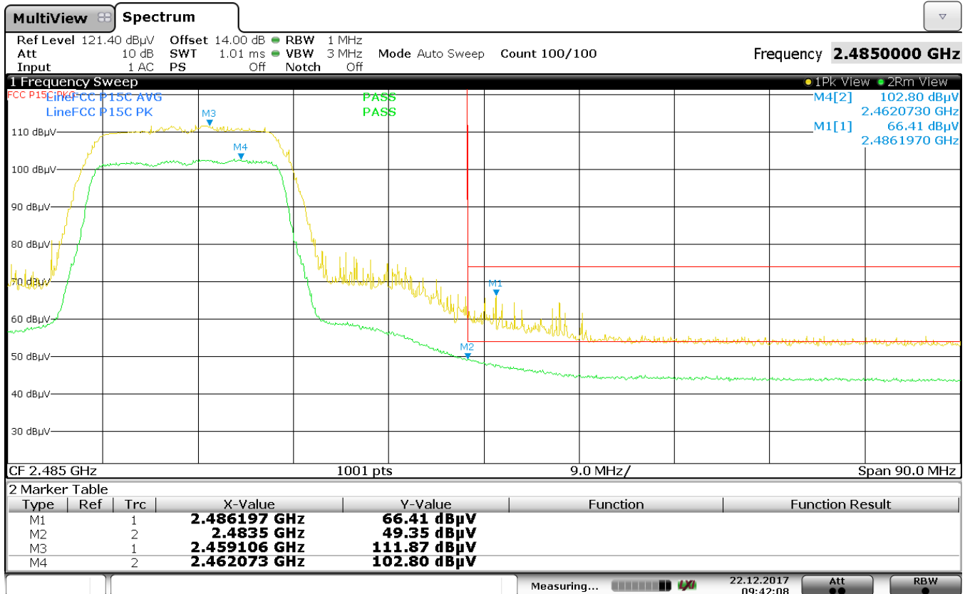
Plot 7-202. Radiated Restricted Upper Band Edge Measurement (Average & Peak)
