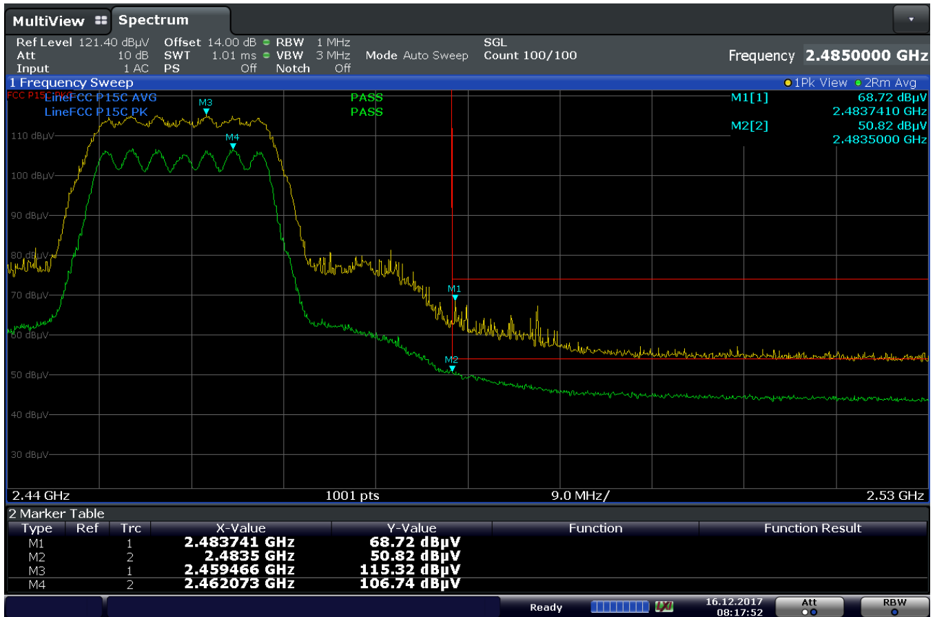
Plot 7-208. Radiated Restricted Upper Band Edge Measurement (Average & Peak)
