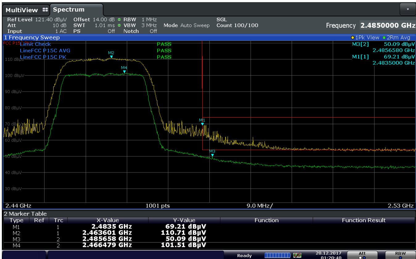
Plot 7-186. Radiated Restricted Upper Band Edge Measurement (Average & Peak)
