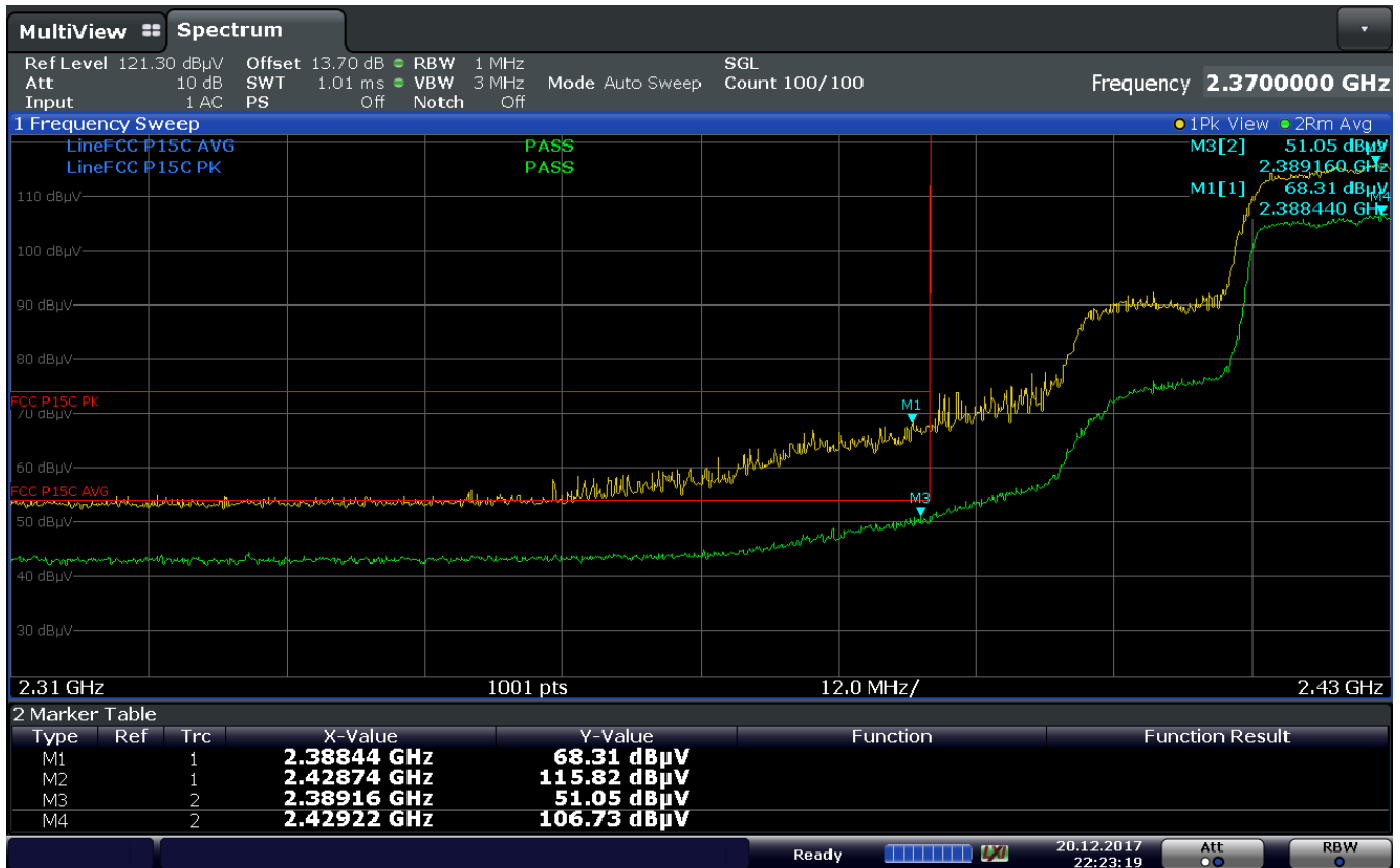
Plot 7-180. Radiated Restricted Upper Band Edge Measurement (Average & Peak)
