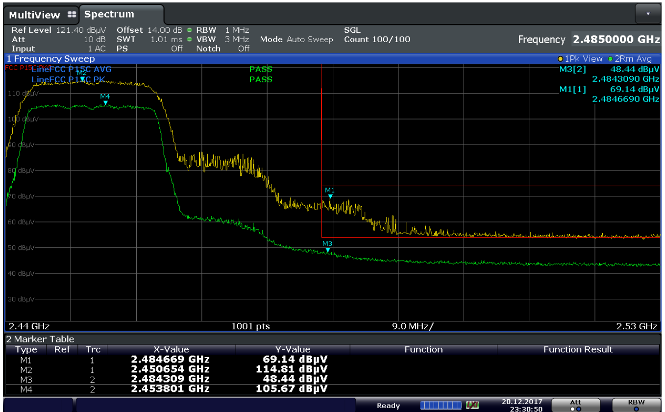
Plot 7-184. Radiated Restricted Upper Band Edge Measurement (Average & Peak)
