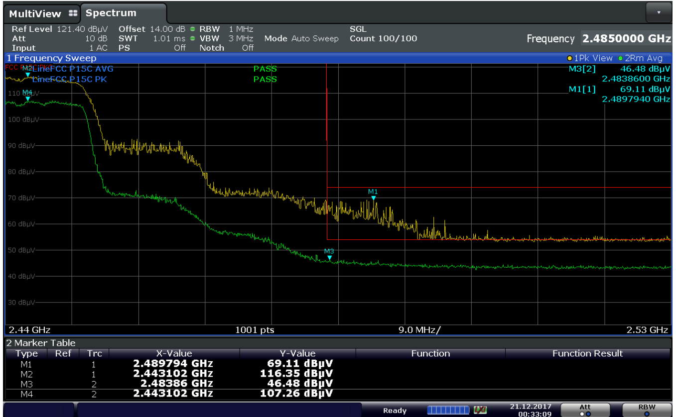
Plot 7-182. Radiated Restricted Upper Band Edge Measurement (Average & Peak)
