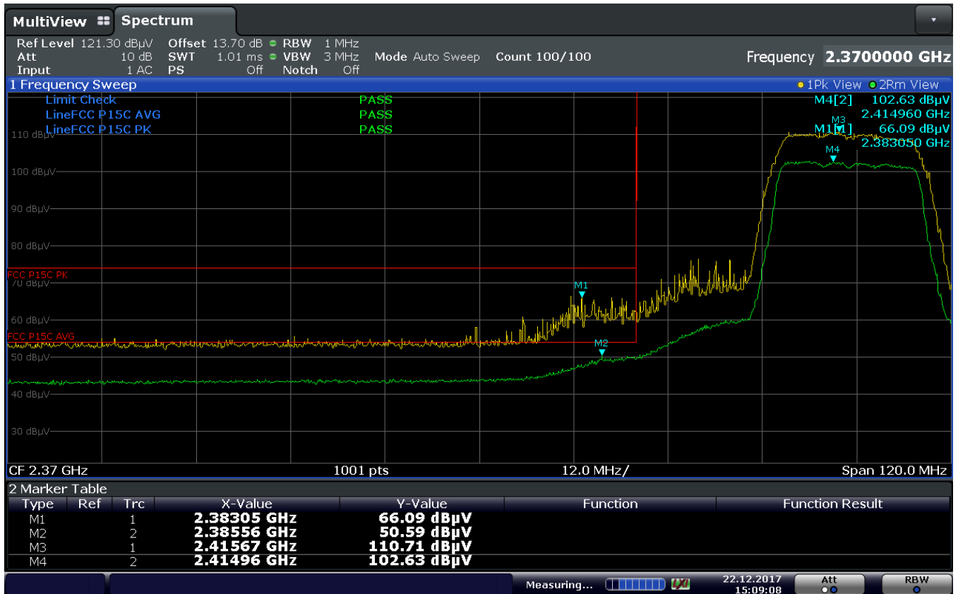
Plot 7-195. Radiated Restricted Upper Band Edge Measurement (Average & Peak)
