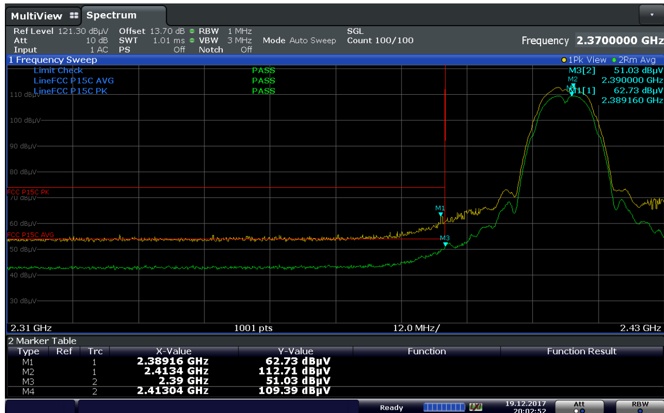
Plot 7-171. Radiated Restricted Lower Band Edge Measurement (Average & Peak)
