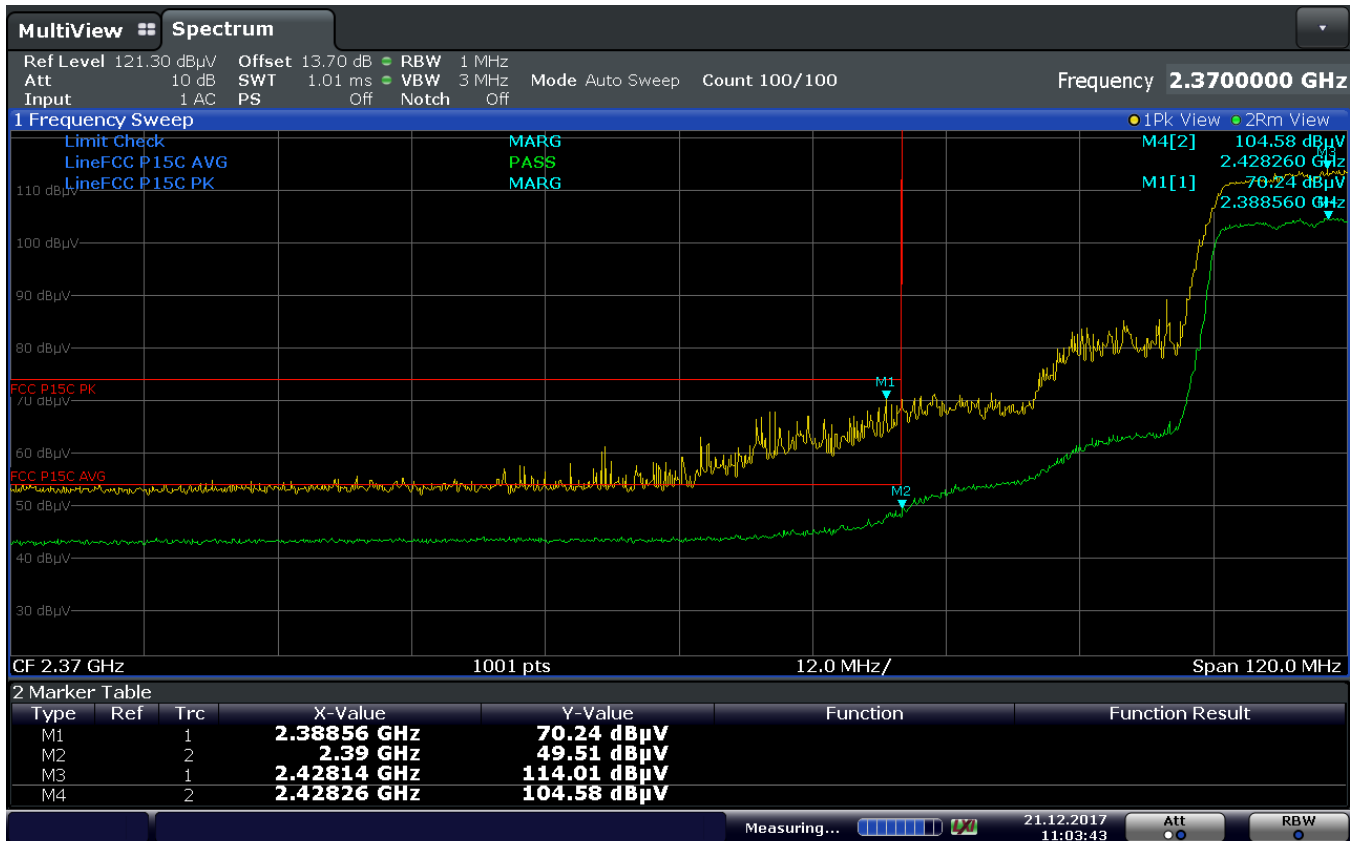
Plot 7-197. Radiated Restricted Upper Band Edge Measurement (Average & Peak)
