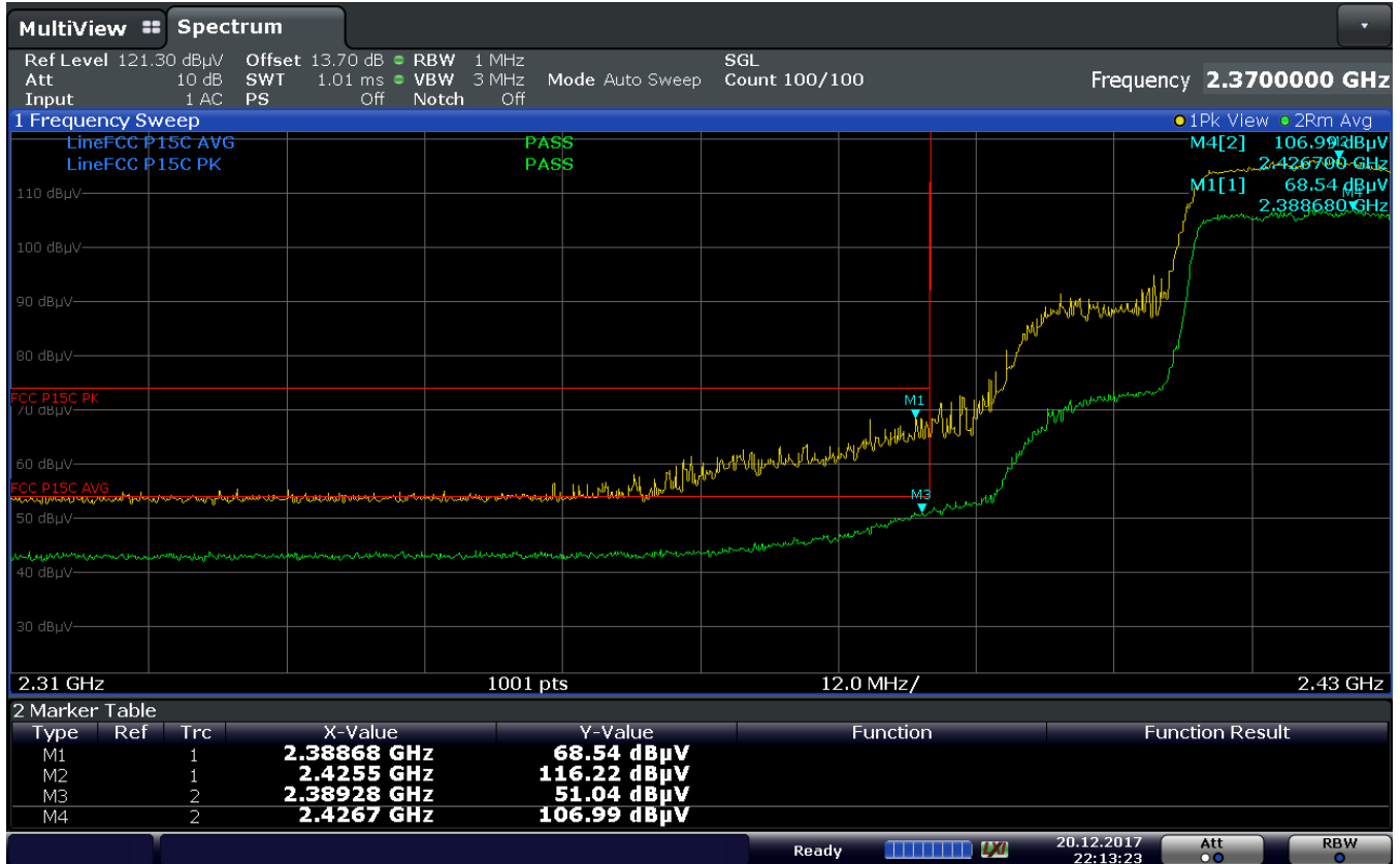
Plot 7-179. Radiated Restricted Lower Band Edge Measurement (Average & Peak)
