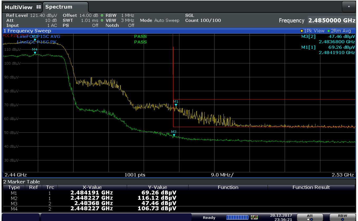
Plot 7-183. Radiated Restricted Upper Band Edge Measurement (Average & Peak)
