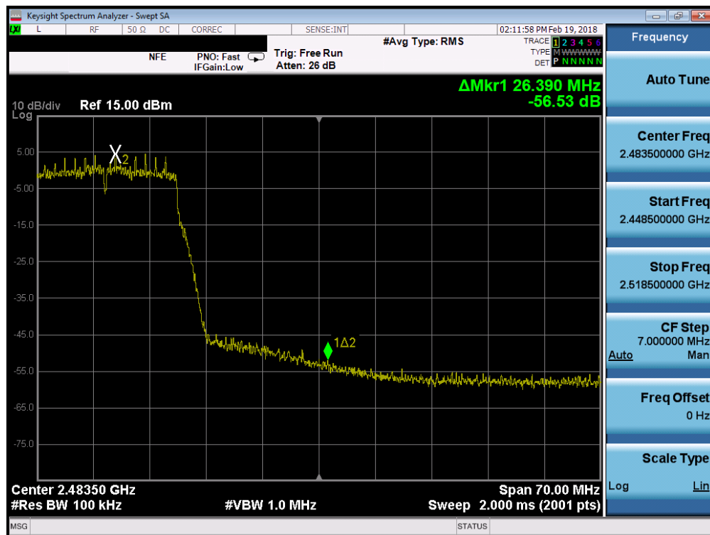
Plot 7-113. Band Edge Plot SISO ANT2 (802.11n (2.4GHz) – Ch. 10)
