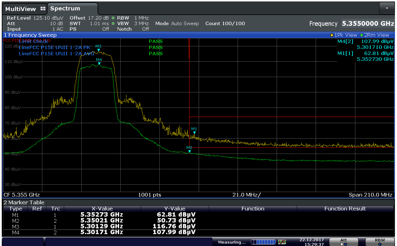
Plot 7-327. Radiated Restricted Upper Band Edge Measurement SISO ANT2 (Average & Peak UNII Band 2A)
