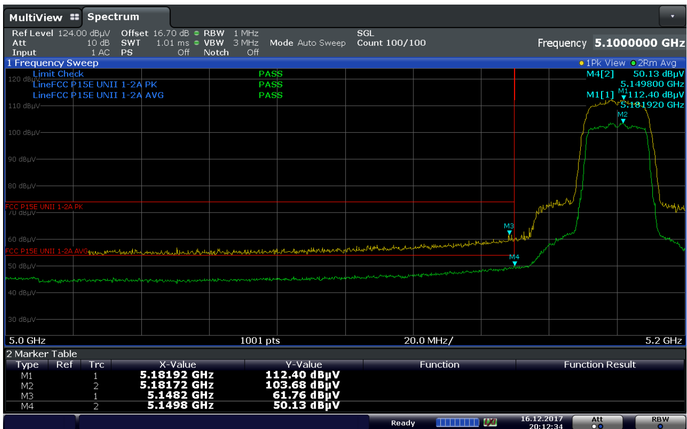
Plot 7-298. Radiated Restricted Lower Band Edge Measurement SISO ANT1 (Average & Peak UNII Band 1)
