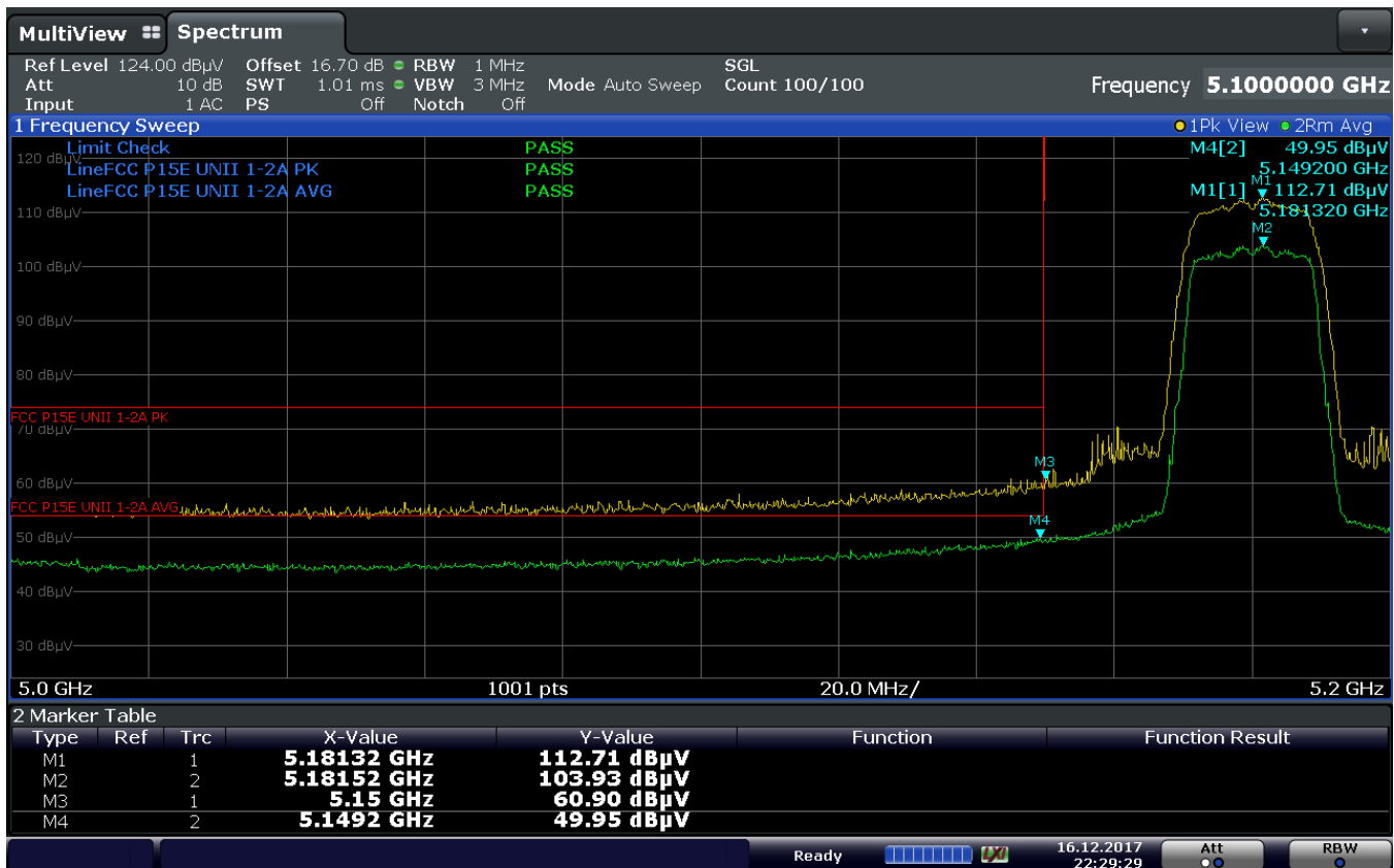
Plot 7-325. Radiated Restricted Lower Band Edge Measurement SISO ANT2 (Average & Peak UNII Band 1)
