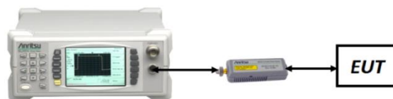
Figure 7-2. Test Instrument & Measurement Setup for Peak & Average Power Measurement
