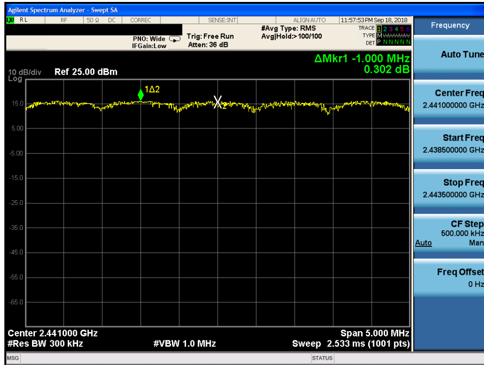
Plot 7-48. Channel Spacing Plot ANT2 (Bluetooth, 8DPSK, ePA)
