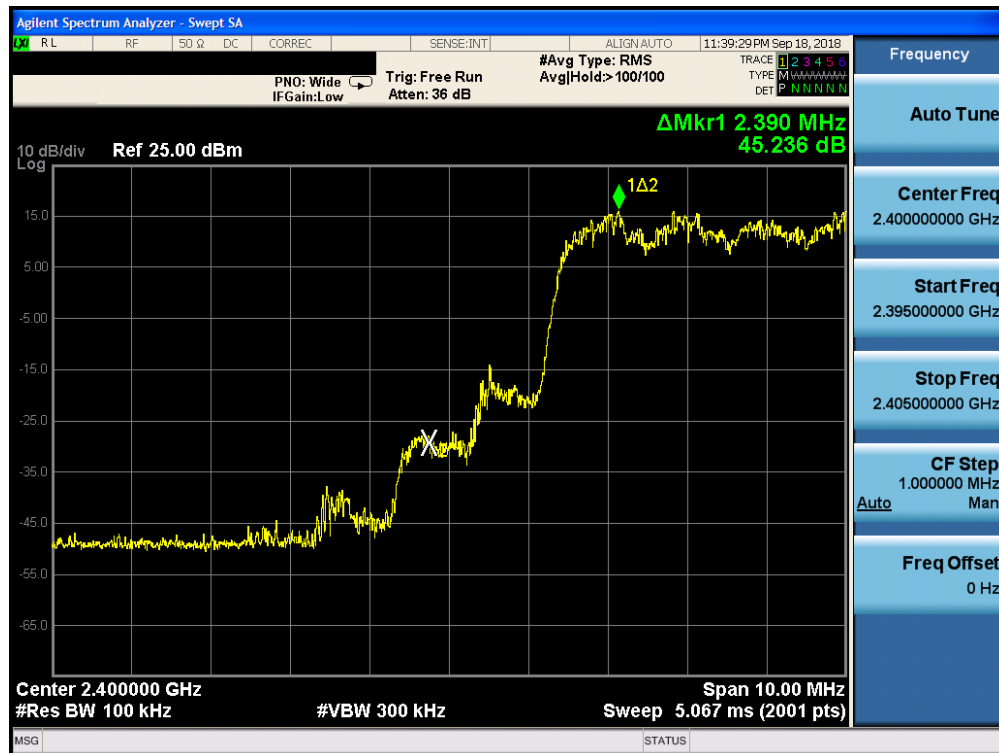
Plot 7-41. Band Edge Plot ANT 2 (Bluetooth with Hopping Enabled, 8DPSK, ePA)
