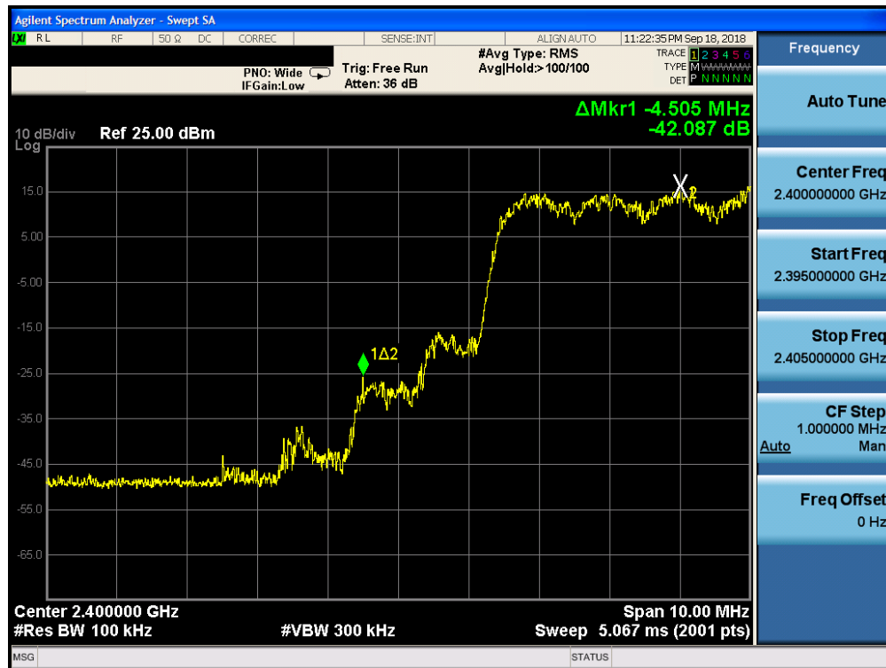
Plot 7-33. Band Edge Plot ANT 1 (Bluetooth with Hopping Enabled, 8DPSK, ePA)
