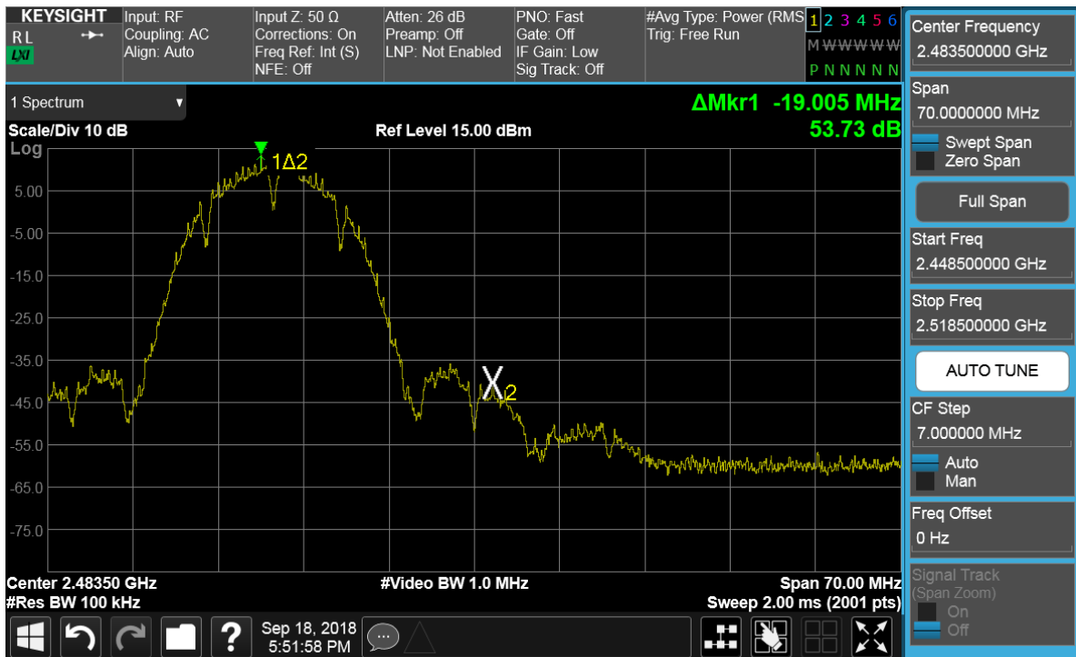
Plot 7-105. Band Edge Plot SISO Core 1 Diversity (802.11b – Ch. 12)
