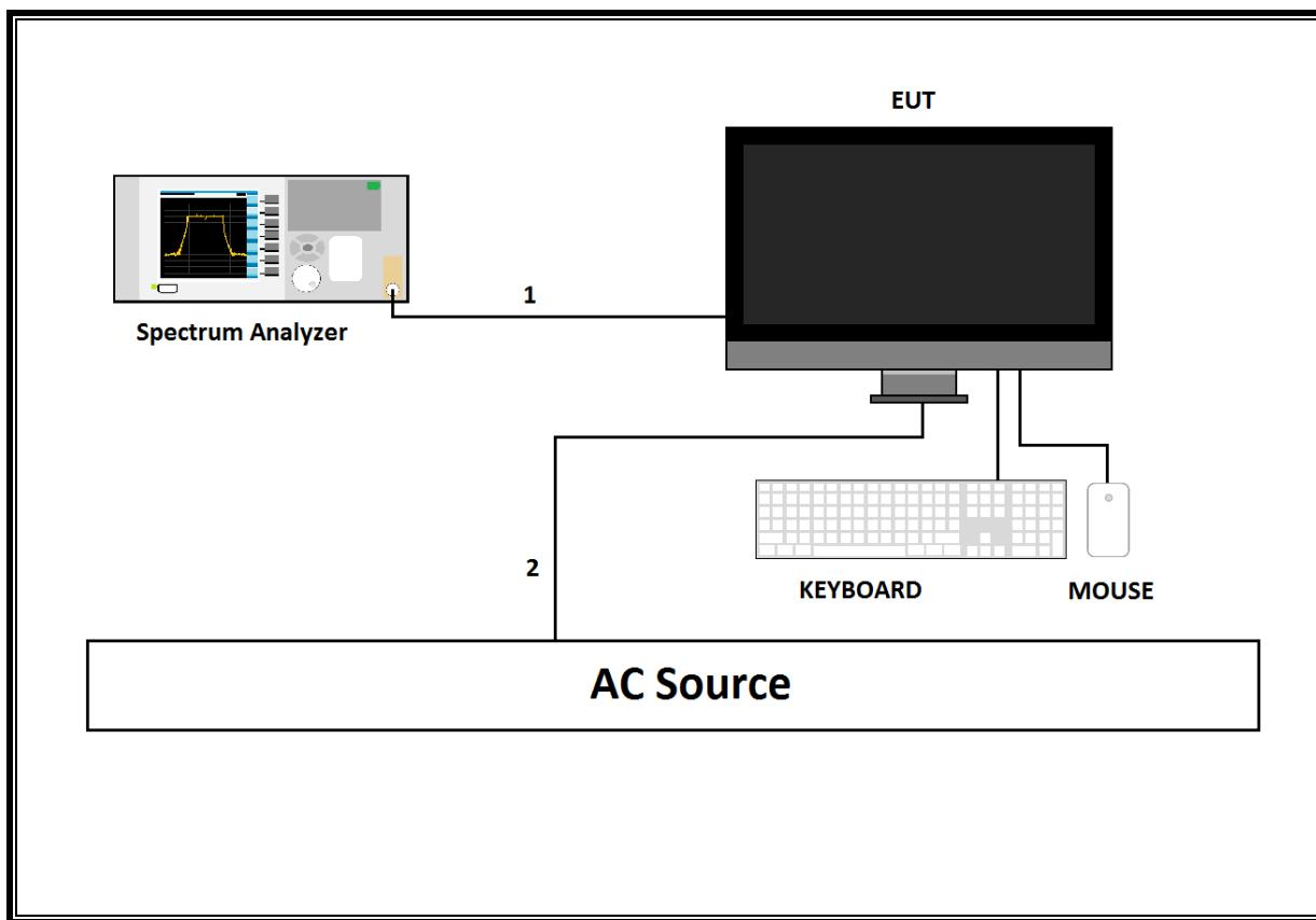
**SETUP DIAGRAM FOR RADIATED TESTS**
