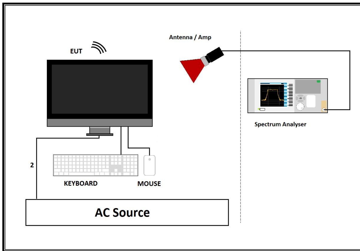
**SETUP DIAGRAM FOR BELOW 1GHz AND LINE CONDUCTED TEST**
