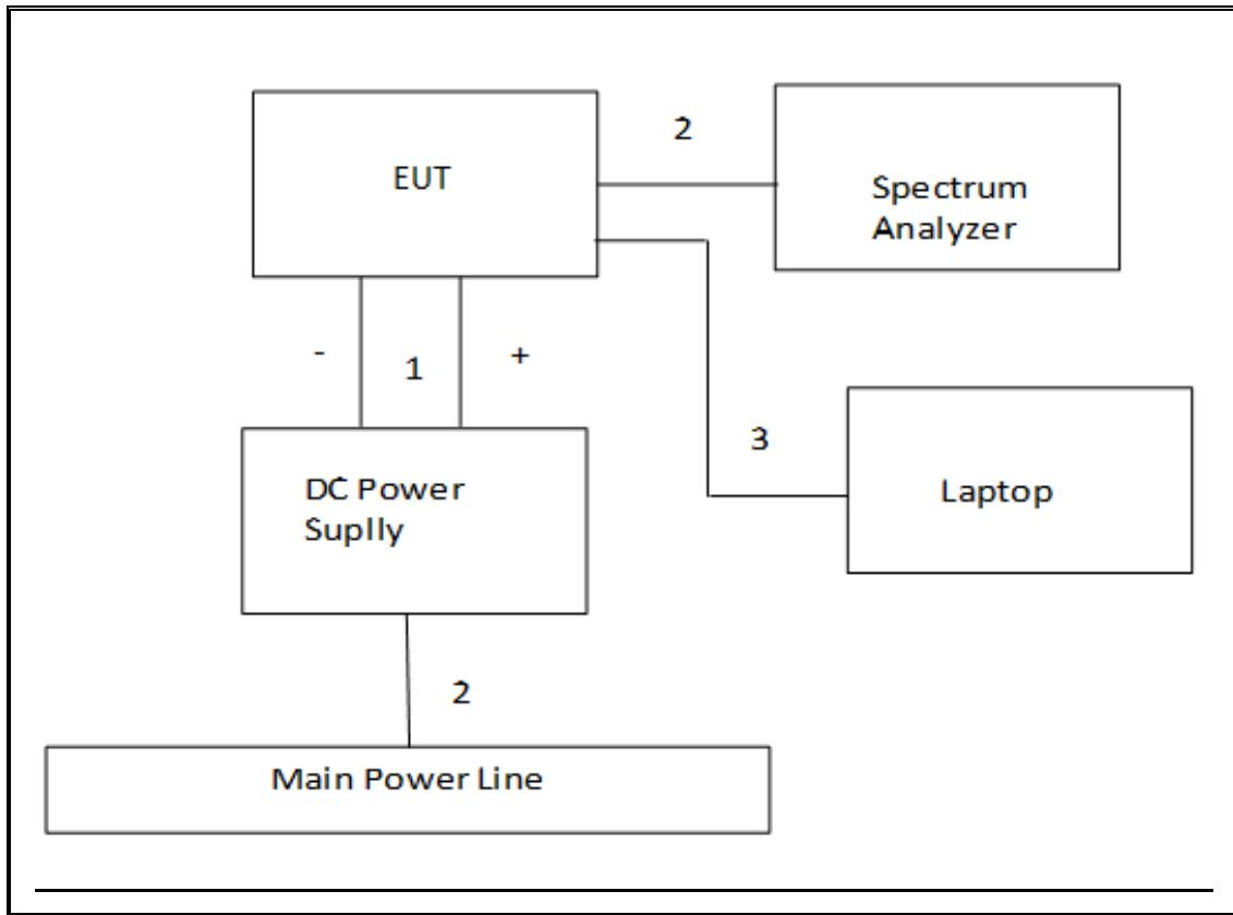
**TEST SETUP- RADIATED-ABOVE 1 GHZ**
