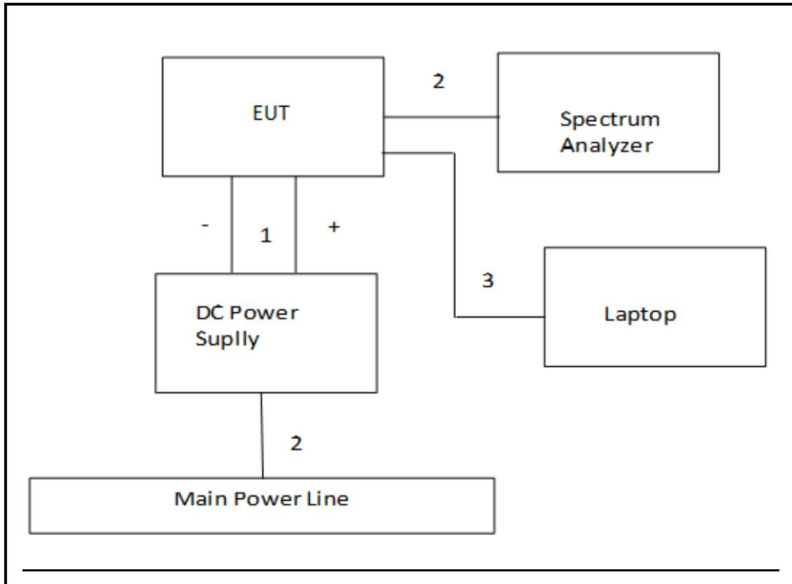
**TEST SETUP- RADIATED-ABOVE 1 GHZ**
