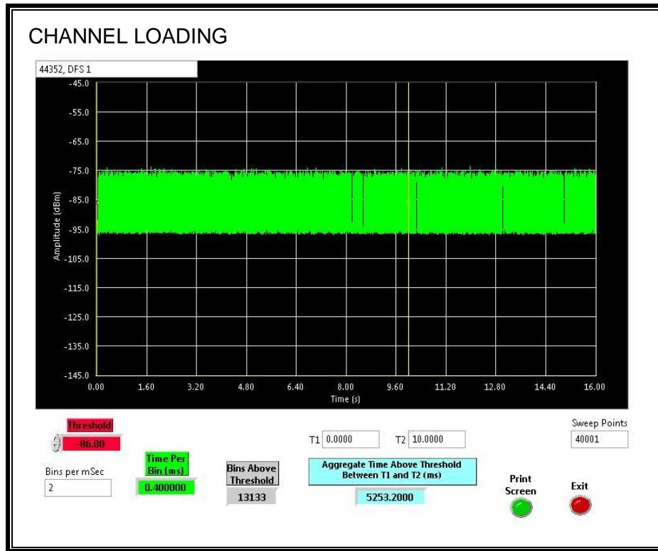
The level of traffic loading on the channel by the EUT is 52.532%
