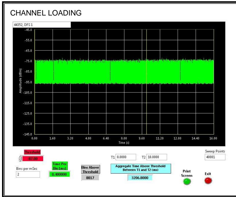
The level of traffic loading on the channel by the EUT is 32.068%
