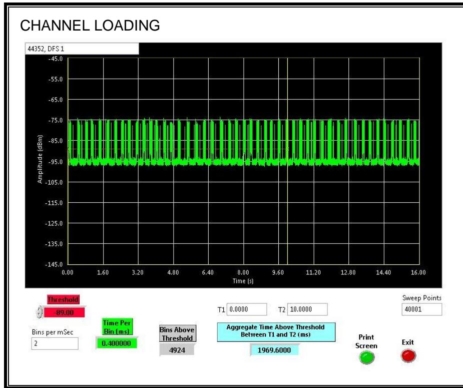
The level of traffic loading on the channel by the EUT is 19.696%
