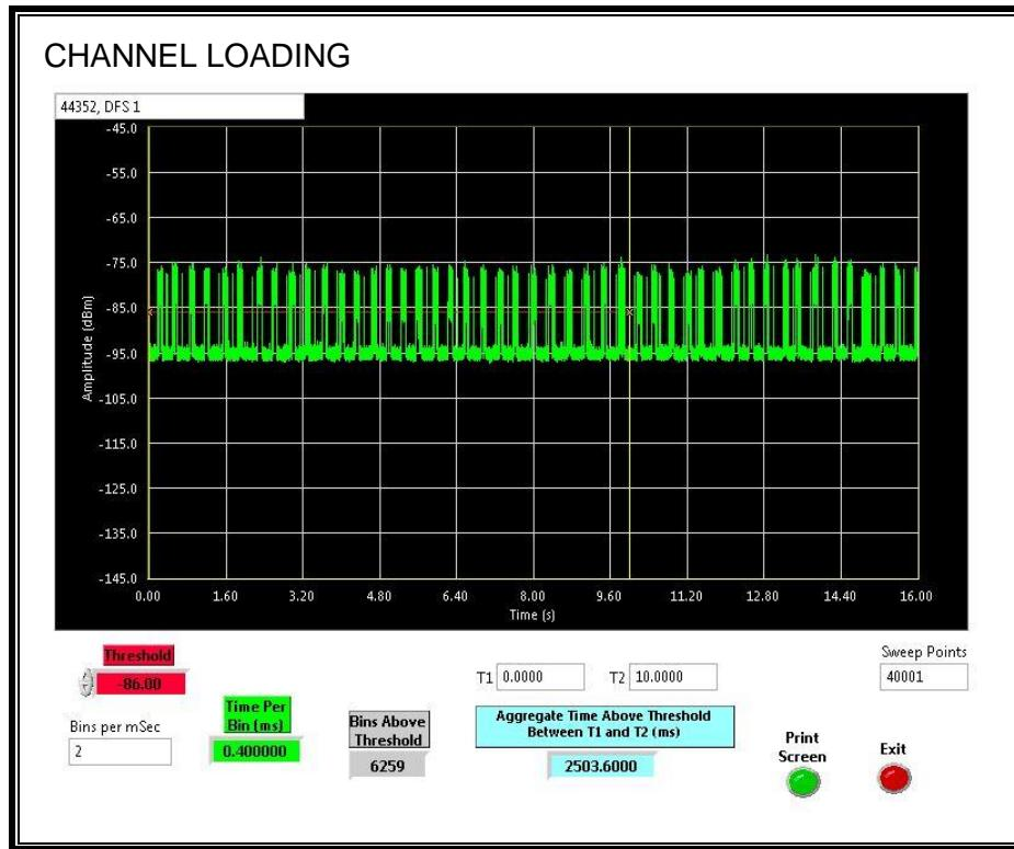
The level of traffic loading on the channel by the EUT is 25.036%
