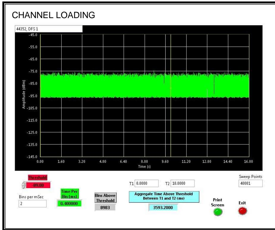
The level of traffic loading on the channel by the EUT is 35.932%
