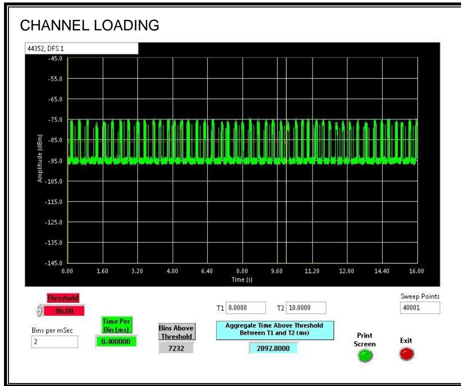
The level of traffic loading on the channel by the EUT is 28.928%
