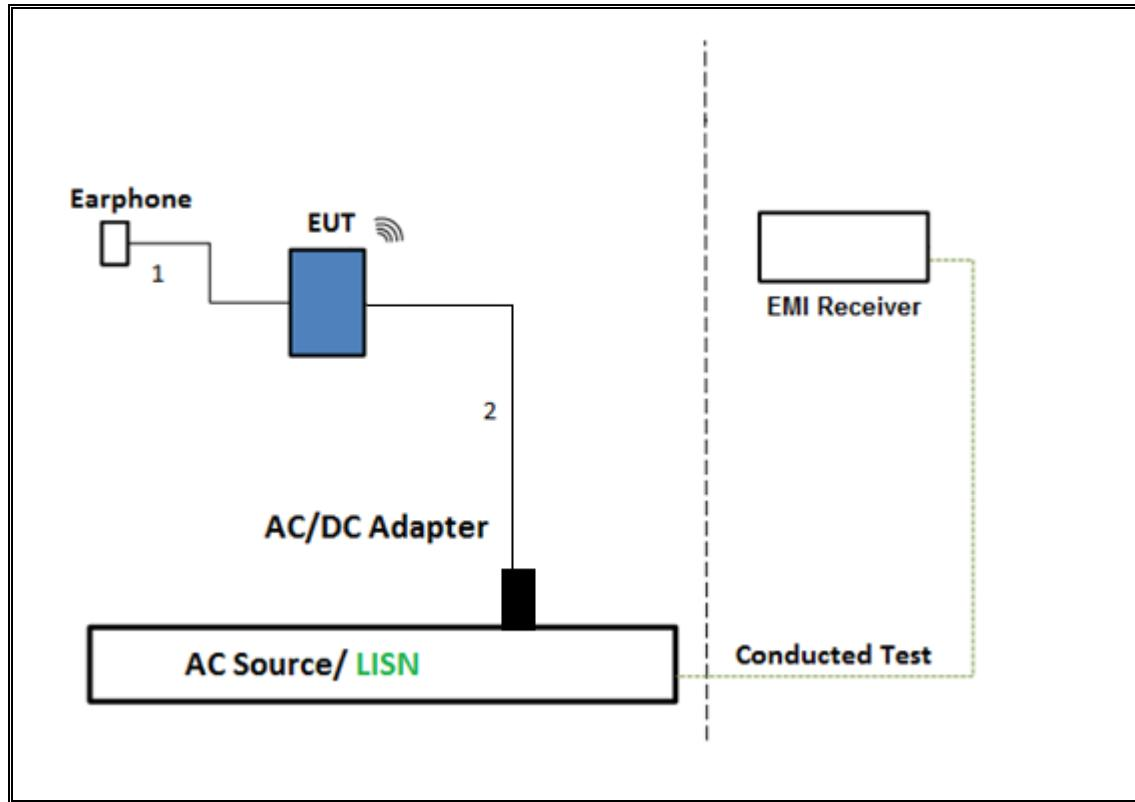
**TEST SETUP- AC LINE CONDUCTED: LAPTOP CONFIGURATION**
