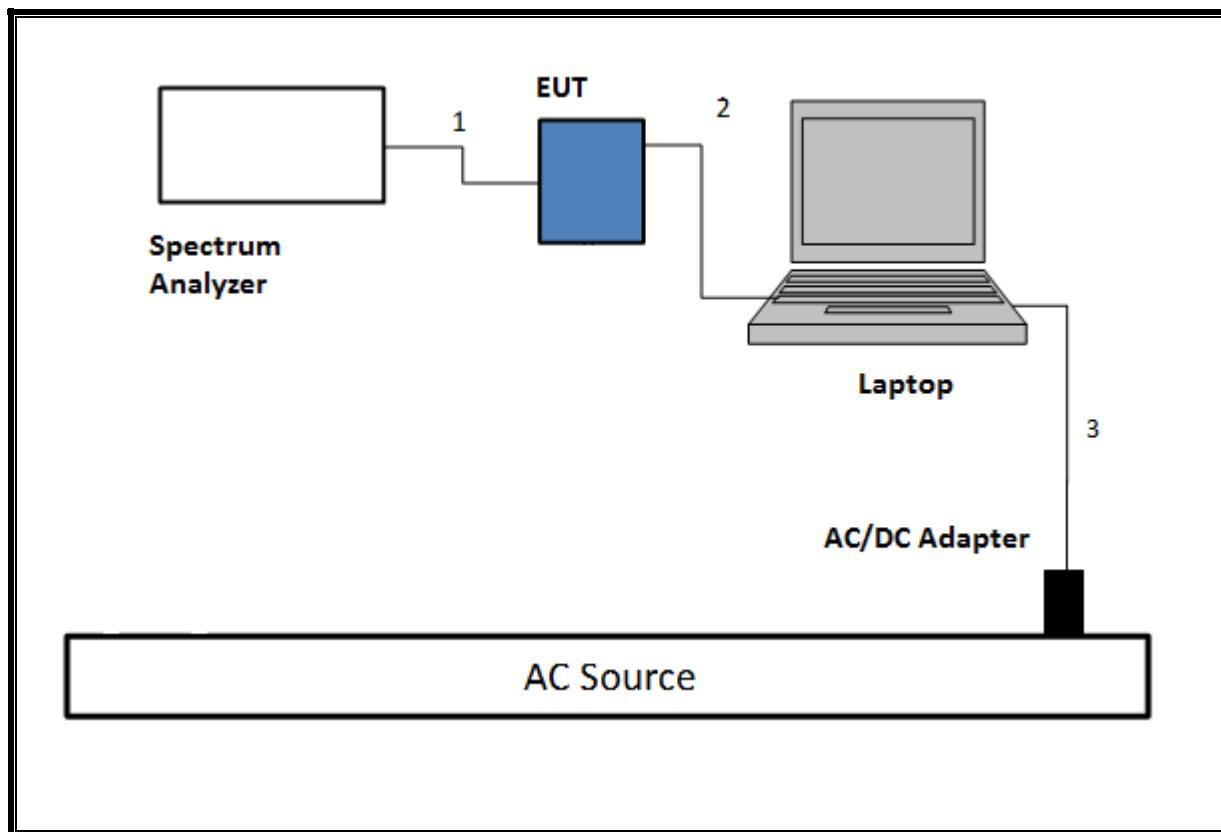
**TEST SETUP- RADIATED-ABOVE 1 GHZ**
