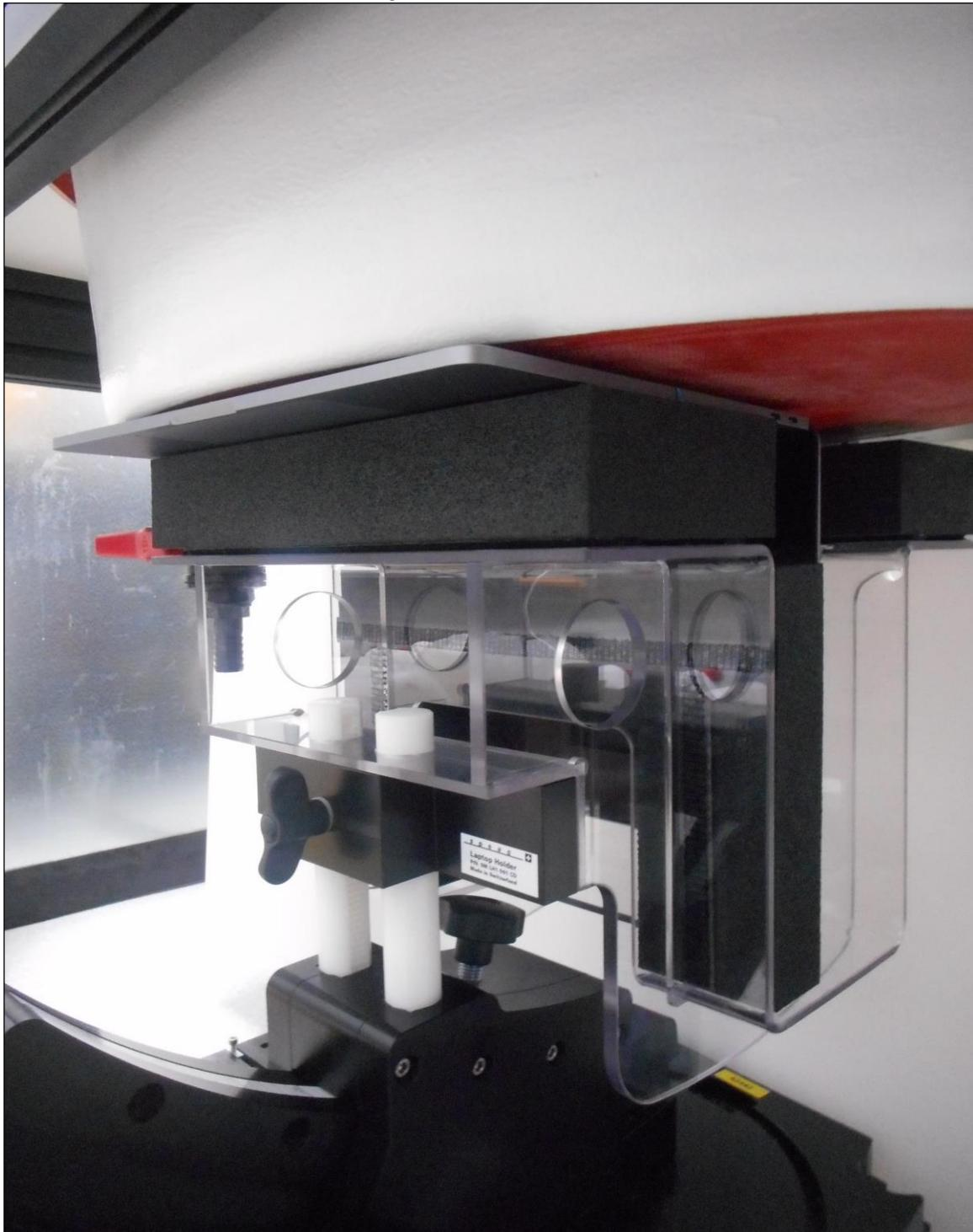
PHT/003: Display Side of EUT Facing Phantom
