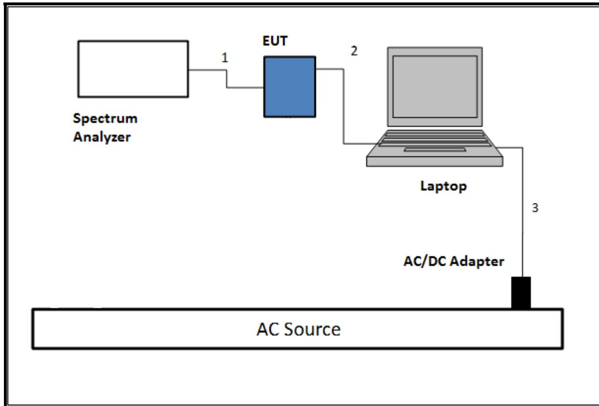
**TEST SETUP- RADIATED-ABOVE 1 GHZ**
