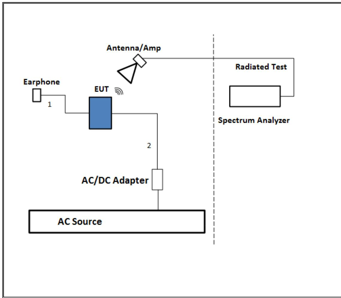
**TEST SETUP- AC LINE CONDUCTED: AC/DC ADAPTER**
