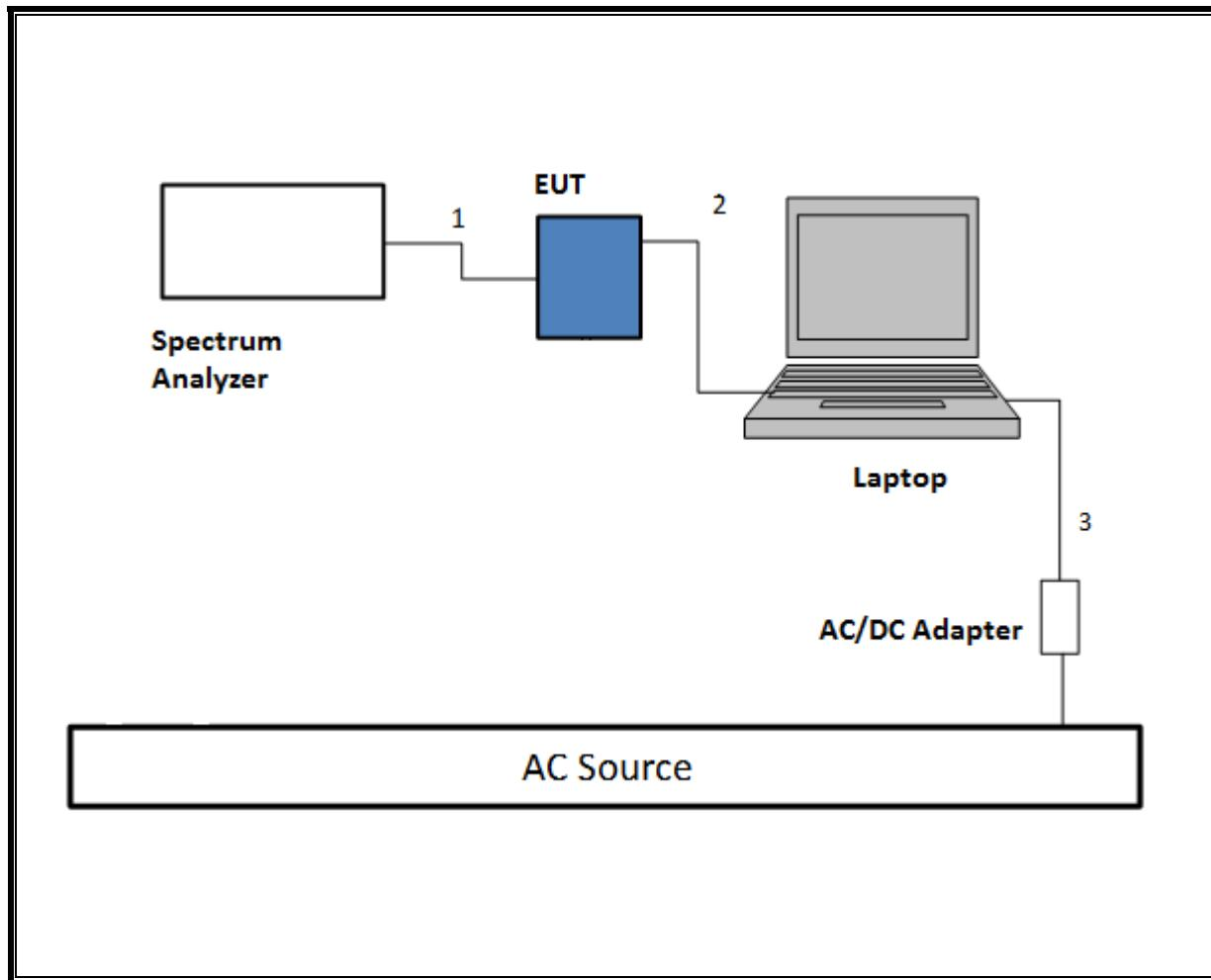
**TEST SETUP- RADIATED-ABOVE 1 GHZ**
