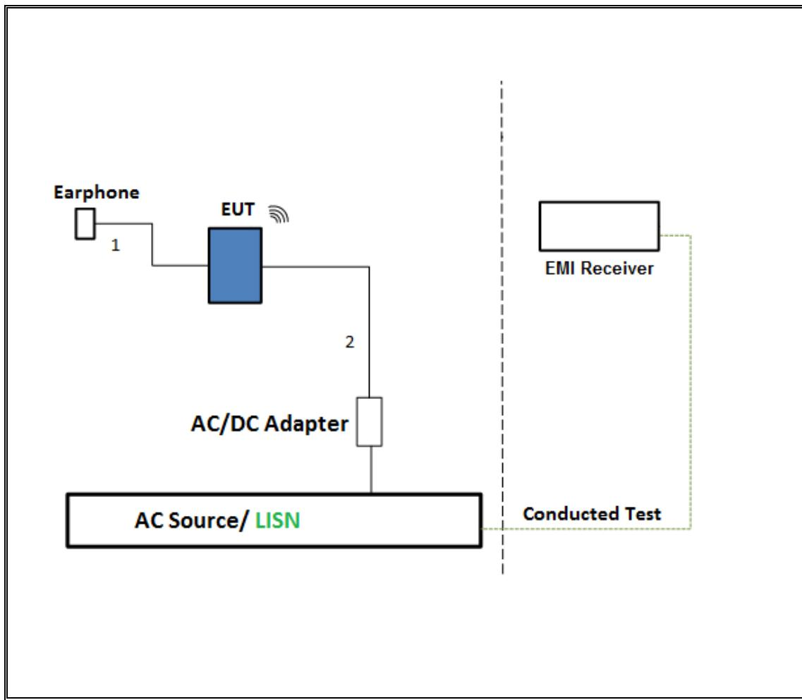
**TEST SETUP- AC LINE CONDUCTED: LAPTOP CONFIGURATION**
