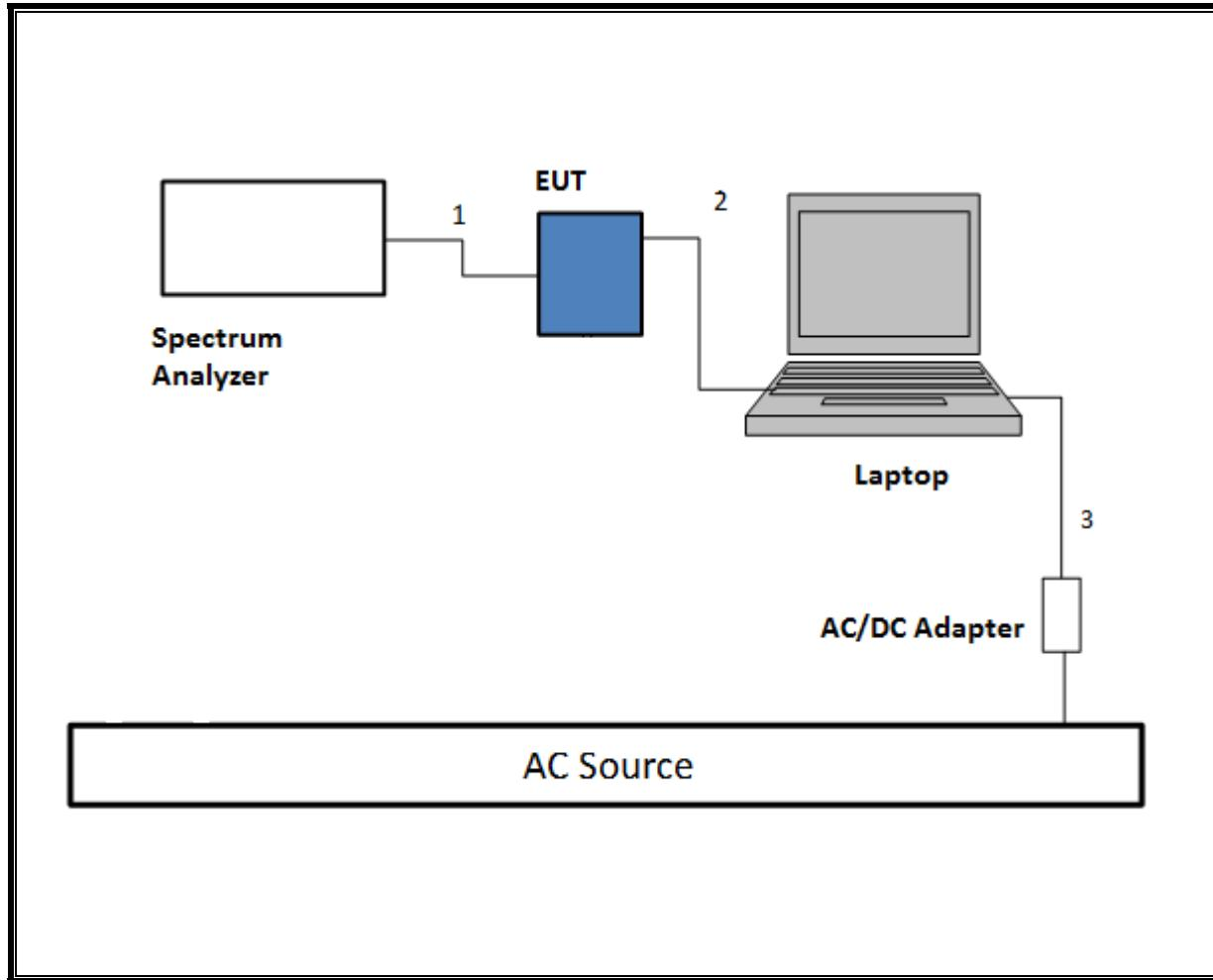
**TEST SETUP- RADIATED-ABOVE 1 GHZ**
