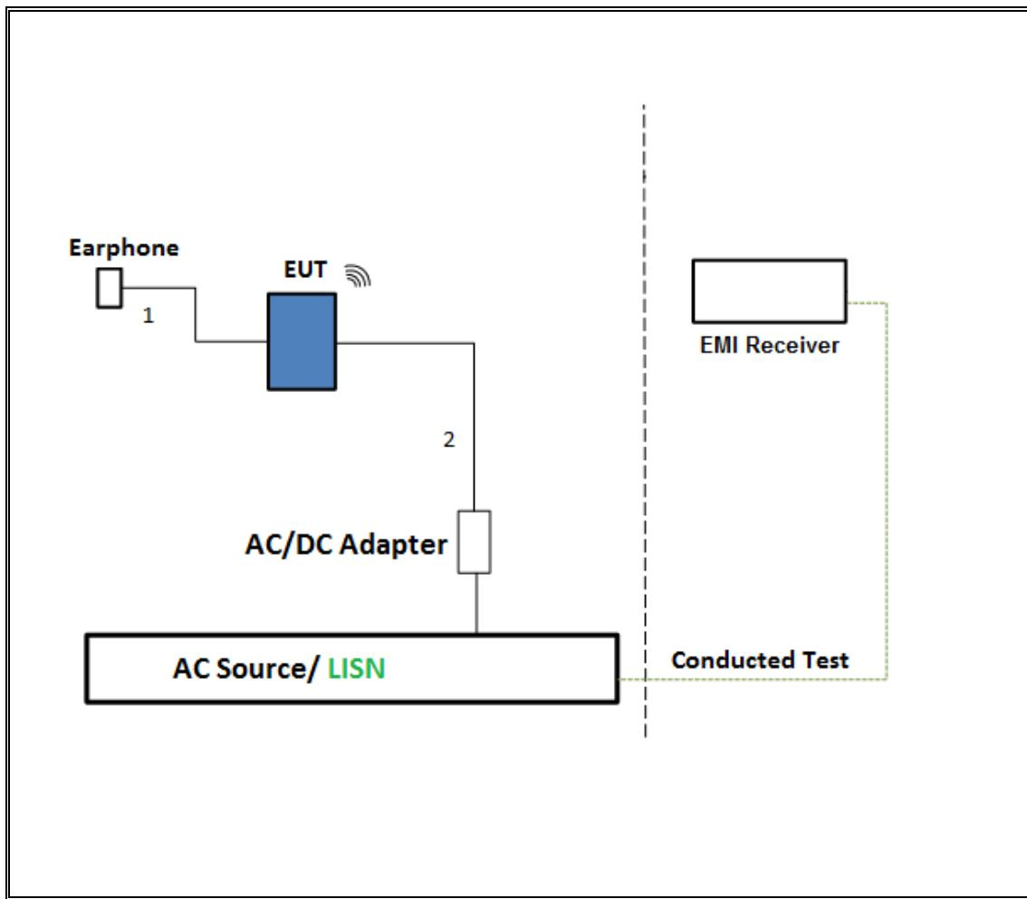
**TEST SETUP- AC LINE CONDUCTED: LAPTOP CONFIGURATION**
