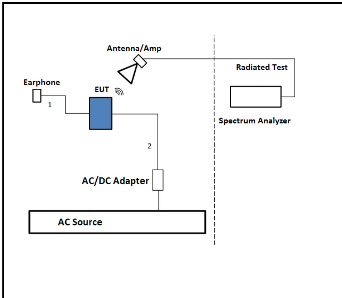
**TEST SETUP- AC LINE CONDUCTED: AC/DC ADAPTER**
