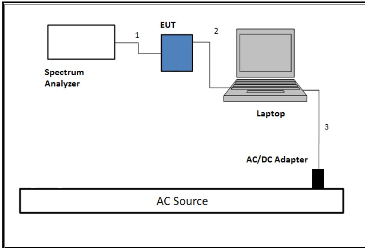
**TEST SETUP- RADIATED-ABOVE 1 GHZ**
