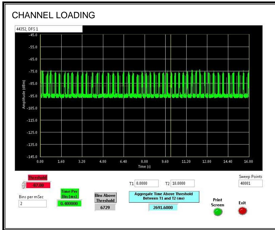
The level of traffic loading on the channel by the EUT is 26.916%
