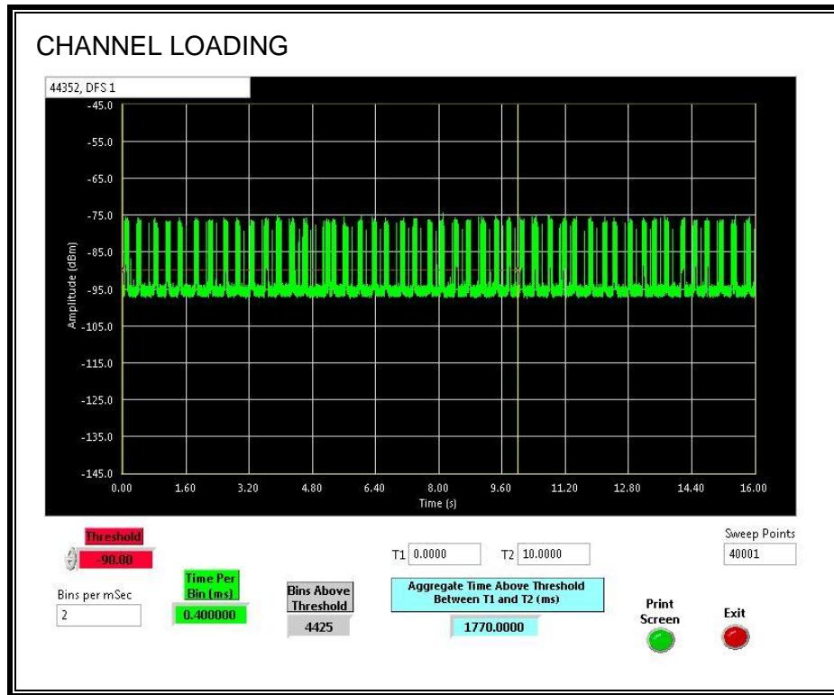
The level of traffic loading on the channel by the EUT is 17.7%
