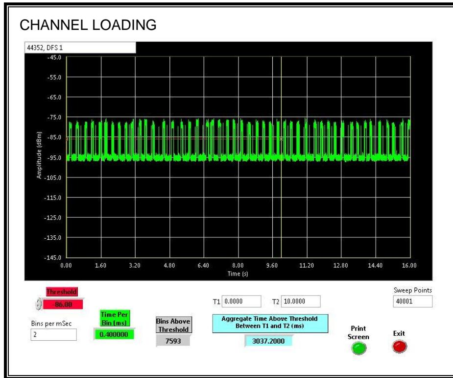
The level of traffic loading on the channel by the EUT is 30.372%
