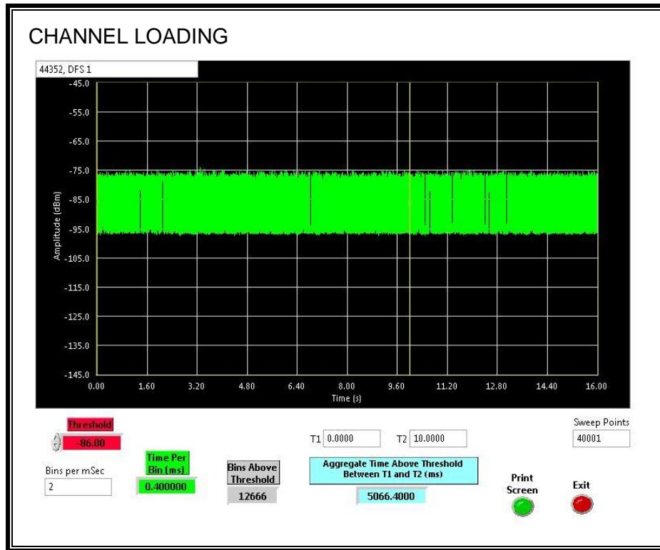
The level of traffic loading on the channel by the EUT is 50.664%
