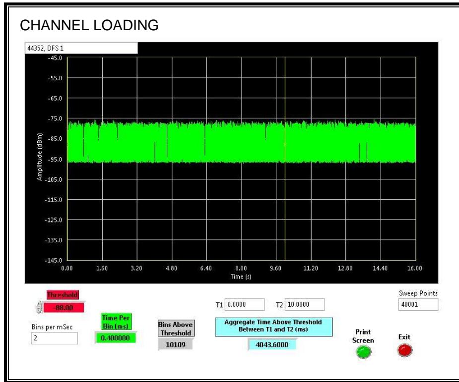
The level of traffic loading on the channel by the EUT is 40.436%
