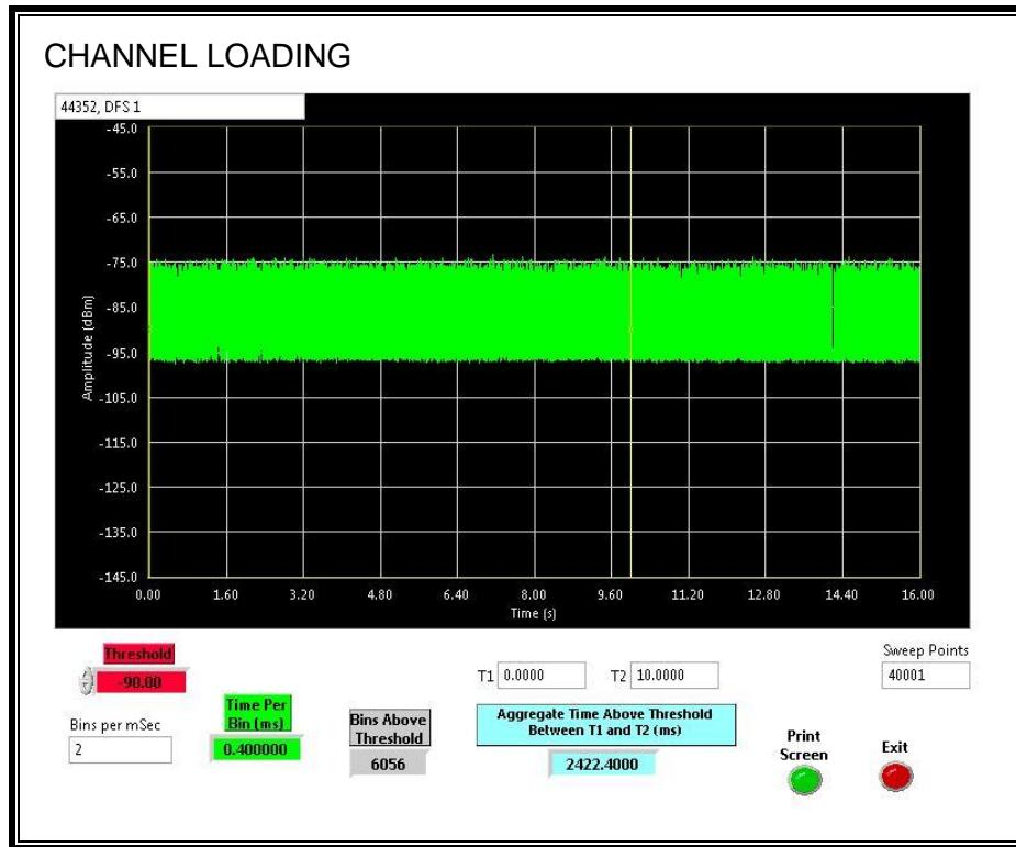
The level of traffic loading on the channel by the EUT is 24.224%
