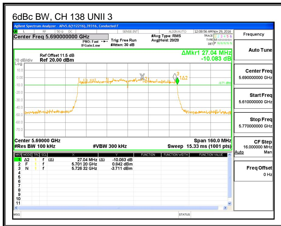
**8.39. 802.11ac VHT80 2Tx (ANTENNA A + ANTENNA B) CDD MODE IN THE 5.6 GHz BAND (5610MHz for FCC only)**
