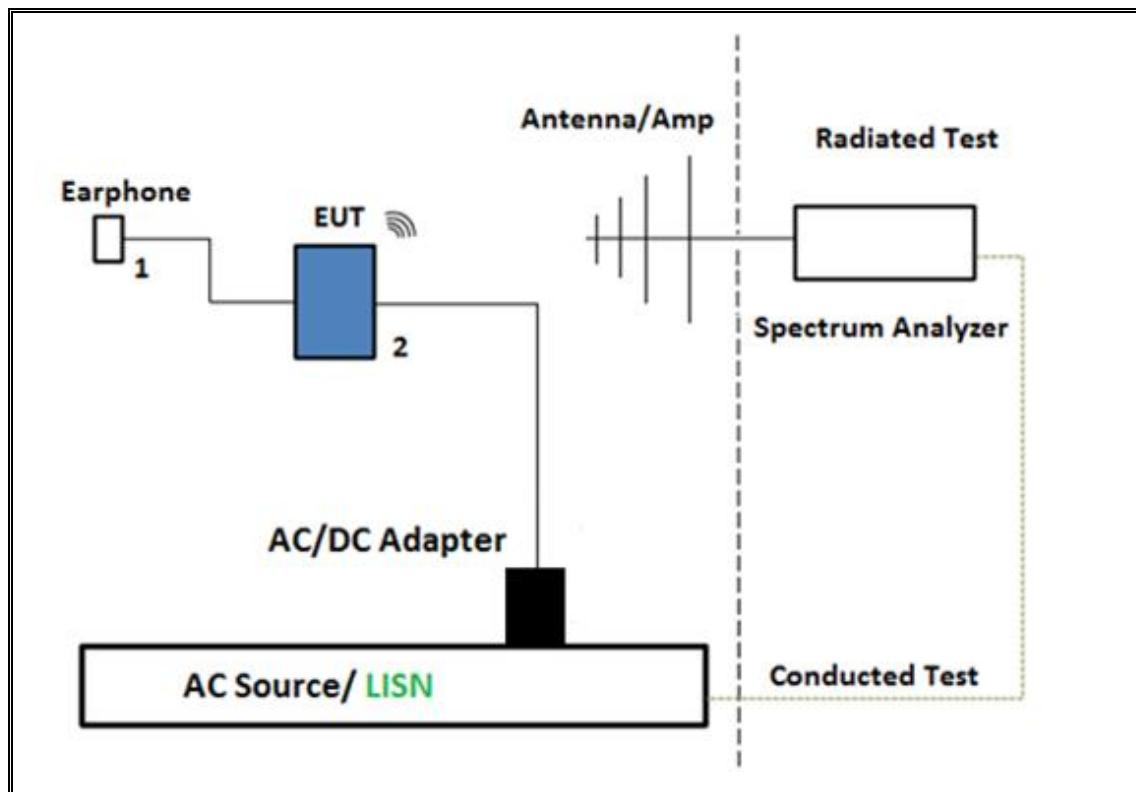
**TEST SETUP- AC LINE CONDUCTED: AC/DC ADAPTER CONFIGURATION**
