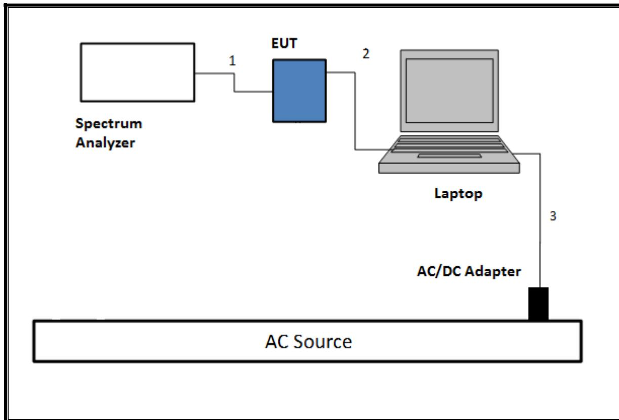
**TEST SETUP- RADIATED-ABOVE 1 GHZ**
