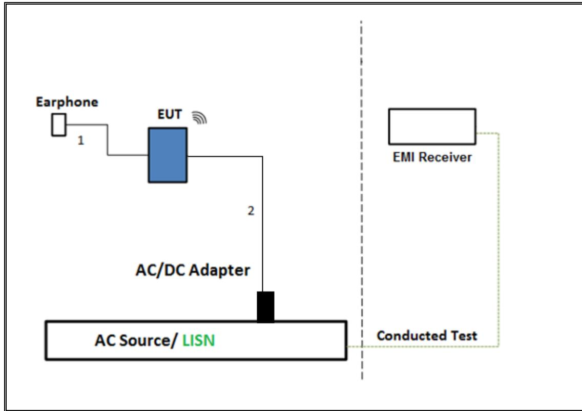
**TEST SETUP- AC LINE CONDUCTED: LAPTOP CONFIGURATION**
