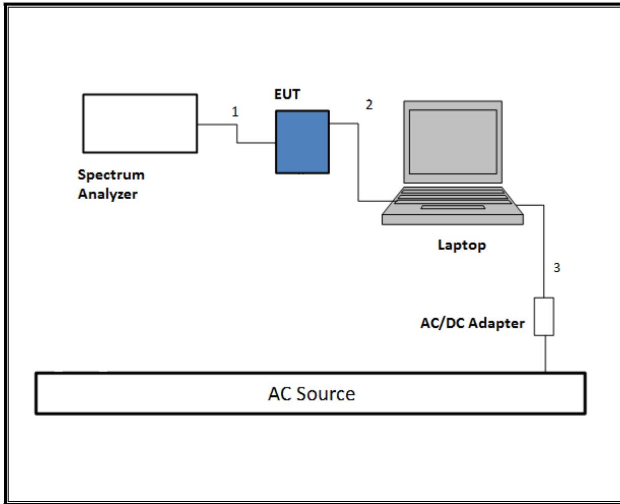
**TEST SETUP- RADIATED-ABOVE 1 GHZ**
