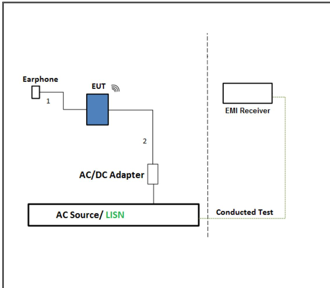
**TEST SETUP- AC LINE CONDUCTED: LAPTOP CONFIGURATION**
