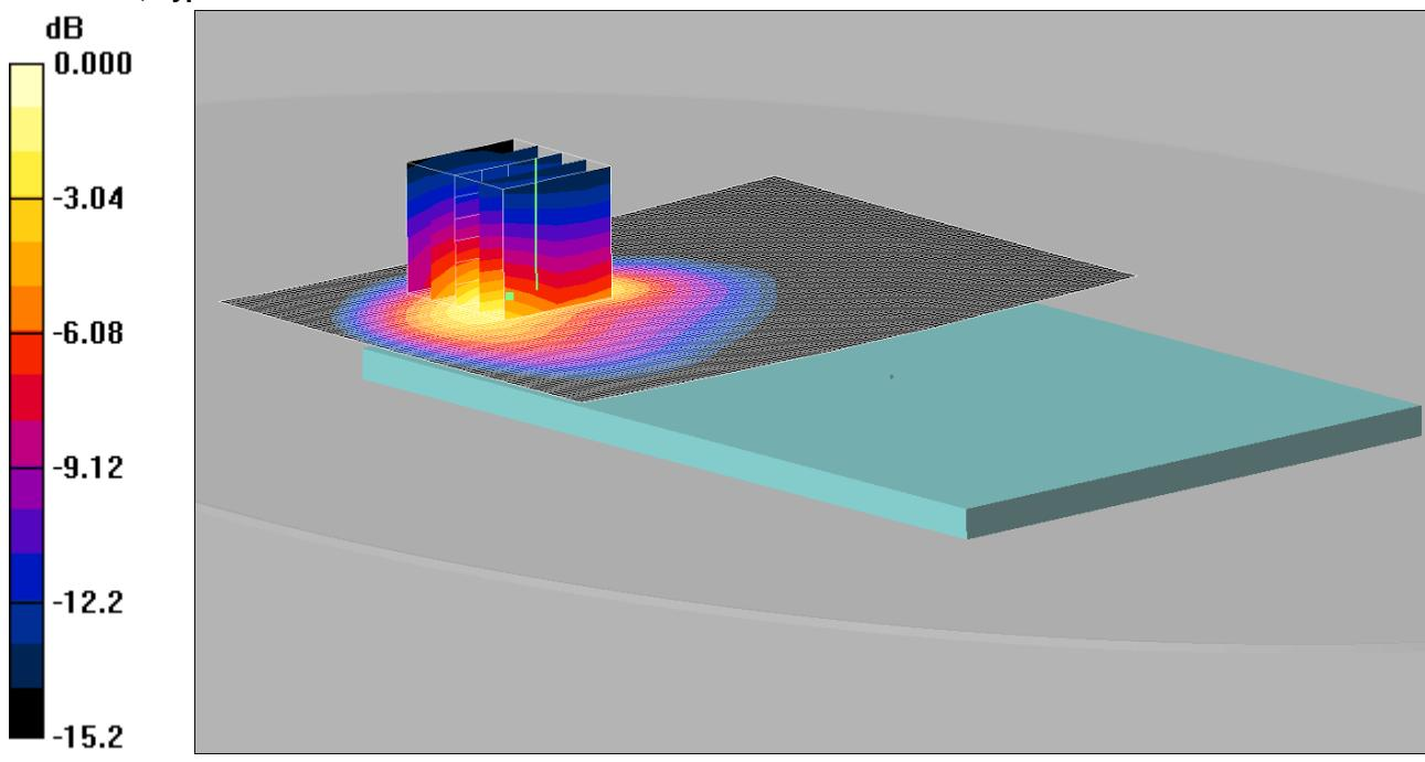
Communication System: LTE - Band 17 / 10MHz Channel; Frequency: 709 MHz; Duty Cycle: 1:1
