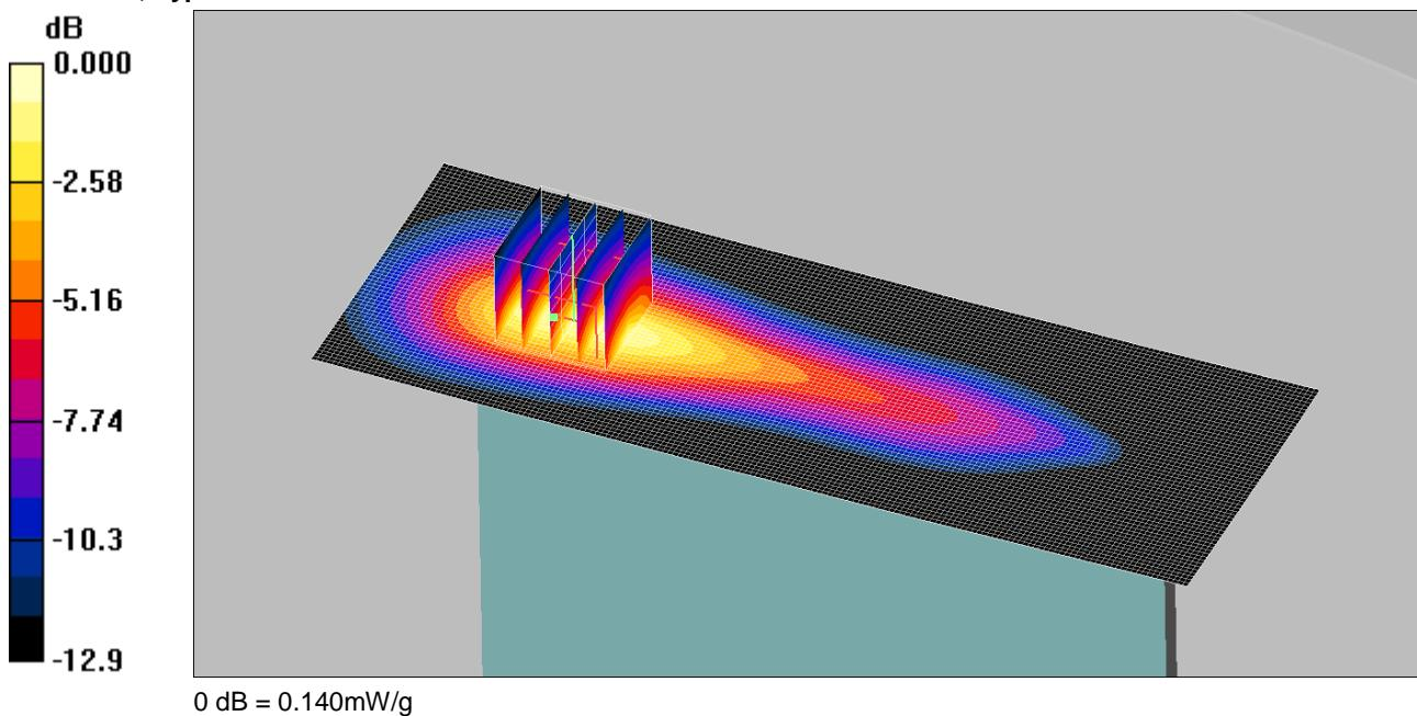
Communication System: LTE - Band 13 / 10MHz Channel; Frequency: 782 MHz; Duty Cycle: 1:1
