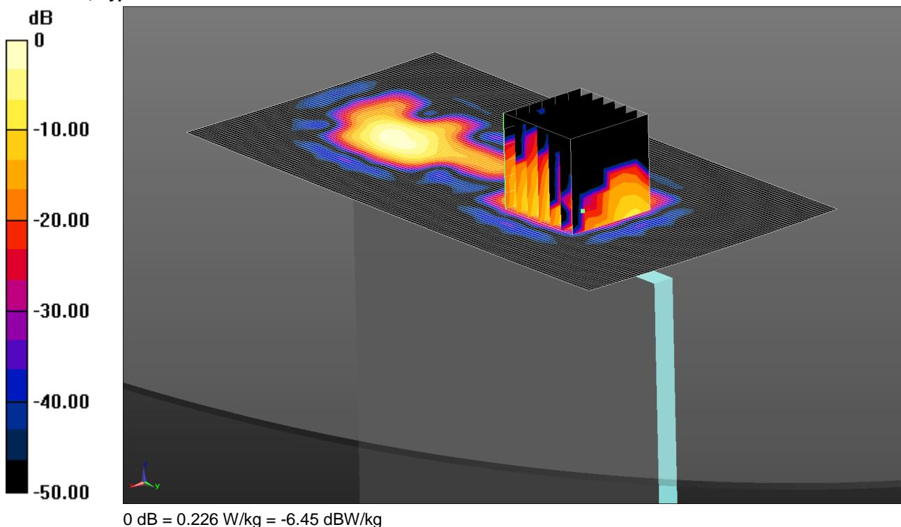
Communication System: UID 0, WLAN 802.11 (0); Frequency: 2412 MHz; Duty Cycle: 1:1
