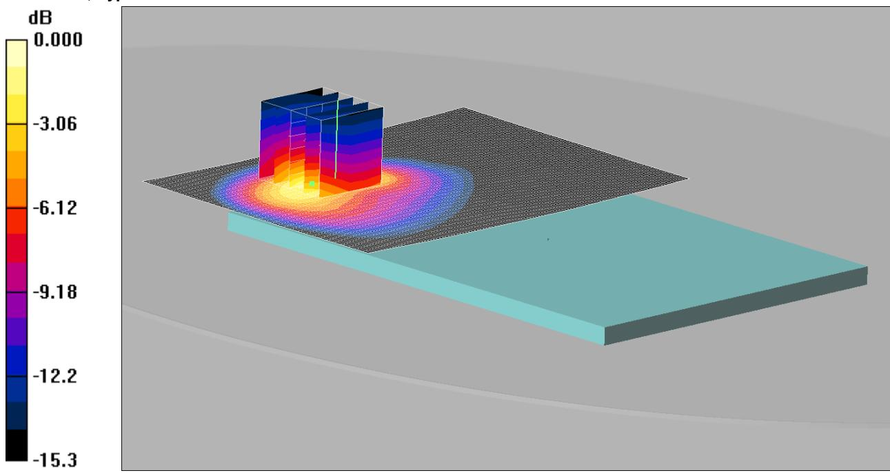
Communication System: LTE - Band 17 / 10MHz Channel; Frequency: 711 MHz; Duty Cycle: 1:1
