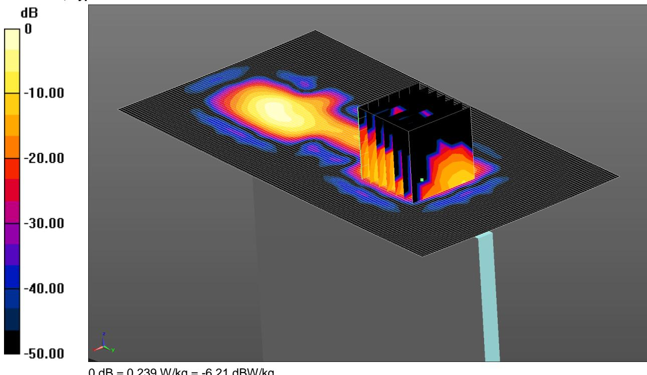
Communication System: UID 0, WLAN 802.11 (0); Frequency: 2462 MHz; Duty Cycle: 1:1
