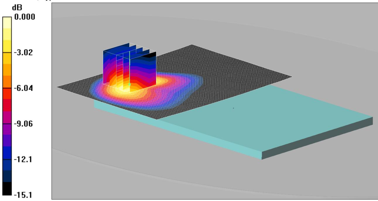
Communication System: LTE - Band 13 / 10MHz Channel; Frequency: 782 MHz; Duty Cycle: 1:1
