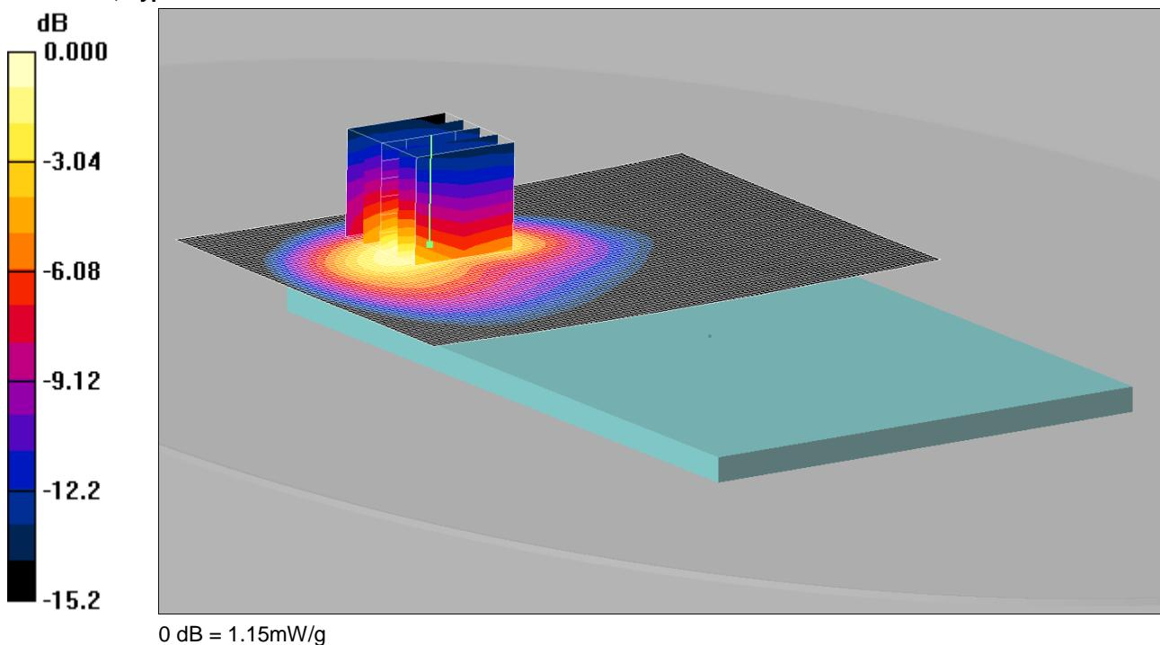
Communication System: LTE - Band 17 / 10MHz Channel; Frequency: 711 MHz; Duty Cycle: 1:1
