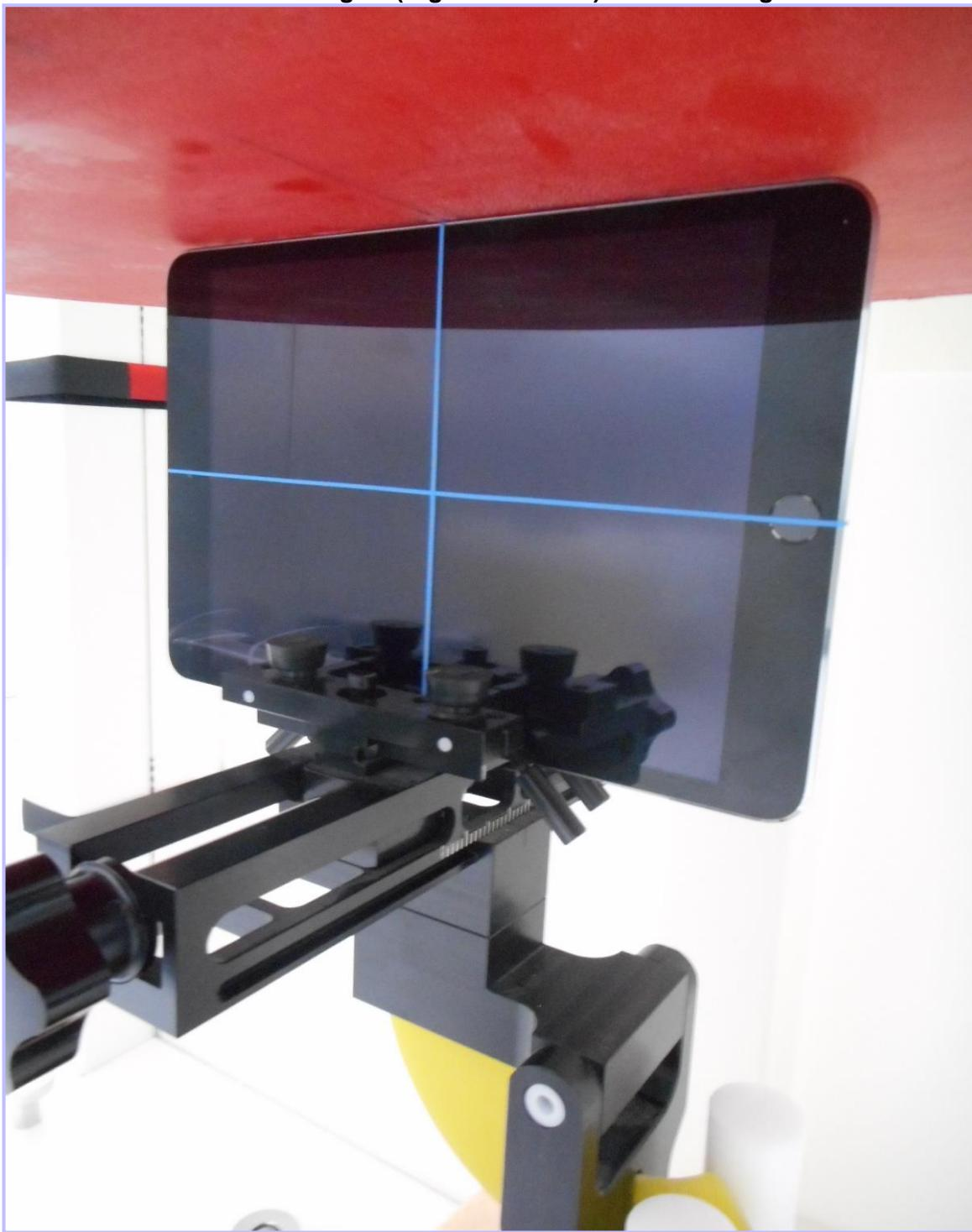
**PHT/10407443JD13A/004: Edge 3 (Bottom) of EUT Facing Phantom at 0mm Separation**
