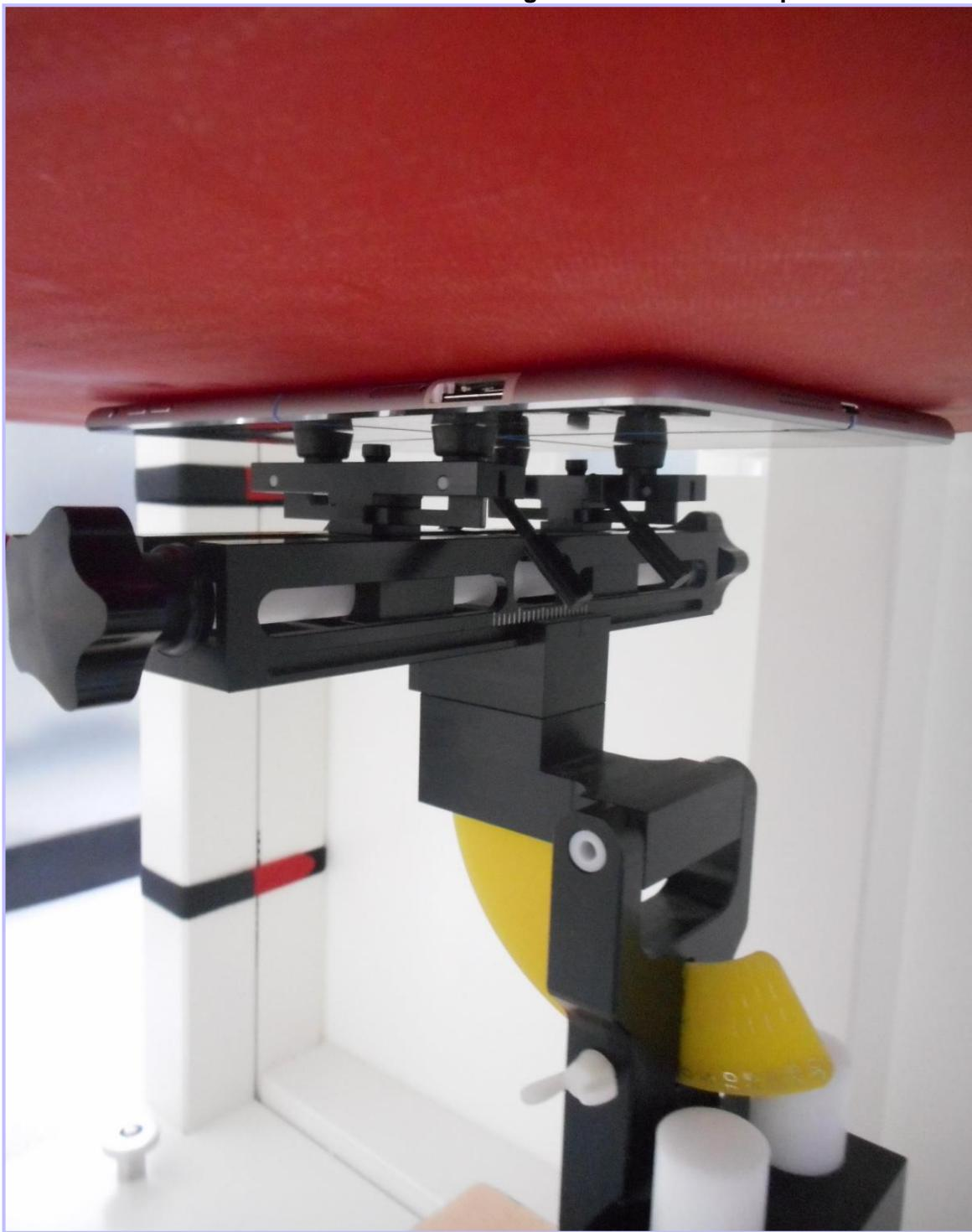
**PHT/10407443JD13A/002: Edge 1 (Top) of EUT Facing Phantom at 0mm Separation**
