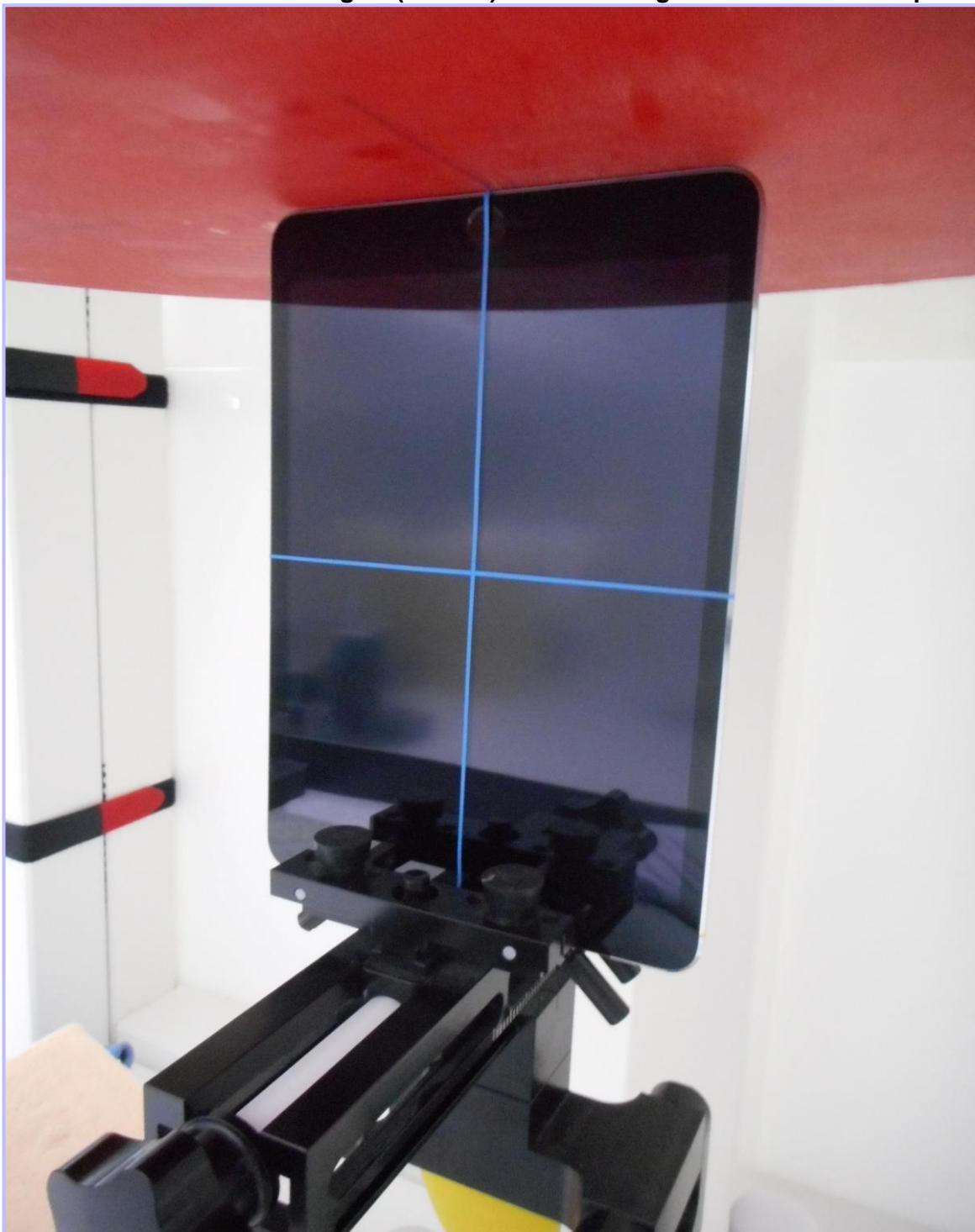
**PHT/10407443JD13A/005: Edge 4 (Left Hand Side) of EUT Facing Phantom at 0mm Separation**
