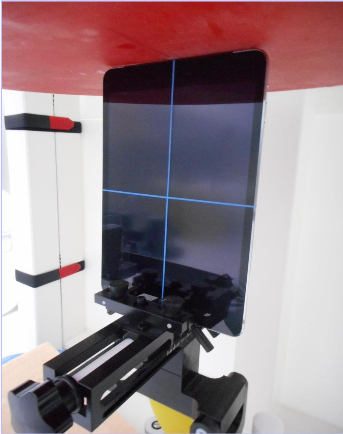
**PHT/10407443JD13A/003: Edge 2 (Right Hand Side) of EUT Facing Phantom at 0mm Separation**
