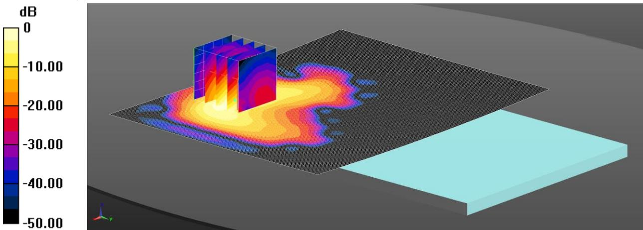
Communication System: UID 0, CDMA2000 (0); Frequency: 1732.5 MHz; Duty Cycle: 1:1
