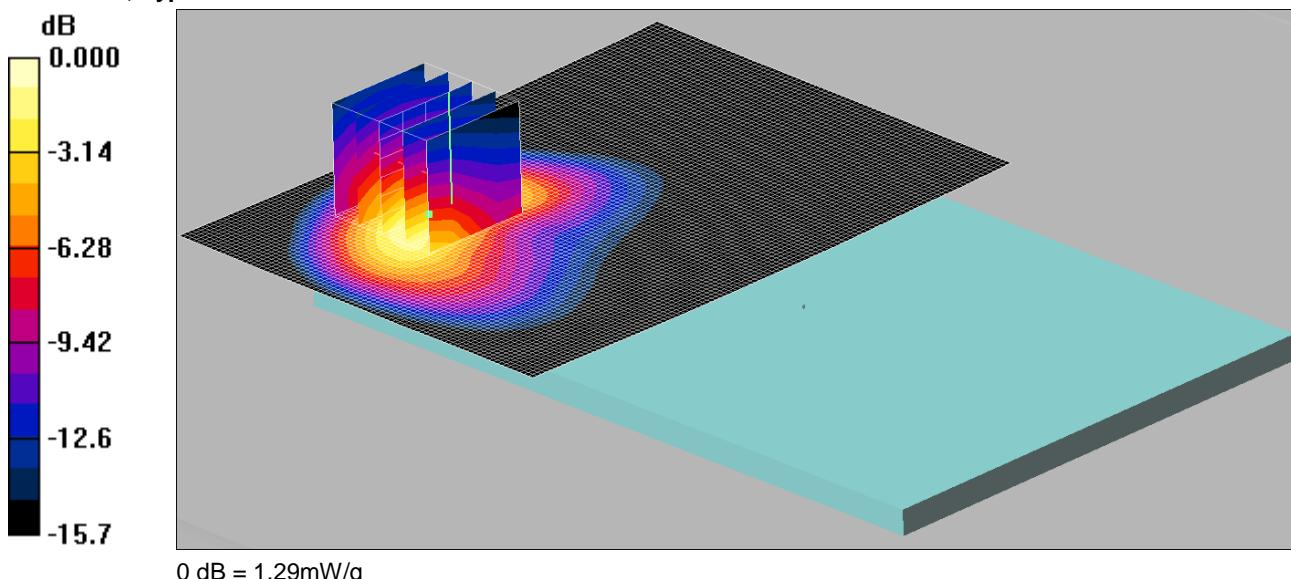
Communication System: LTE Band 5 / 10MHz; Frequency: 836.5 MHz; Duty Cycle: 1:1
