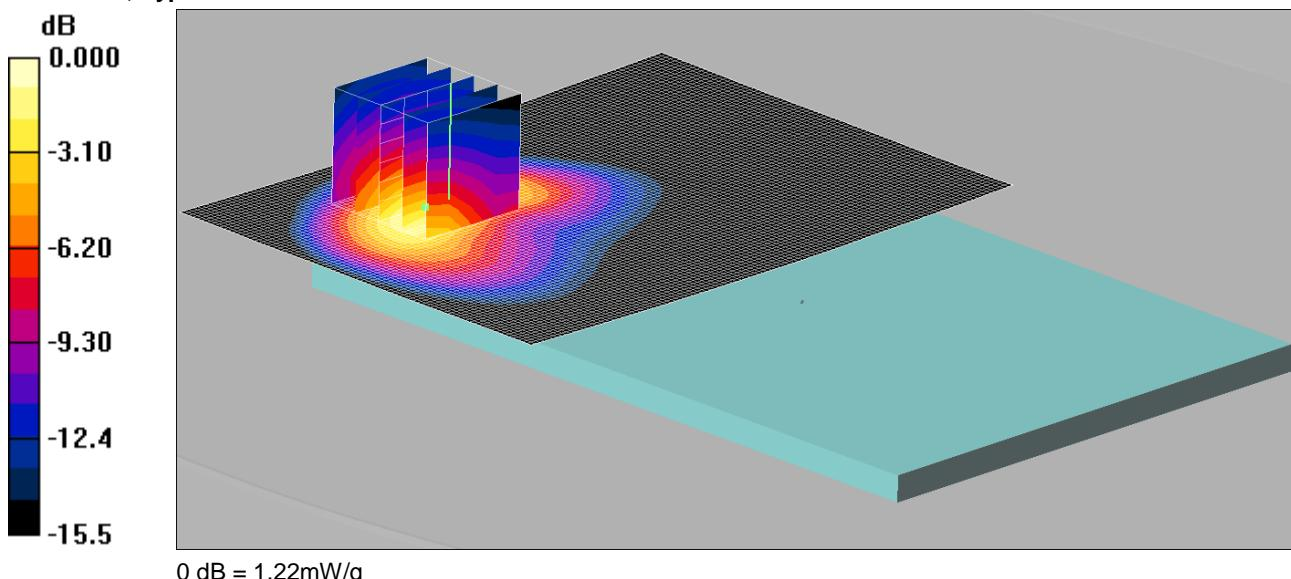
Communication System: LTE Band 5 / 10MHz; Frequency: 829 MHz; Duty Cycle: 1:1
