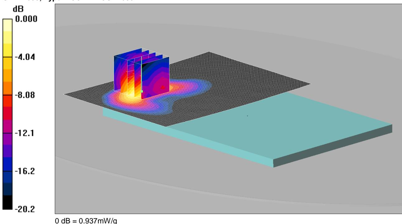
Communication System: CDMA 2000 BC15; Frequency: 1711.25 MHz; Duty Cycle: 1:1
