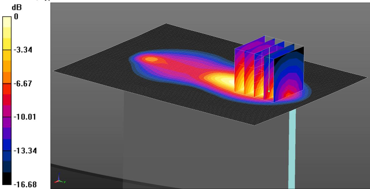
Communication System: UID 0 - n/a, LTE Band 5 / 10MHz; Frequency: 836.5 MHz; Duty Cycle: 1:1
