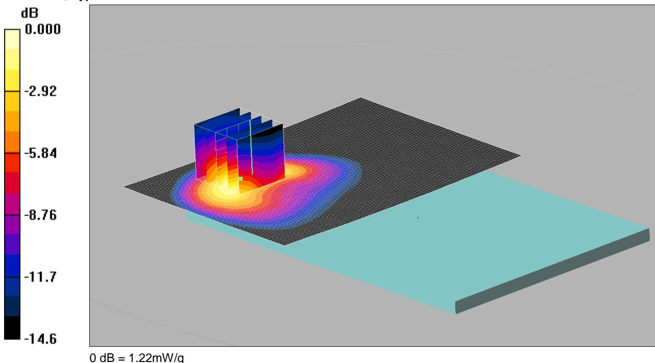
Communication System: CDMA 2000 BC10; Frequency: 817.9 MHz; Duty Cycle: 1:1
