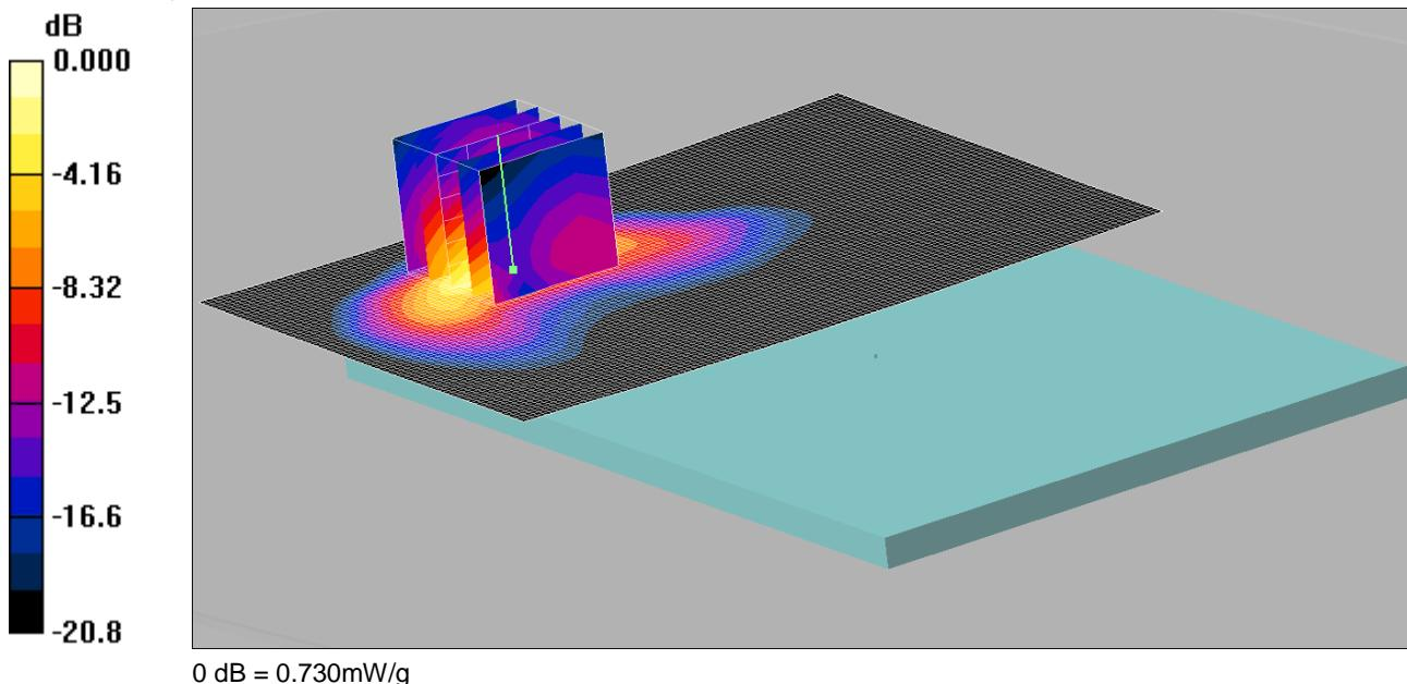
Communication System: LTE - Band 4 / 20MHz Channel; Frequency: 1732.5 MHz; Duty Cycle: 1:1
