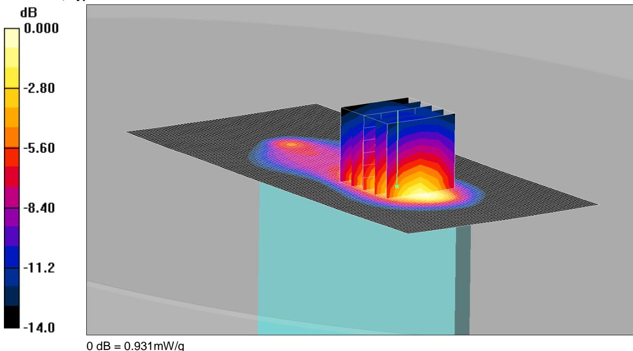
Communication System: LTE Band 5 / 10MHz; Frequency: 836.5 MHz; Duty Cycle: 1:1
