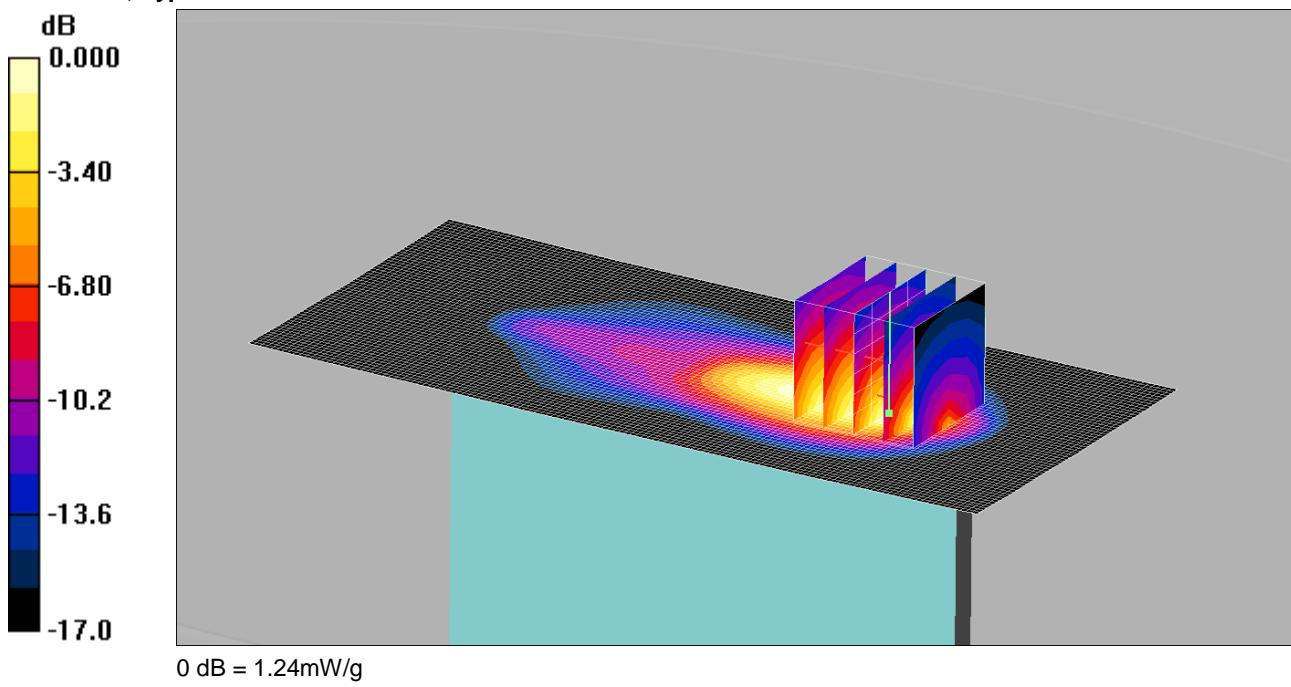
Communication System: CDMA 2000 BC10; Frequency: 817.9 MHz; Duty Cycle: 1:1
