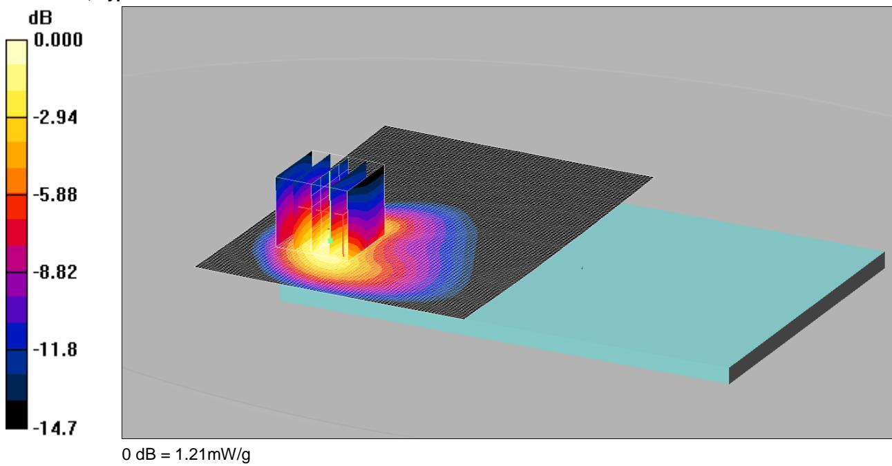
Communication System: CDMA 2000 BC10; Frequency: 823.1 MHz; Duty Cycle: 1:1
