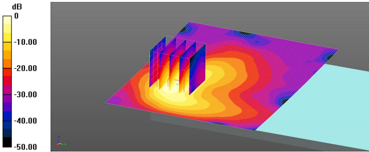
Communication System: UID 0, LTE FDD Bands - 20MHz Channel BW (0); Frequency: 1732.5 MHz; Duty Cycle: 1:1
