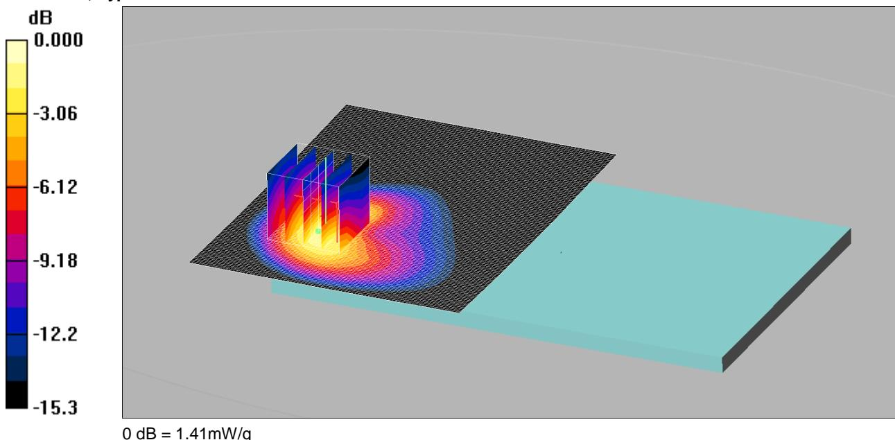
Communication System: CDMA 2000 BC10; Frequency: 820.5 MHz; Duty Cycle: 1:1
