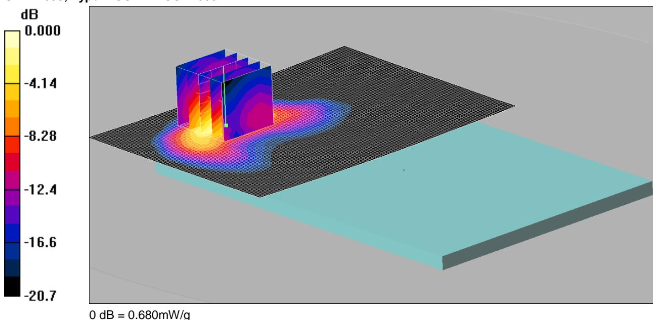
Communication System: LTE - Band 4 / 20MHz Channel; Frequency: 1745 MHz; Duty Cycle: 1:1
