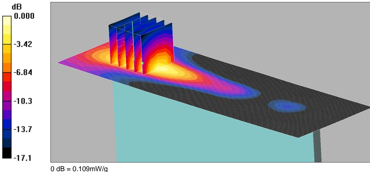
Communication System: LTE - Band 4 / 20MHz Channel; Frequency: 1720 MHz; Duty Cycle: 1:1
