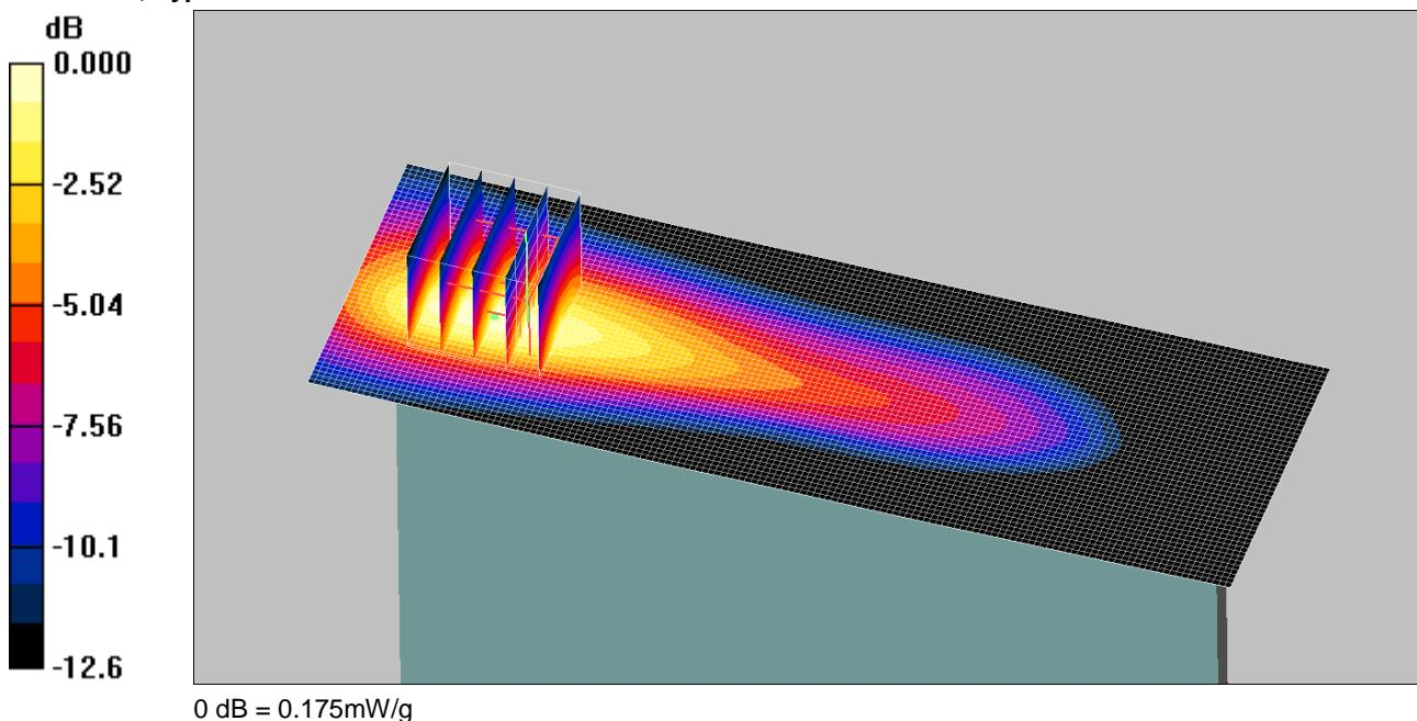
Communication System: CDMA 2000 BC10; Frequency: 823.1 MHz; Duty Cycle: 1:1
