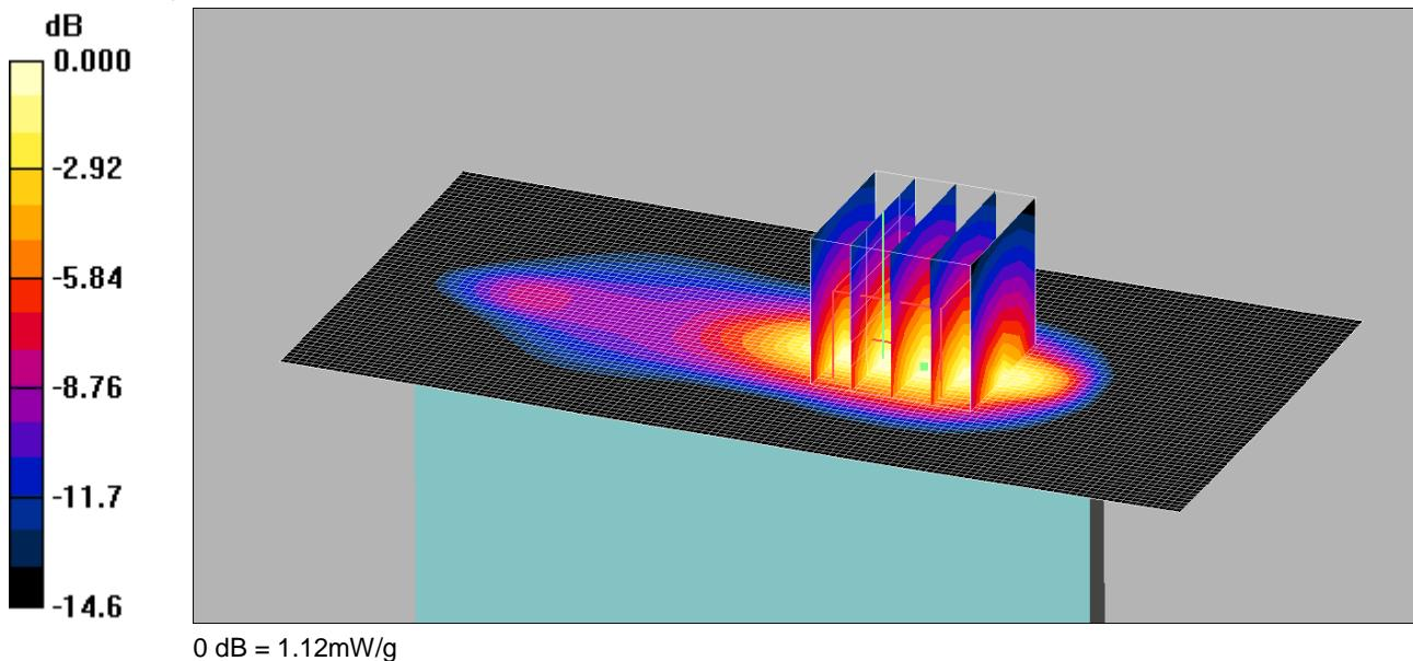
Communication System: CDMA 2000 BC10; Frequency: 823.1 MHz; Duty Cycle: 1:1
