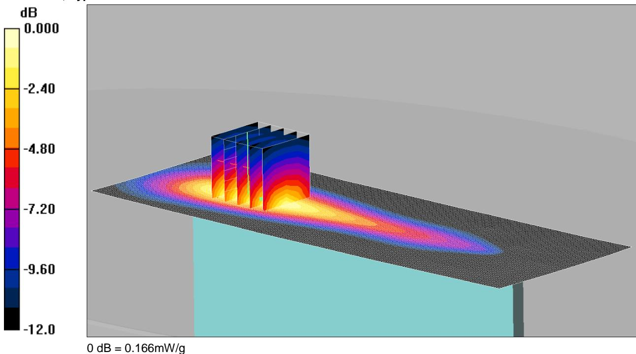
Communication System: CDMA 2000 BC10; Frequency: 820.5 MHz; Duty Cycle: 1:1
