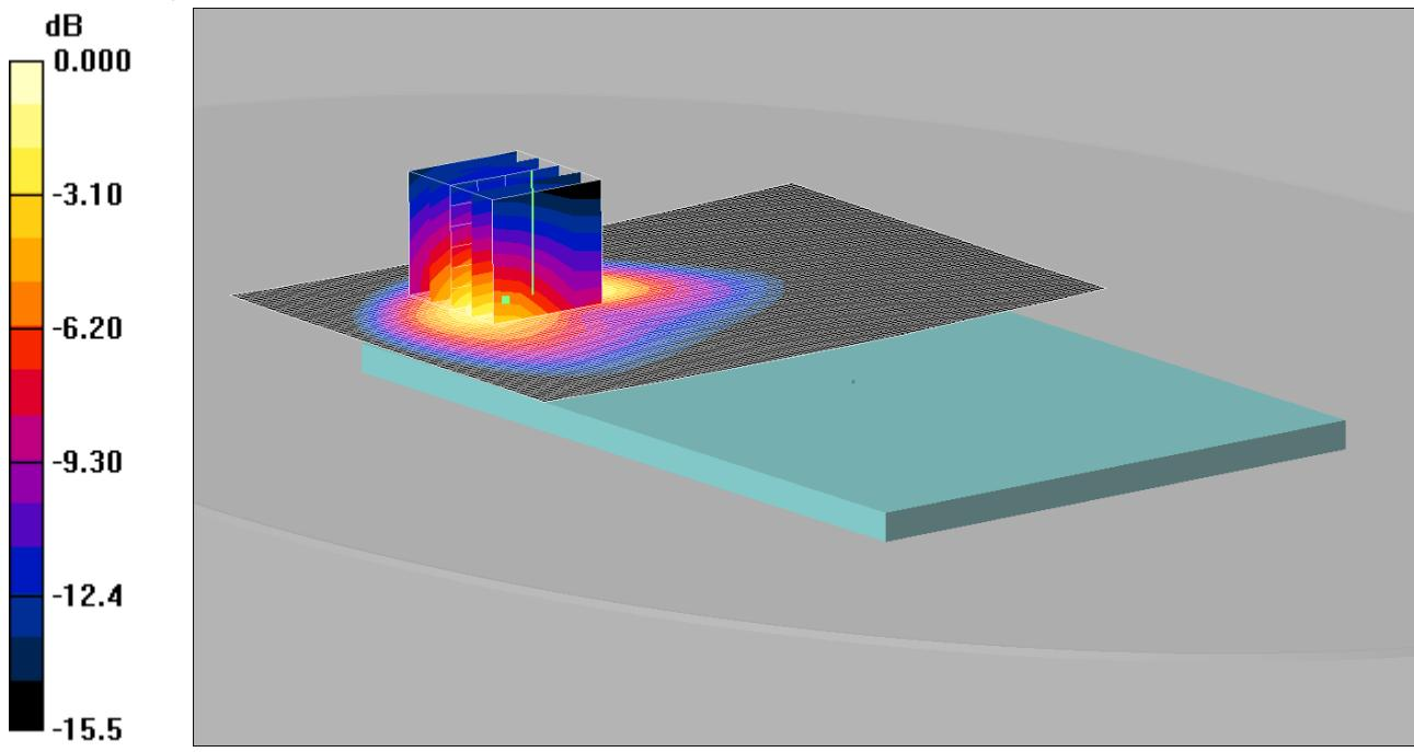
Communication System: LTE Band 5 / 10MHz; Frequency: 836.5 MHz; Duty Cycle: 1:1
