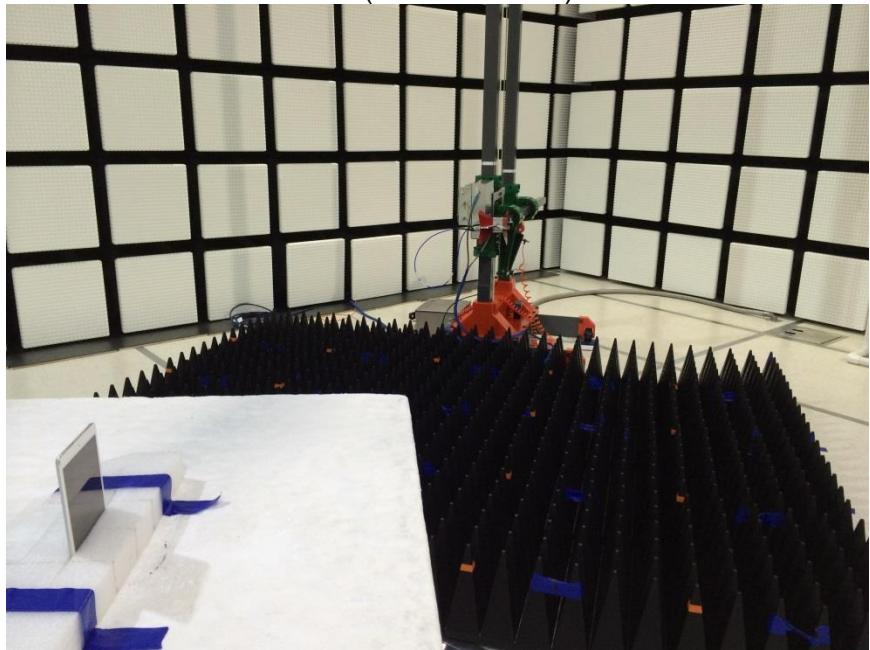
**RADIATED RF MEASUREMENT SETUP**
