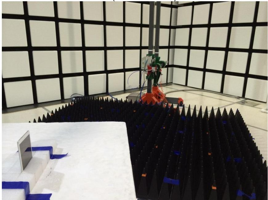
**RADIATED RF MEASUREMENT SETUP**
