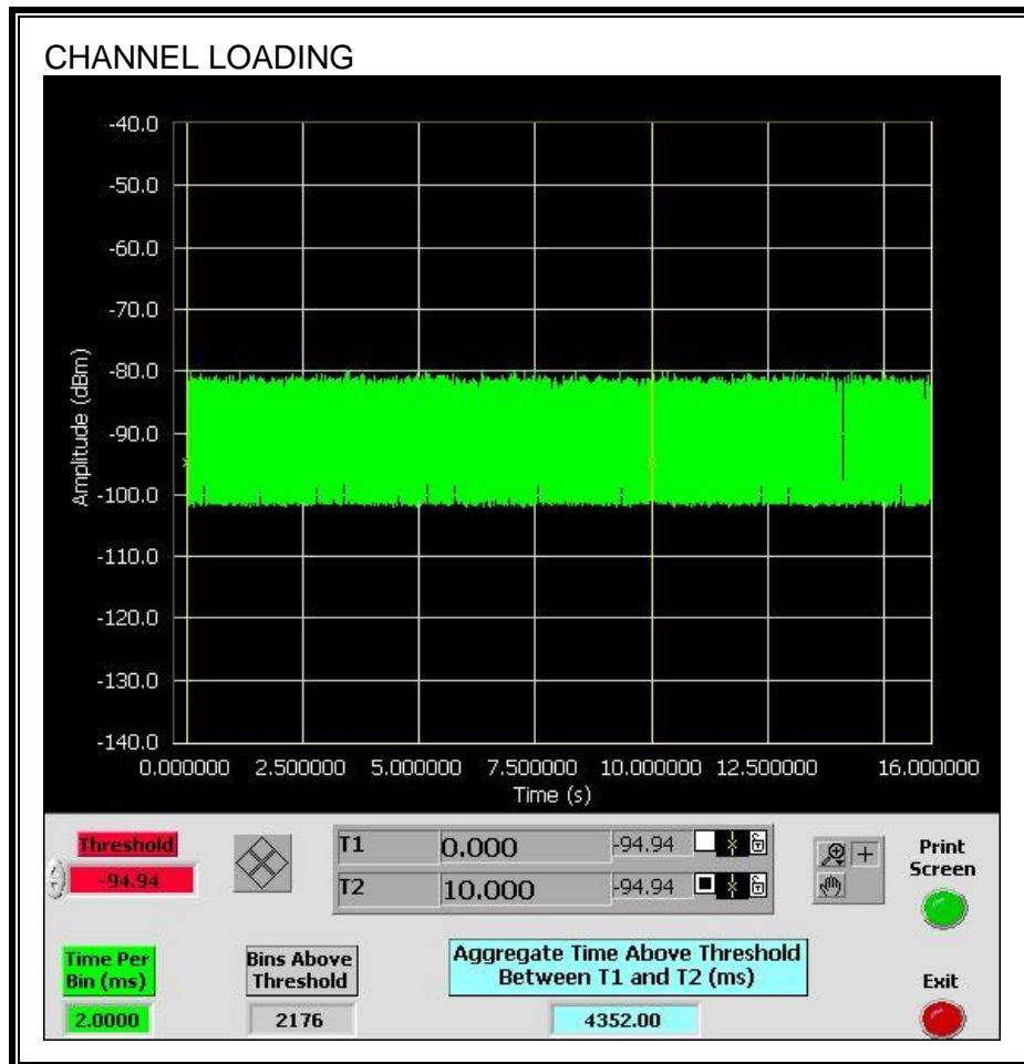
The level of traffic loading on the channel by the EUT is 43.52%
