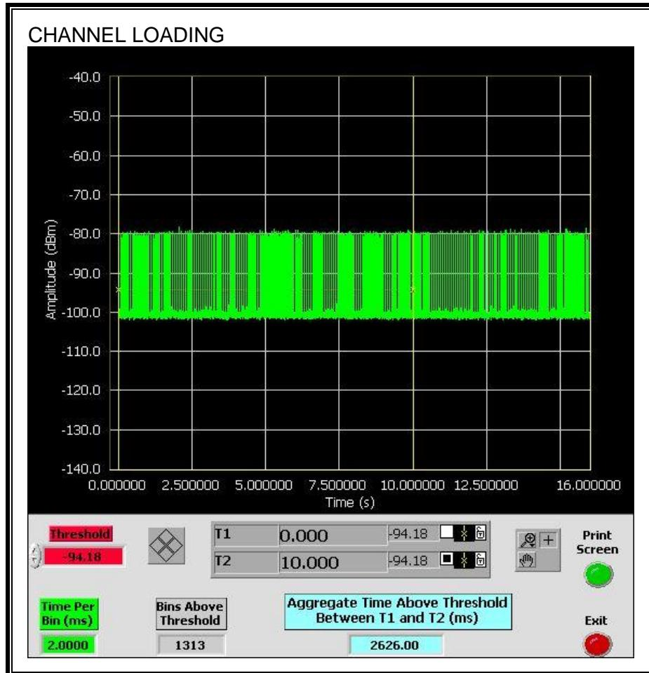
The level of traffic loading on the channel by the EUT is 26.26%
