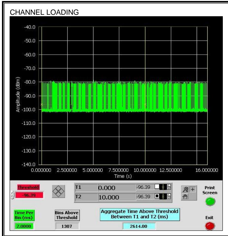
The level of traffic loading on the channel by the EUT is 26.14%
