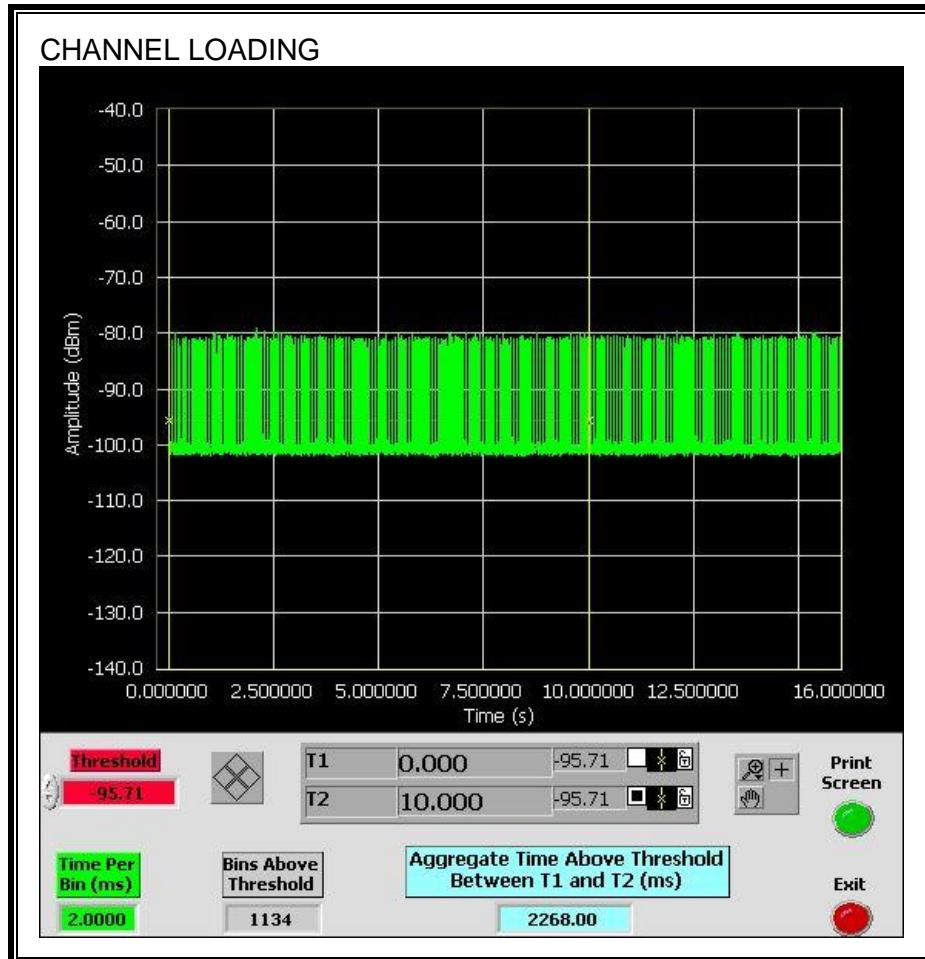
The level of traffic loading on the channel by the EUT is 22.68%
