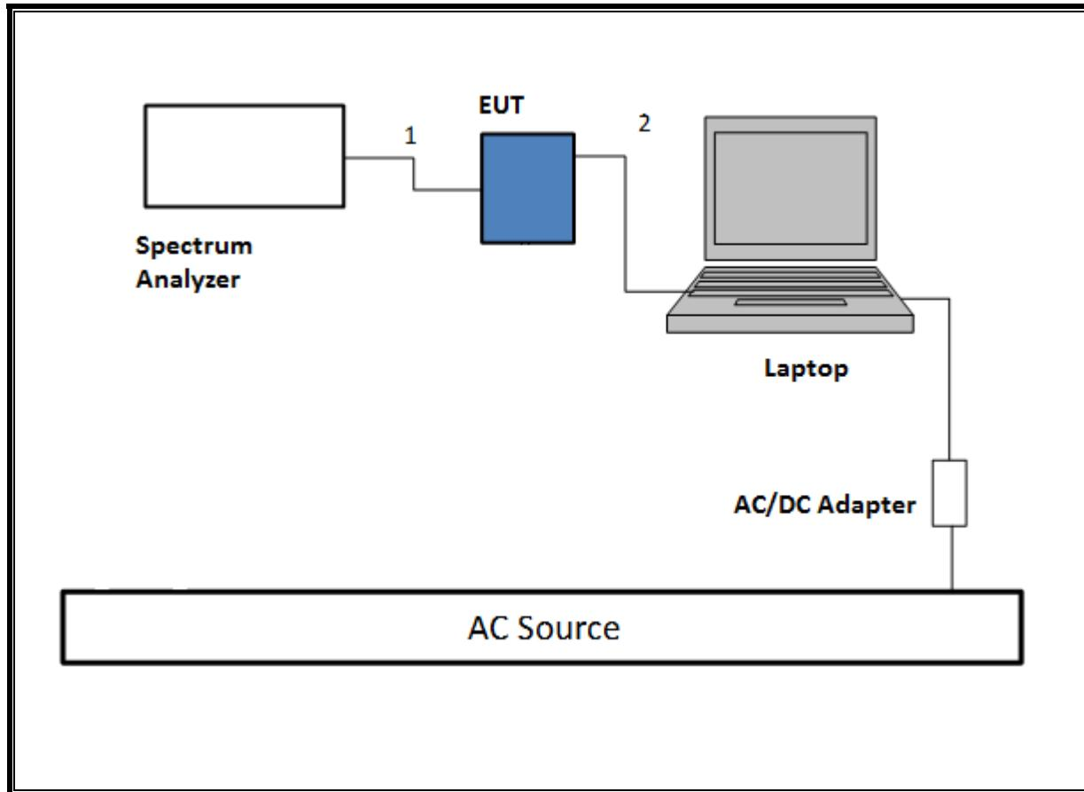
**TEST SETUP- RADIATED-ABOVE 1 GHZ**
