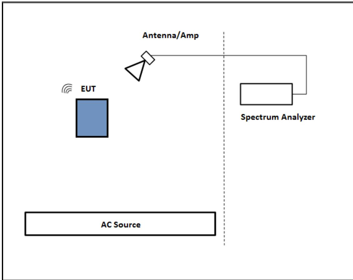
**TEST SETUP- BELOW 1GHZ & AC LINE CONDUCTED TESTS**
