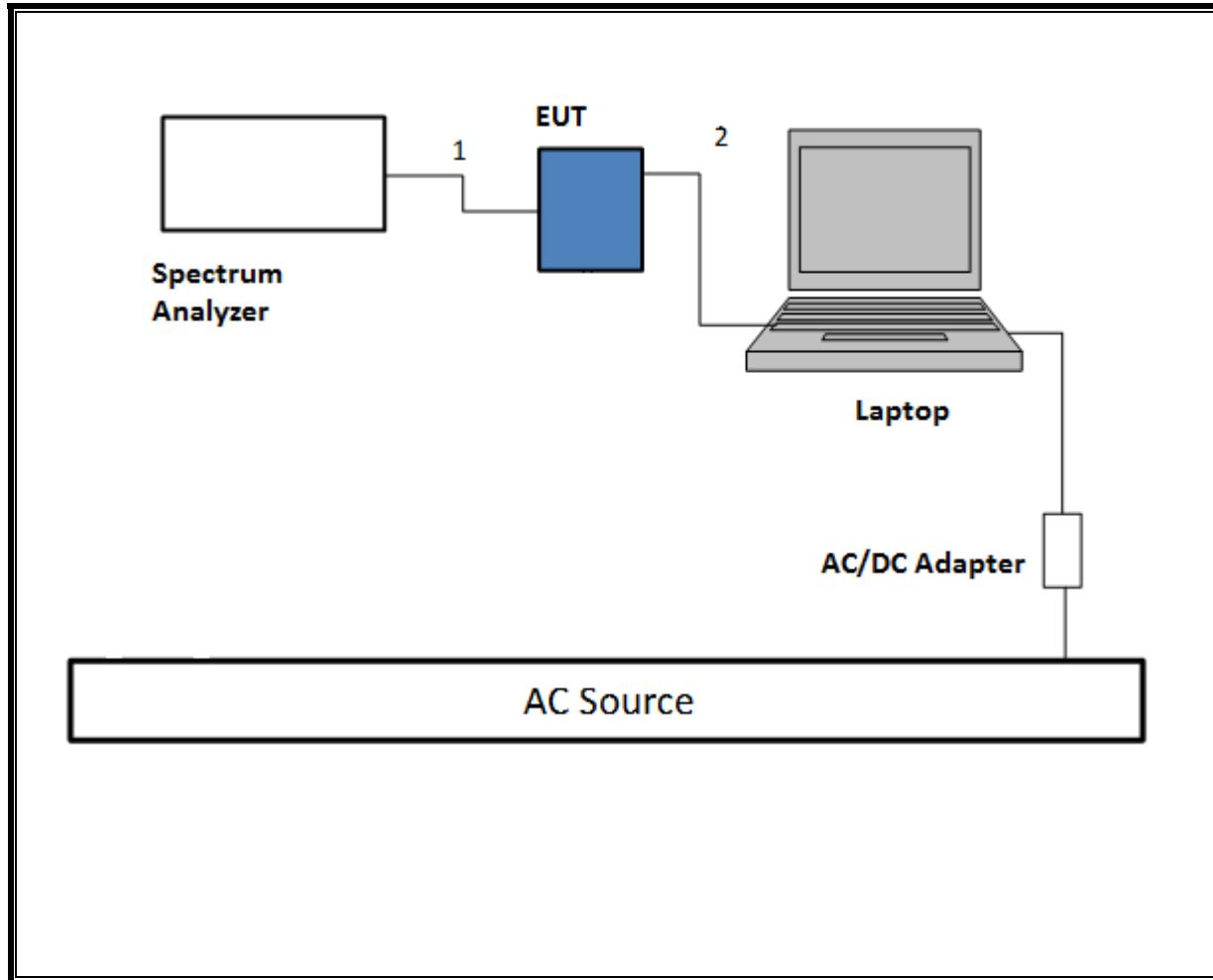
**TEST SETUP- RADIATED-ABOVE 1 GHZ**
