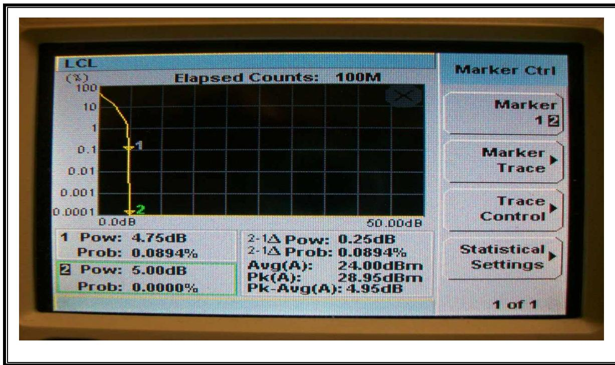
LTE 16QAM Band 2 (10.0 MHz BAND WIDTH)
