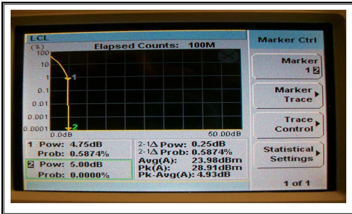
LTE 16QAM Band 2 (5.0 MHz BAND WIDTH)
