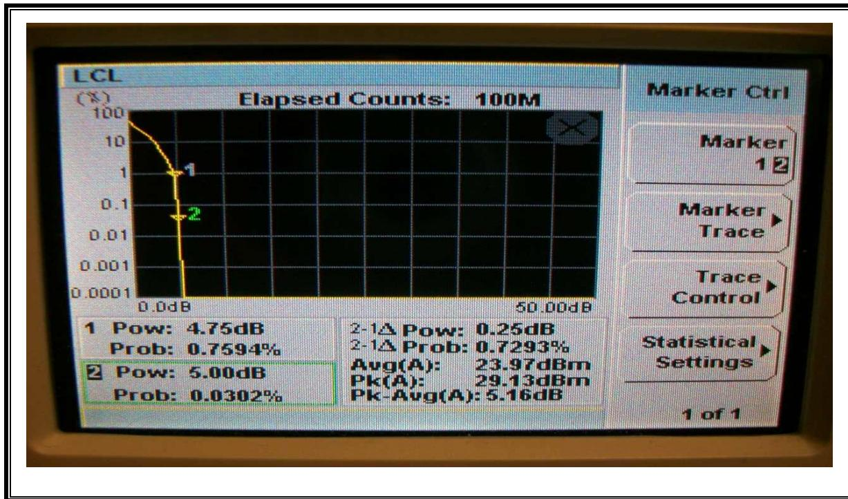
**16QAM Band 2 (1.4 MHz BAND WIDTH)**
