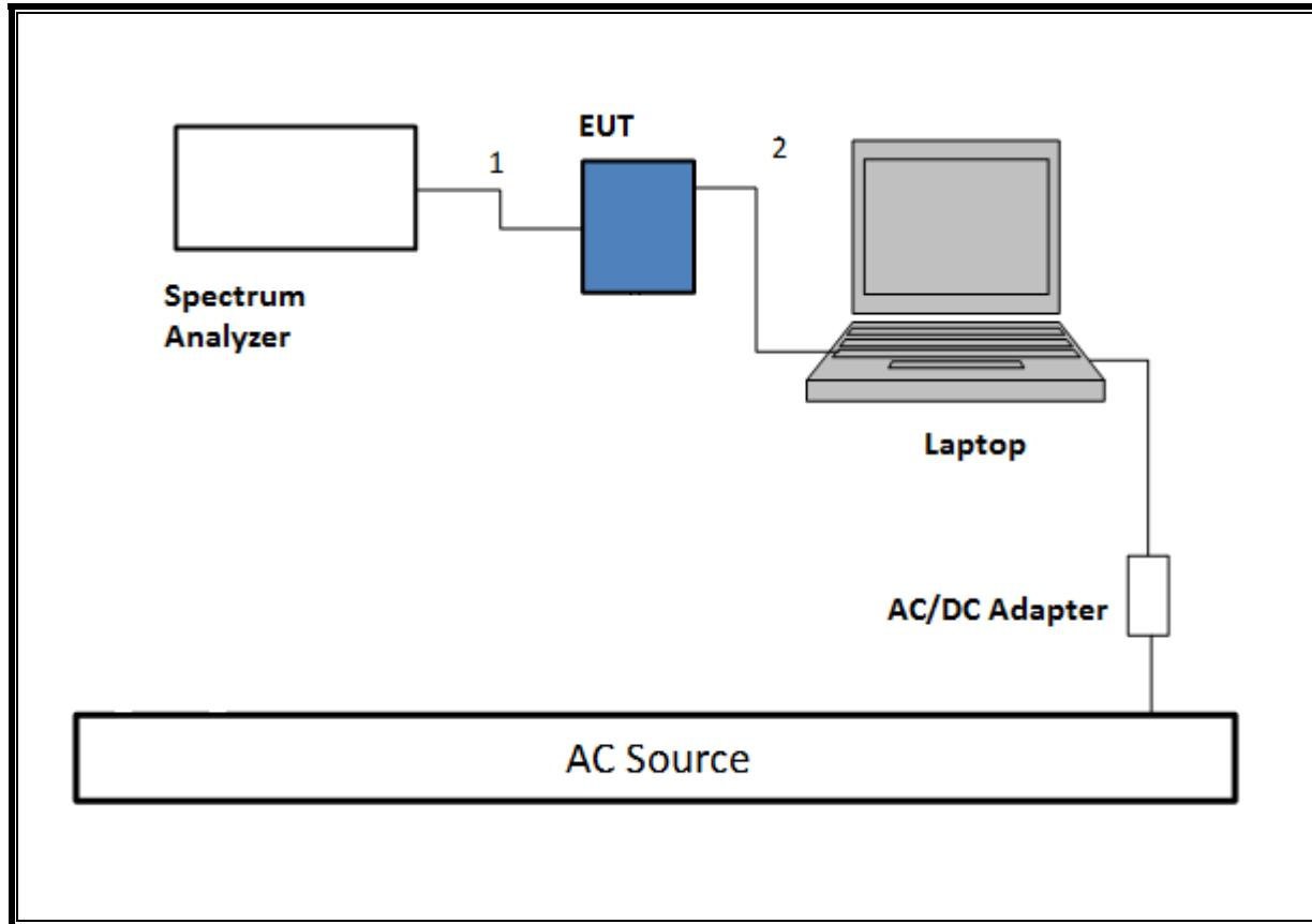
**TEST SETUP- RADIATED-ABOVE 1 GHZ**
