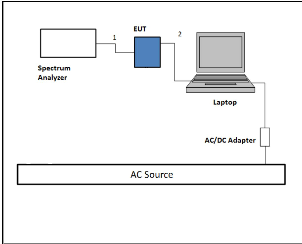
**TEST SETUP- RADIATED-ABOVE 1 GHZ**
