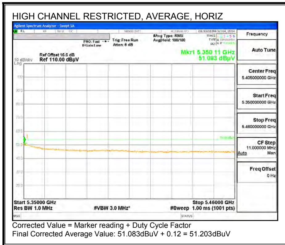
Corrected Value = Marker reading + Duty Cycle Factor
