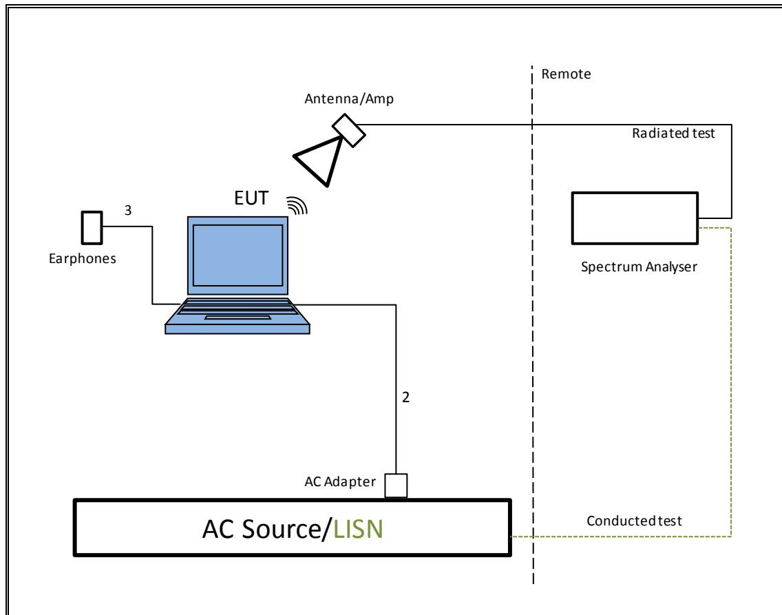
**TEST SETUP- RADIATED ABOVE 1 GHz**
