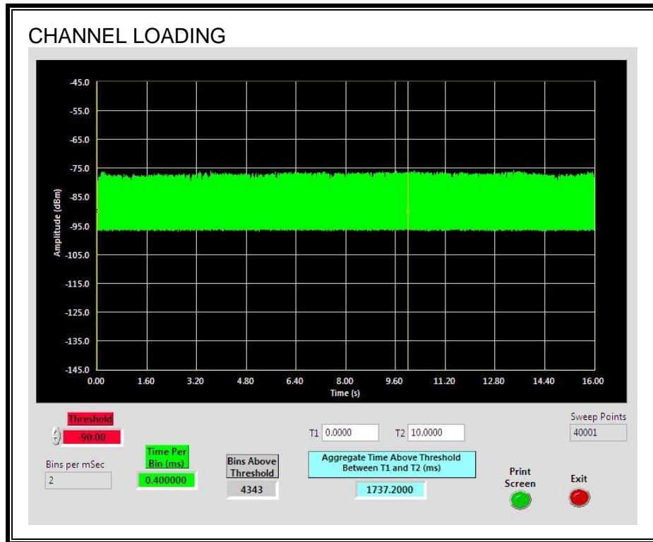
The level of traffic loading on the channel by the EUT is 17.37%
