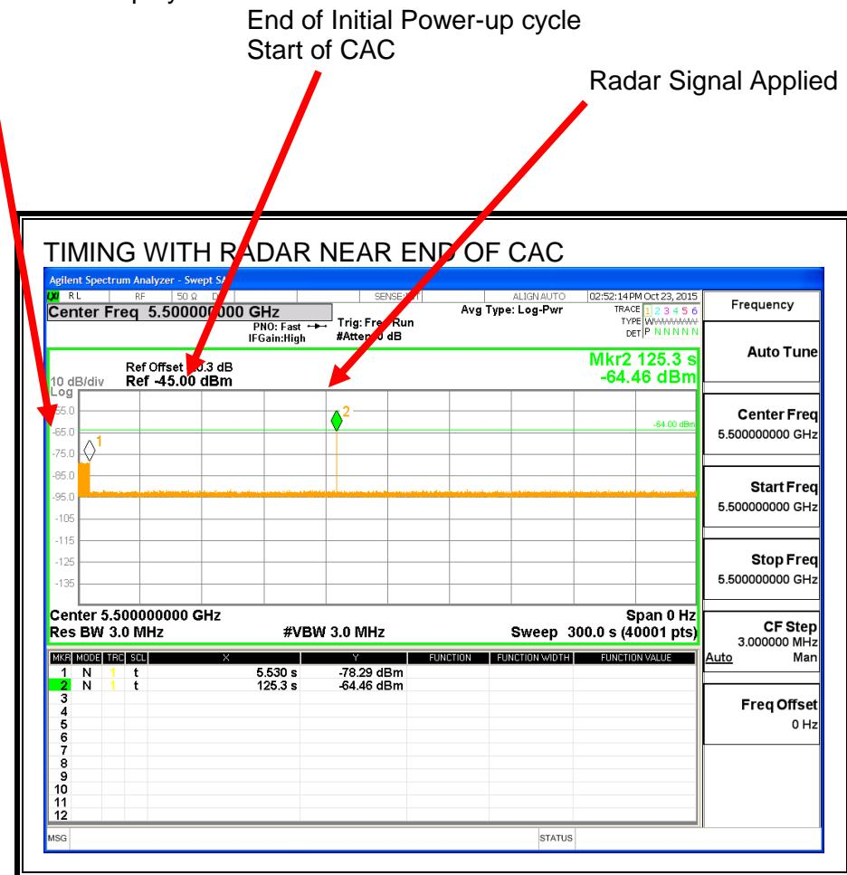
No EUT transmissions were observed after the radar signal.
