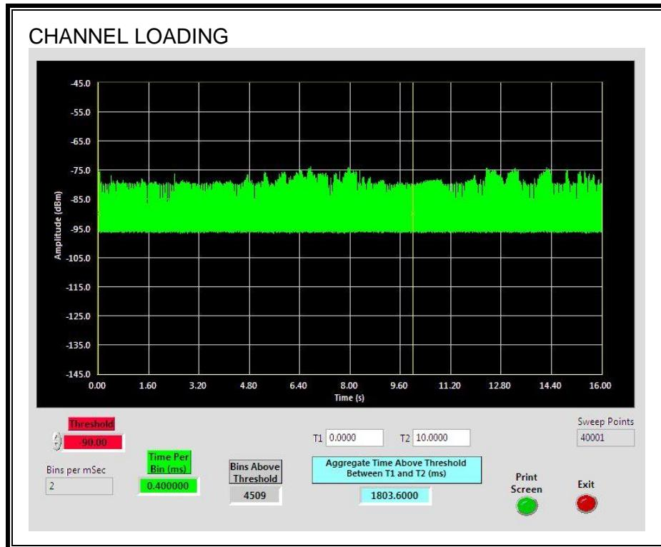
The level of traffic loading on the channel by the EUT is 18.03%
