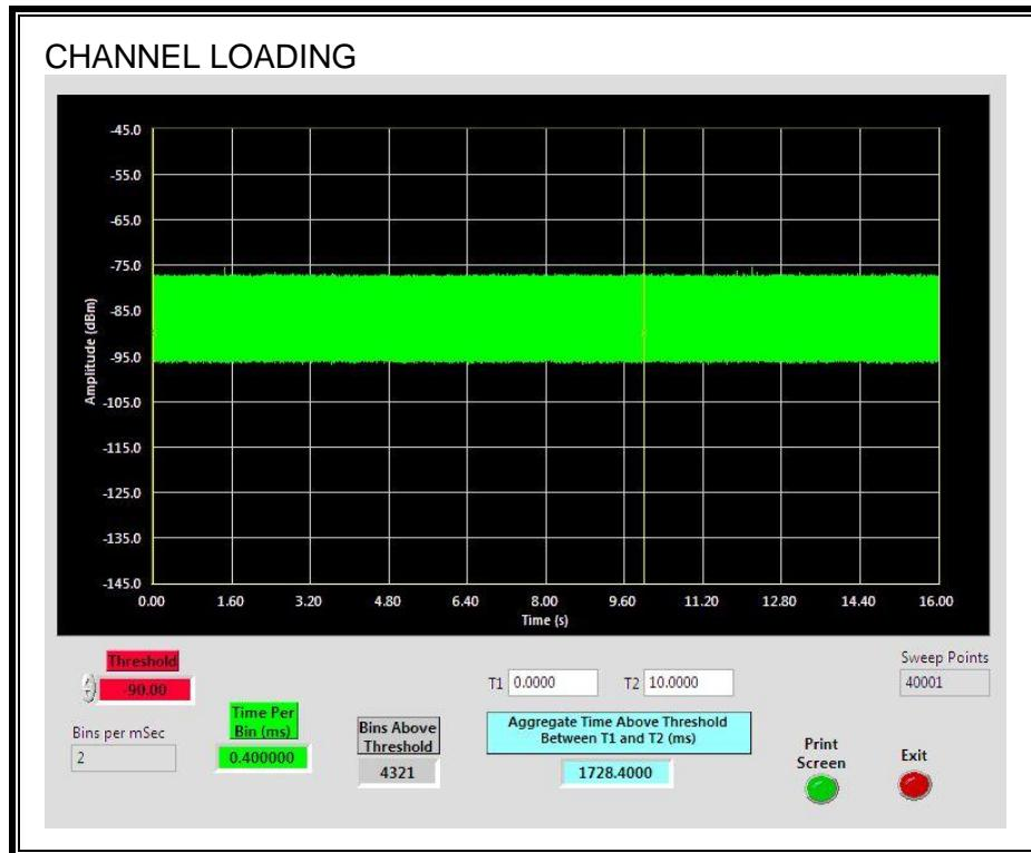
The level of traffic loading on the channel by the EUT is 17.28%
