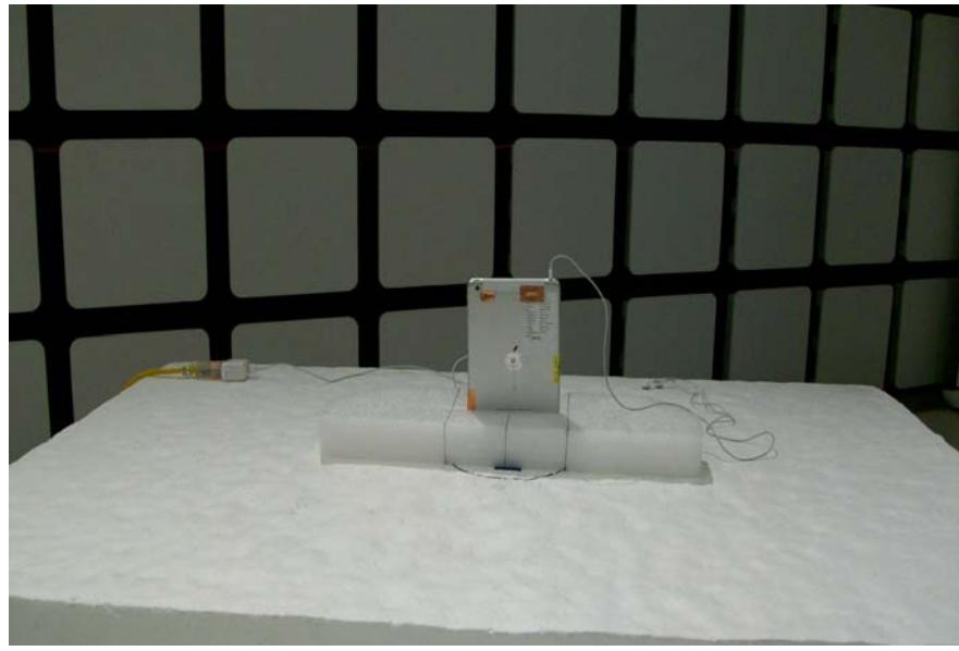
**RADIATED RF MEASUREMENT SETUP**
